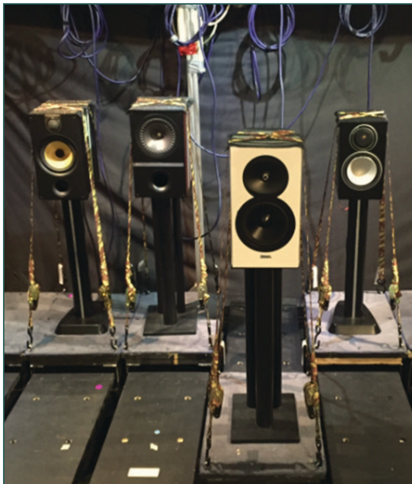
Photo 1: The Speaker Shuffler moves each speaker into the listening location so quickly that the listener can maintain the memory of the last speaker.
