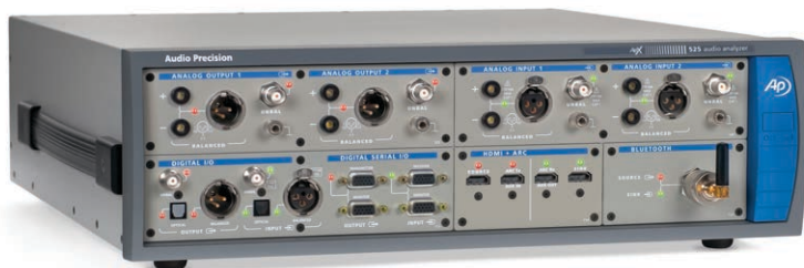
Photo 4: Audio Precision's APx525 analyzers provide typical THD+N at -108 dB (-110 dB with the AG52 option) offering high-quality analog performance.
