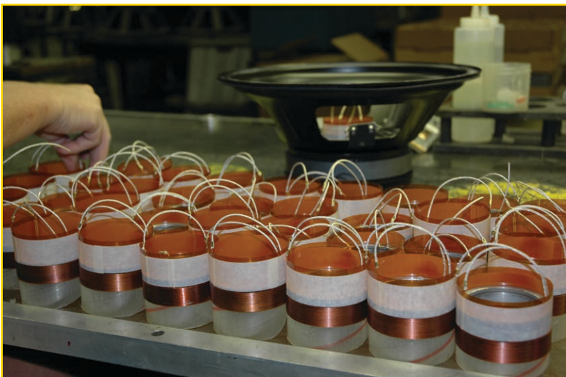
Voice coils are inserted into the loudspeaker during the final assembly process. (Photo courtesy of Eminence)
