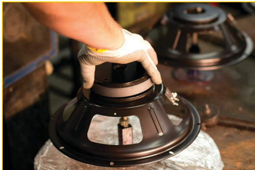
A magnet and a back plate are glued to the top plate and basket assembly. (Photo courtesy of Eminence)
