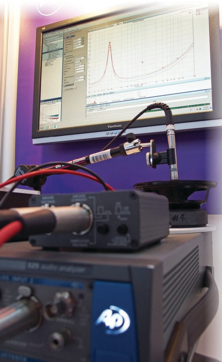
Photo 1: Audio Precision's APx525 is a two-channel audio analyzer for R&D engineers and production technicians who want fast and easy audio testing capabilities.
