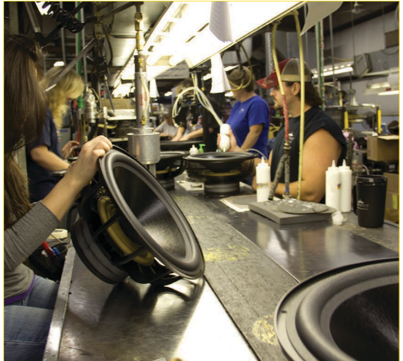
Speakers in the final assembly area move down a conveyer system where technicians apply the edge treatment and attach the leads to the terminals. (Photo courtesy of Eminence)
