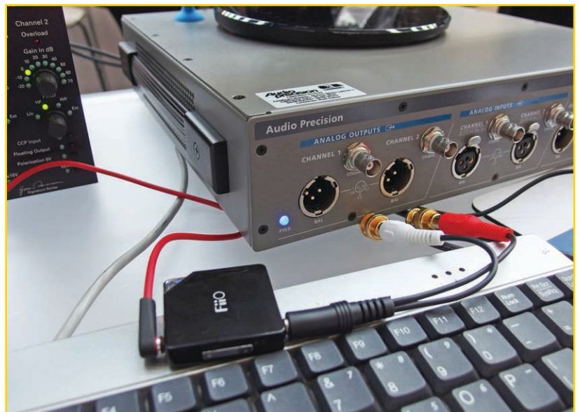
Photo 2: Audio Precision’s APx515 is a high-performance audio analyzer optimized for production tests. The APx515 has a typical THD+N of -106 dB, a one million point fast Fourier transform (FFT) with 24-bit resolution, and 192-kHz digital I/O.
