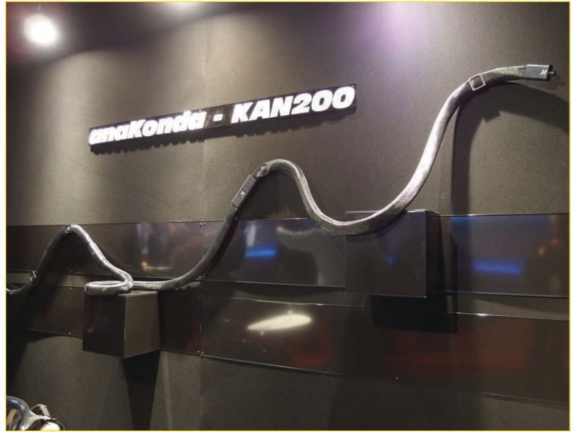
K-array's Anakonda KAN200 is the first bendable loudspeaker. It can be wrapped around poles or mounted to uneven surfaces. Each element is 2 m (6.6') in length, and can be daisy-chained to form one seamless sound line. ( www.k-array.com )
