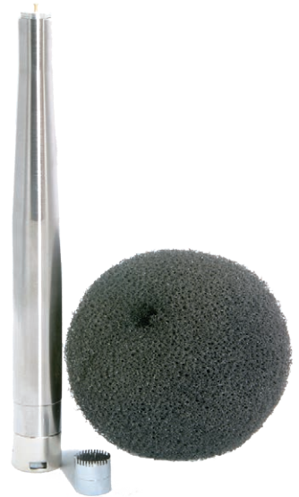
7052PH PHANTOM POWERED MEASUREMENT MIC IEC61094 Compliant <4Hz to >25kHz <18 dBA Operational Temp <-20°C to >70°C Storage Temp <-30°C to >85°C
