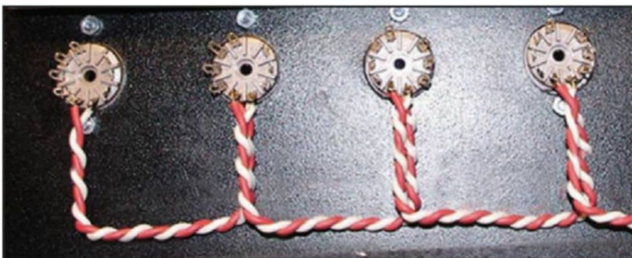
Photo 1: Twisting filament leads together and routing them close to the chassis can reduce hum.
