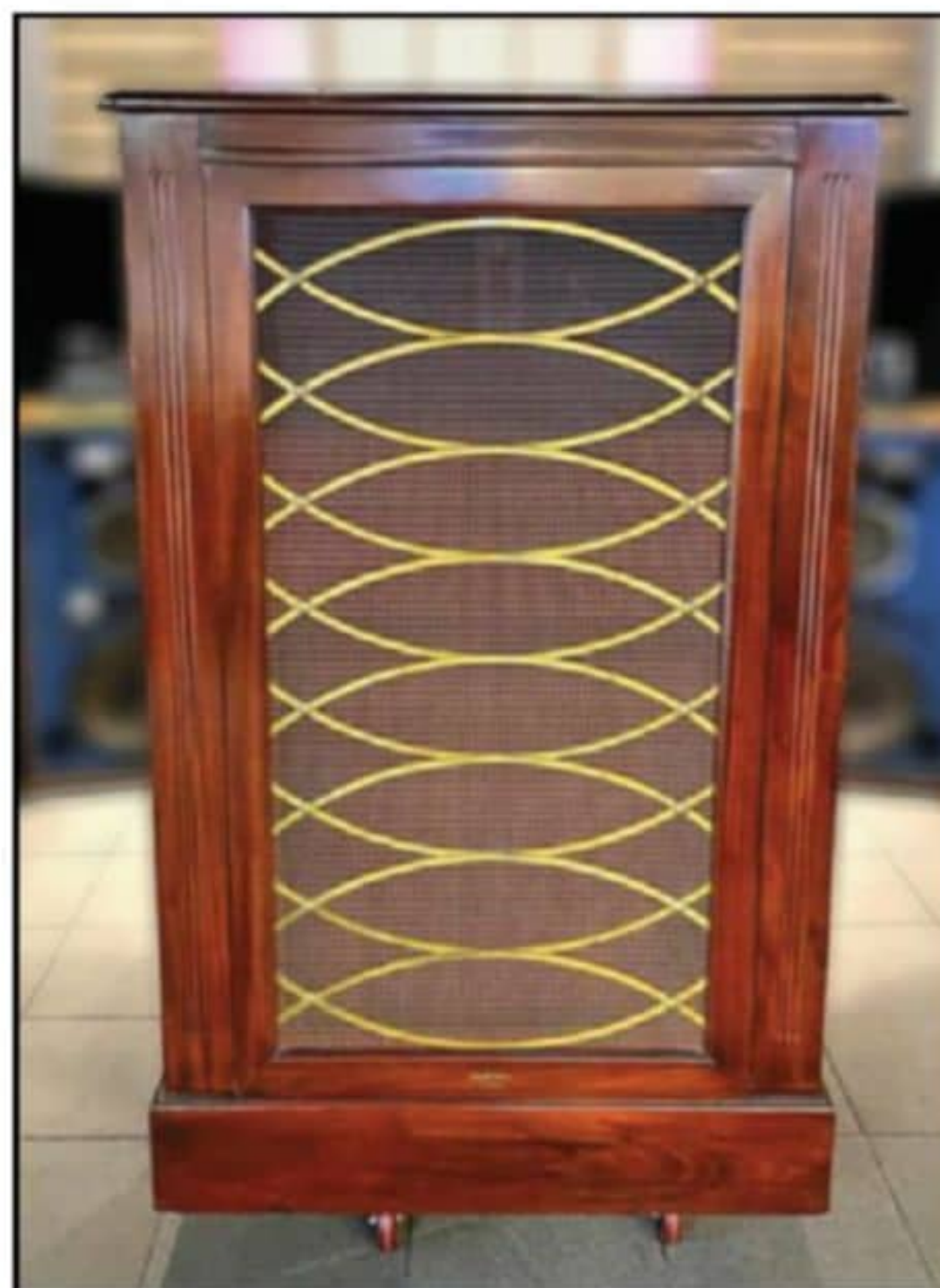
Photo 12: The Electro Voice Patrician boasted 15Hz to 23,000Hz frequency response.
