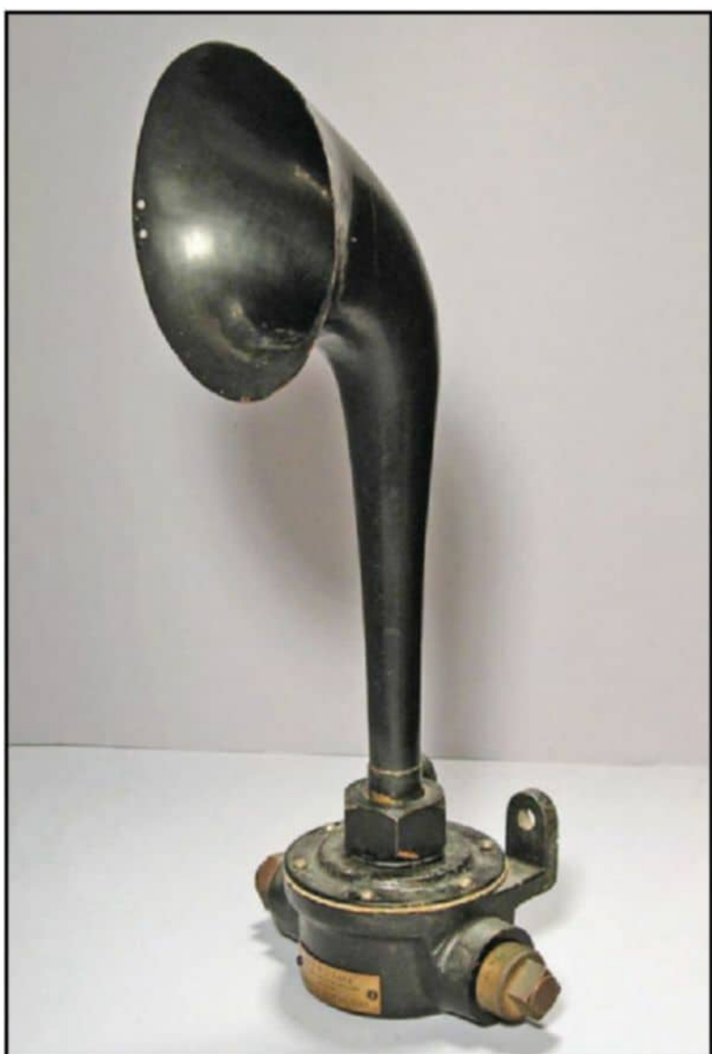
Photo 4: The WE CW-929 "loudspeaking telephone" used a design similar to Jensen's.
