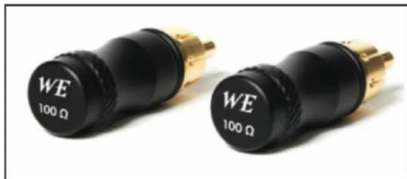
Photo 4: Phono termination plugs can optimize the load impedance presented to the cartridge.
