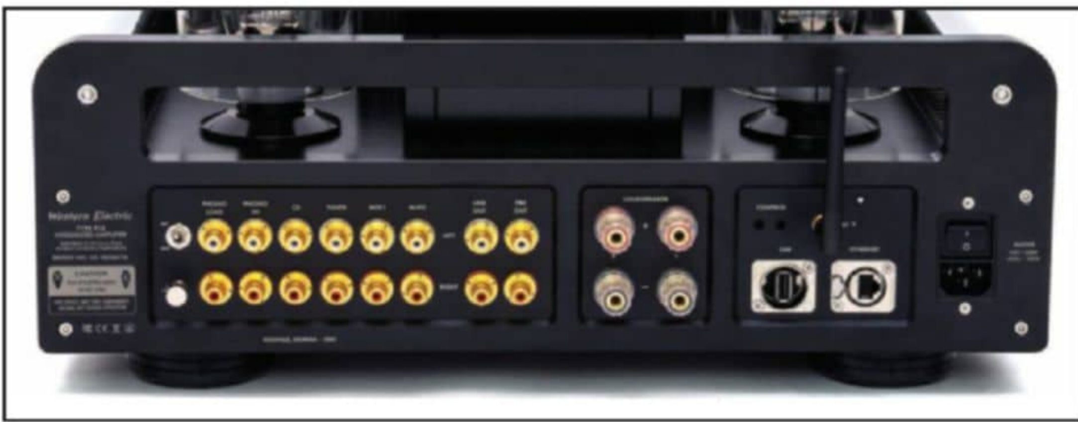
Photo 3: The MC/MM switch and phono load jacks can be seen at the left of the 91E's back panel.
