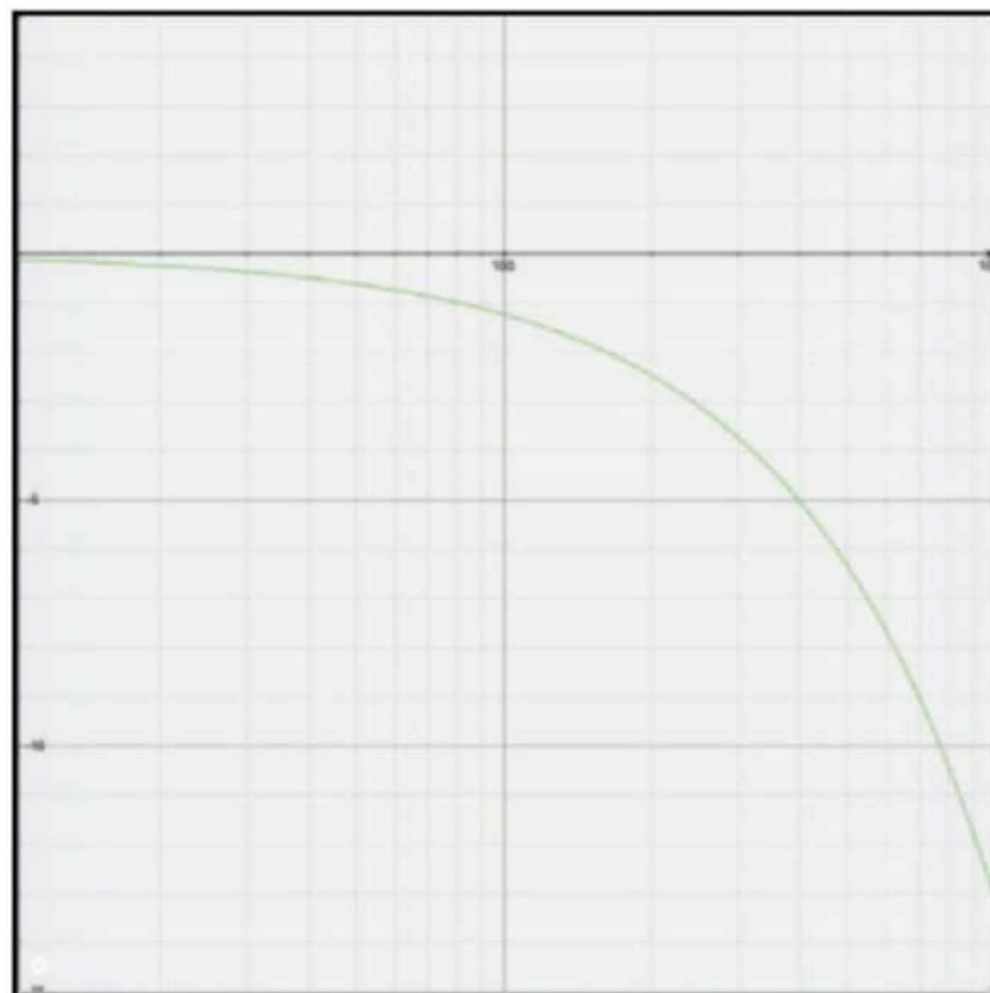
Figure 3c: This graph shows the resulting frequency response. It is accurate within +0 to -0.1dB up to 1000Hz.
