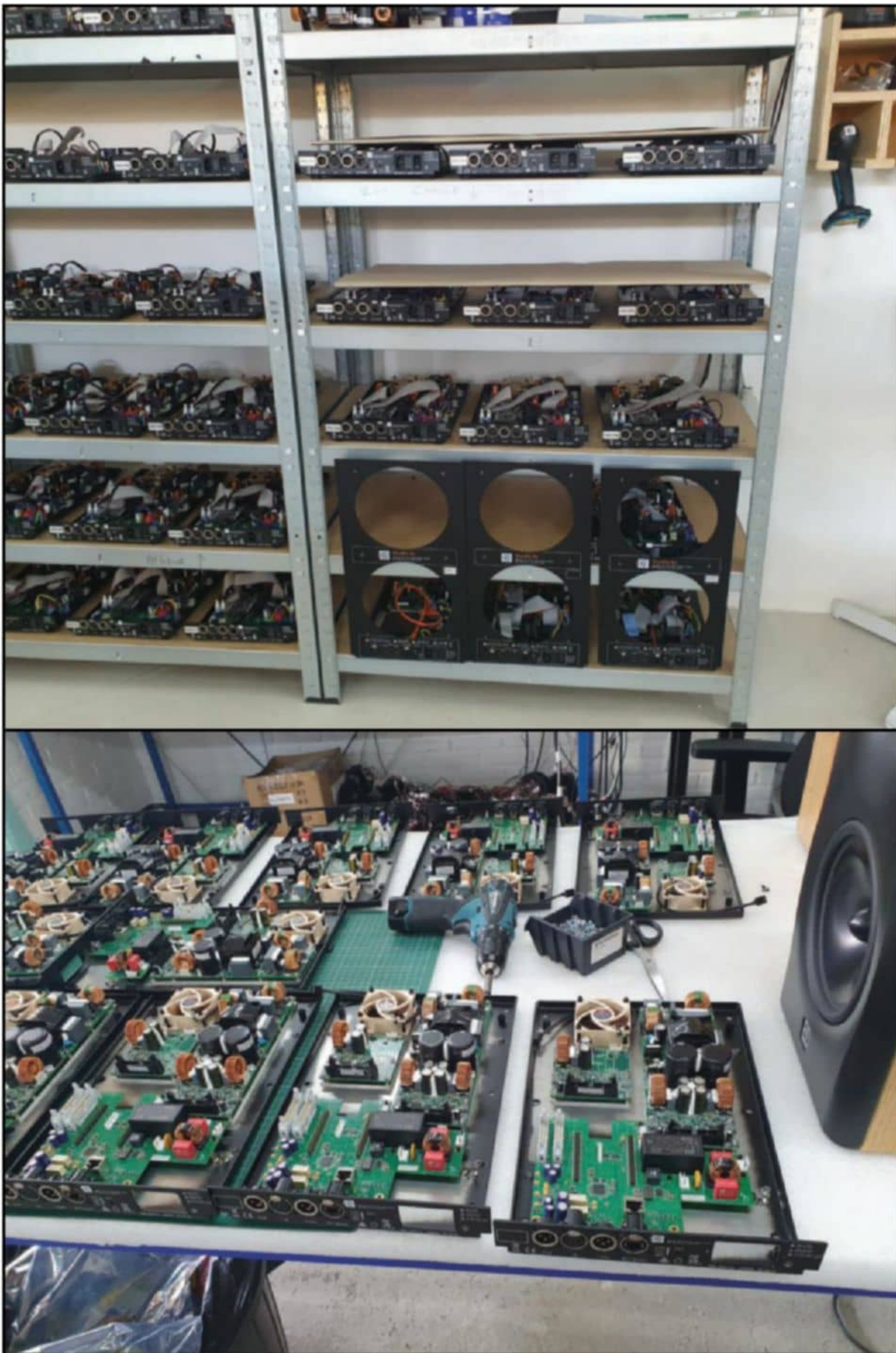
All Dutch & Dutch speakers are assembled and fully tested in-house. Here we see the electronics modules being assembled and units ready to be incorporated in the speaker cabinets, which are mostly assembled to order.
