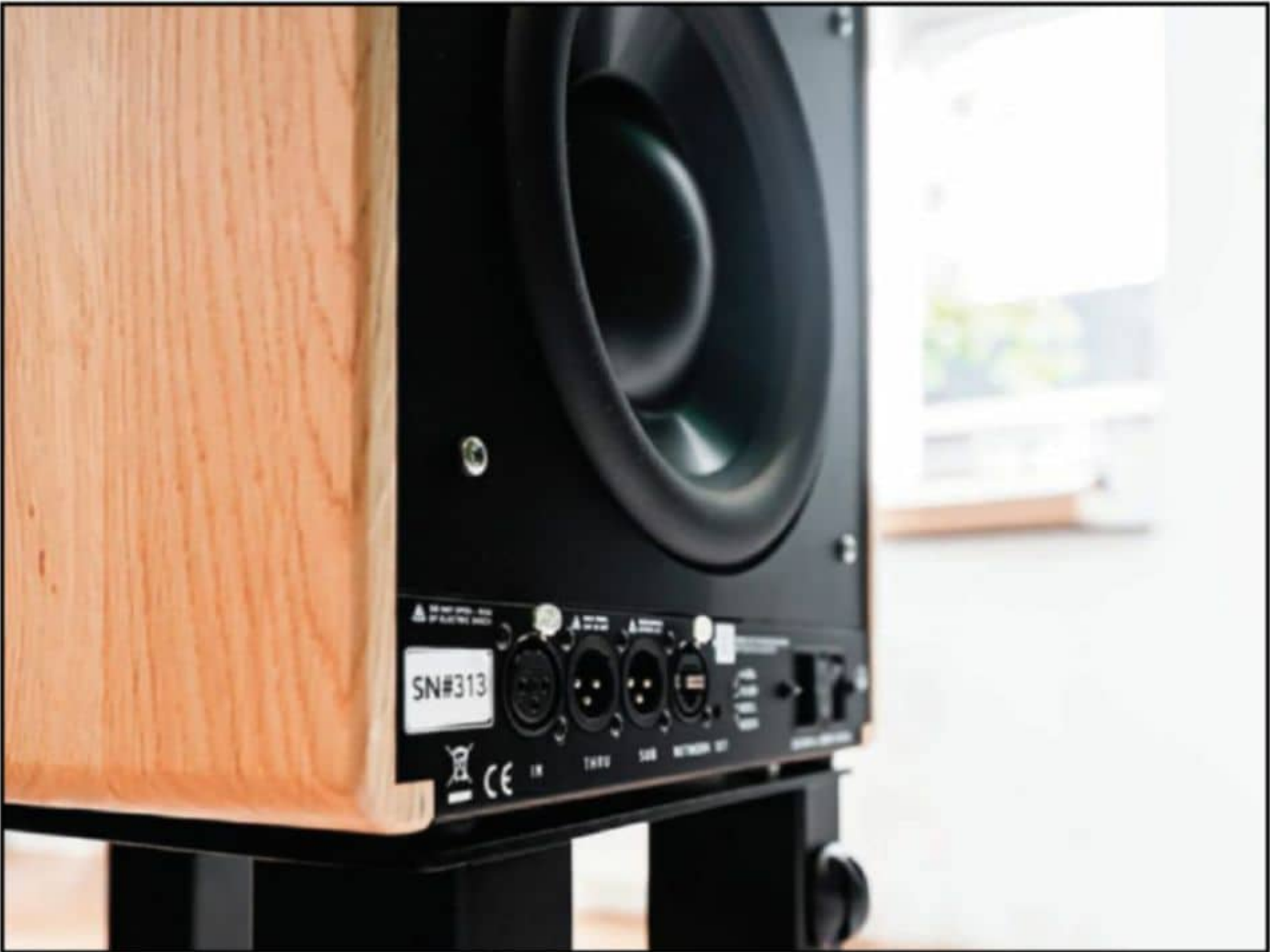
The connectivity in the 8c was also carefully planned, including the use of balanced analog, digital AES3 inputs, plus Ethernet LAN, allowing users to create groups of speakers in zones or multichannel configurations (e.g., Dolby Atmos). AES3 inputs allow balanced Type 1 connections or SPDIF with PCM up to 24-bit/192kHz.
