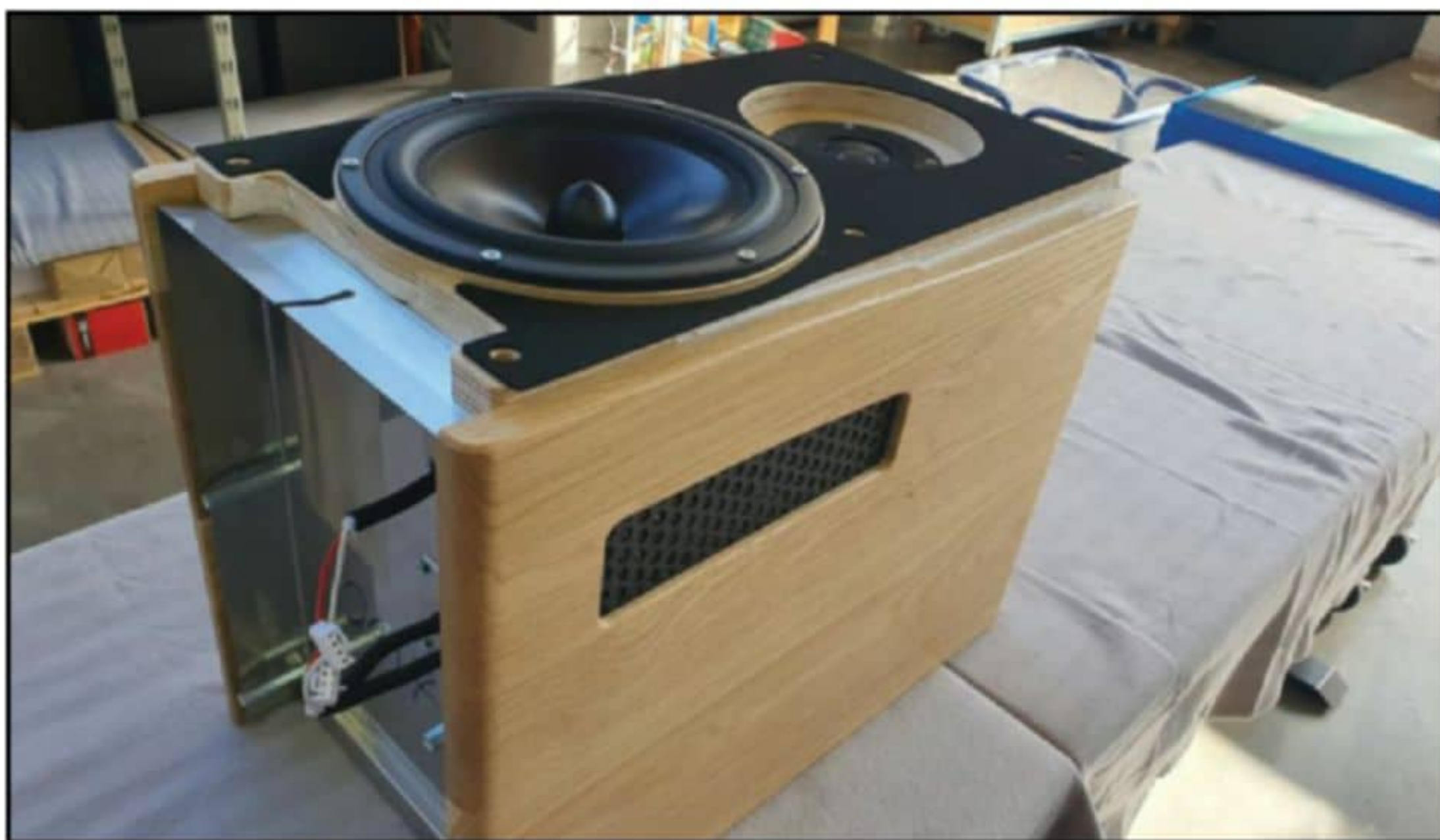
An 8c speaker in the assembly with all drivers in place (1" SEAS aluminum/magnesium alloy dome tweeters, 8" SEAS midranges, and 2x8" woofers), and now ready to receive the electronics and I/O module, and lastly the front baffle
