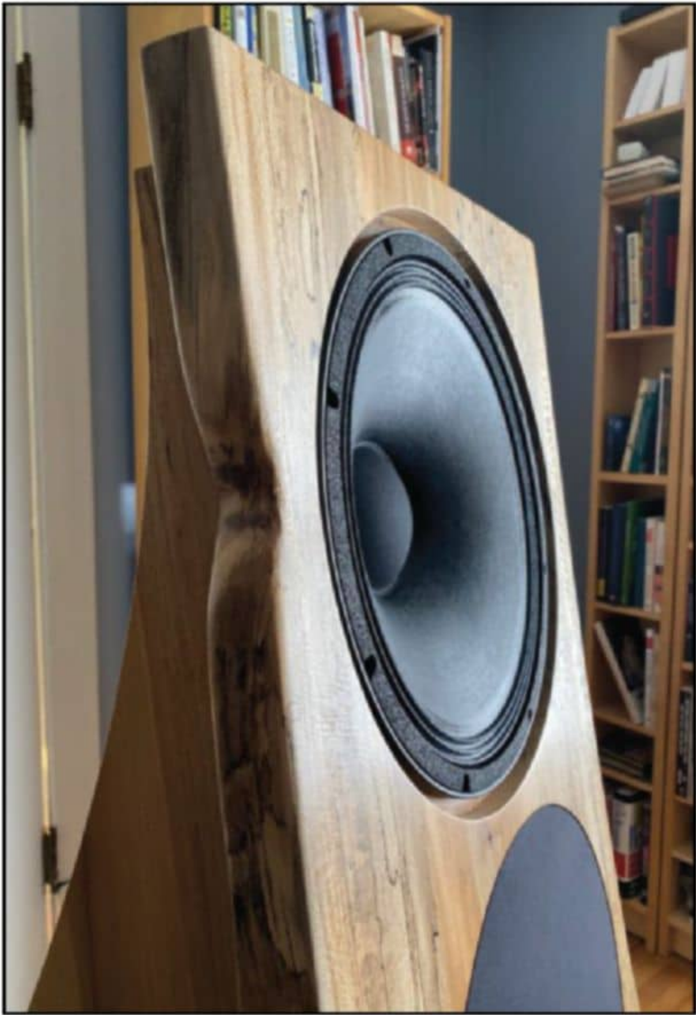
Photo 4: The upper driver is the coaxial B&C Speakers 15CN88, and the SB Audience 150B350 woofers below have 11mm Xmax.
