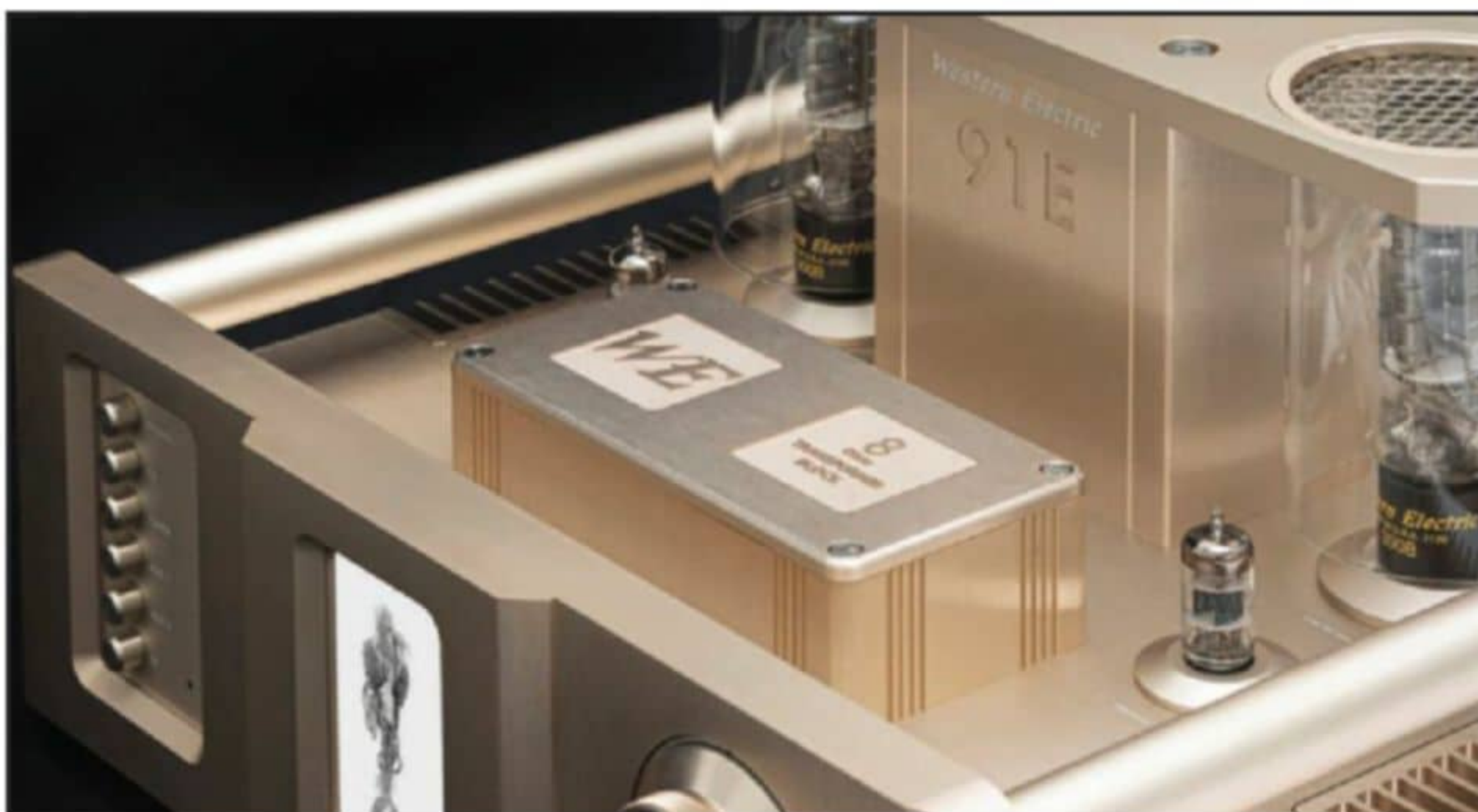
Photo 2: User-pluggable output transformers optimally accommodate different speaker impedances.
