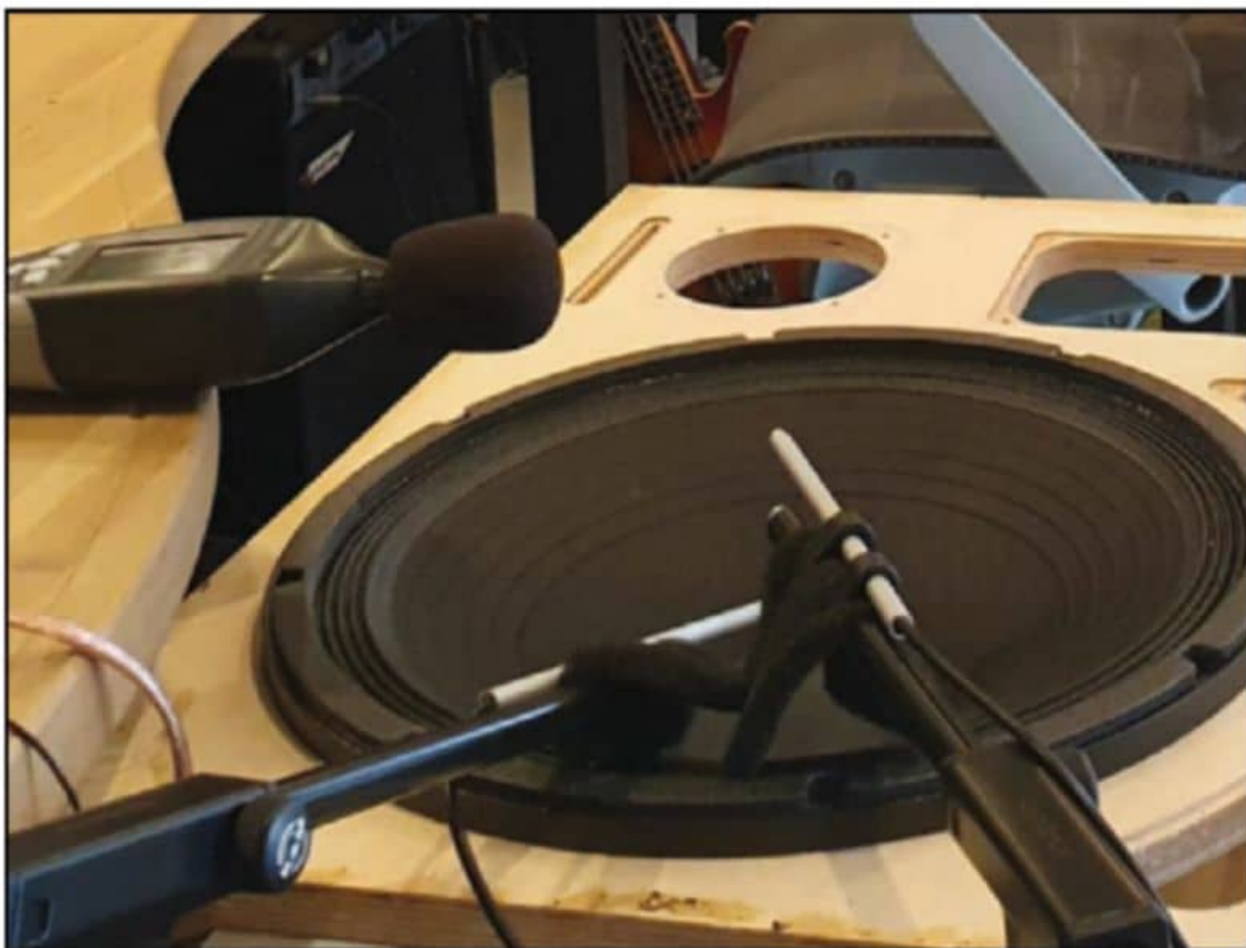
Photo 1: Measurement setup with microphones positioned 5cm and 10cm above the cone
