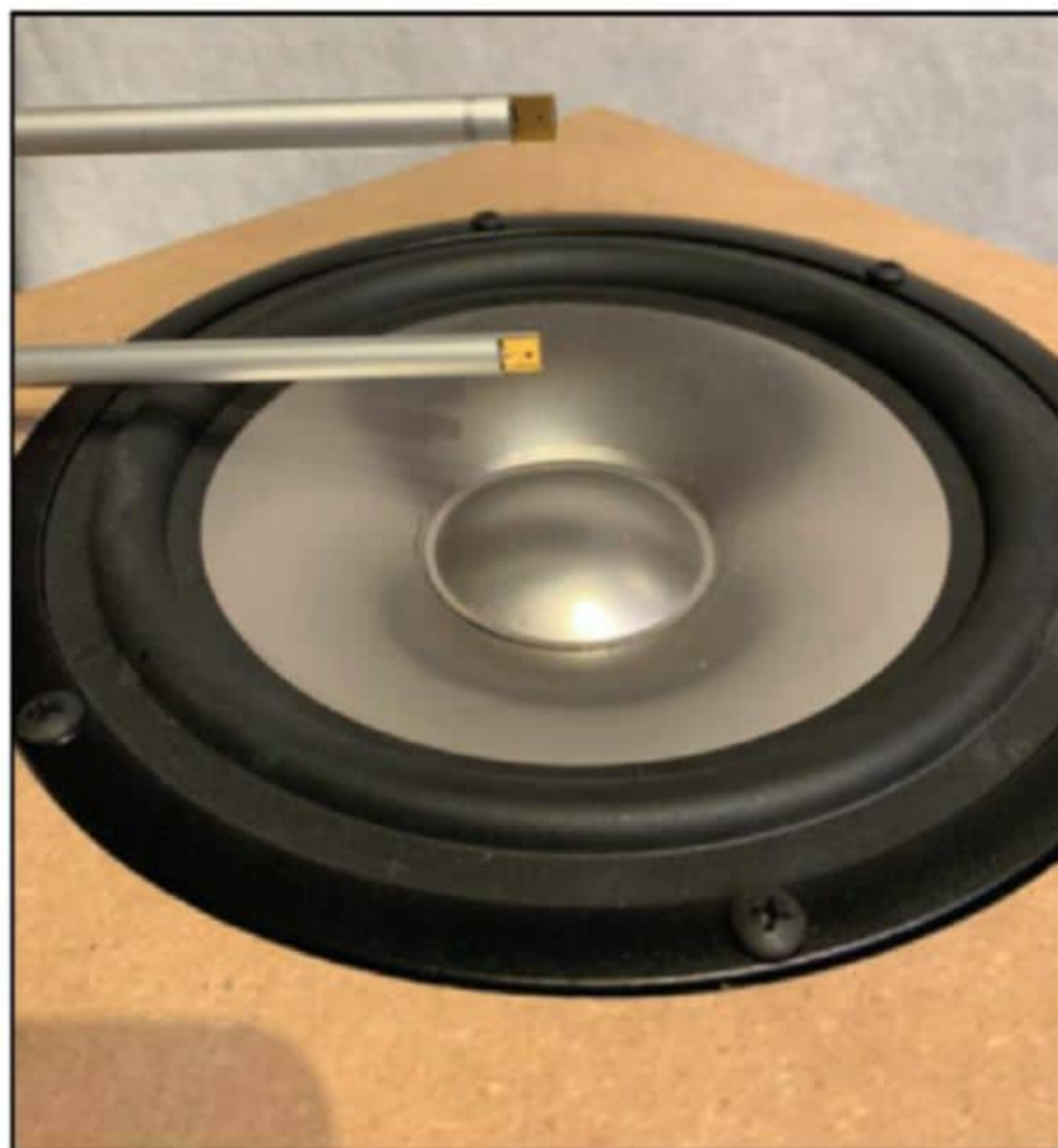
Photo 1: AudioChiemgau has developed an affordable ModeCompensator comprising two calibrated MEMS microphones and the necessary electronics to perform measurement tasks.
