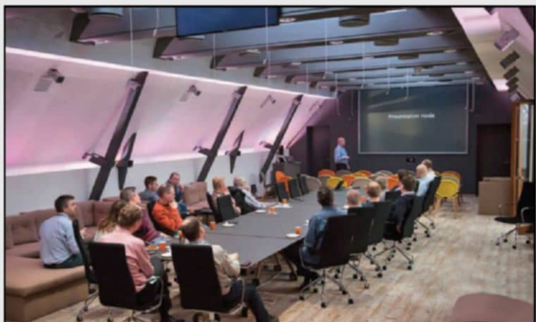
A Meyer Sound Constellation is used in a bank's boardroom, with the multiple microphones and compact speakers visible in the ceiling.
