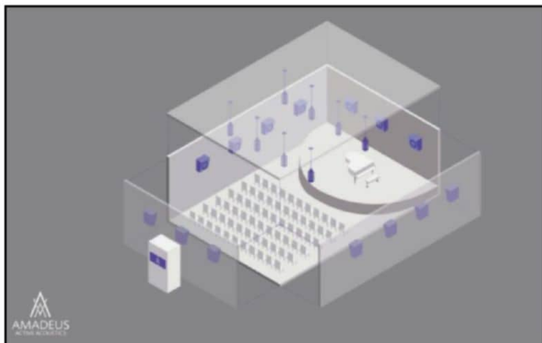
A simplified illustration of an Amadeus Active Acoustics room is shown with microphones and speakers.
