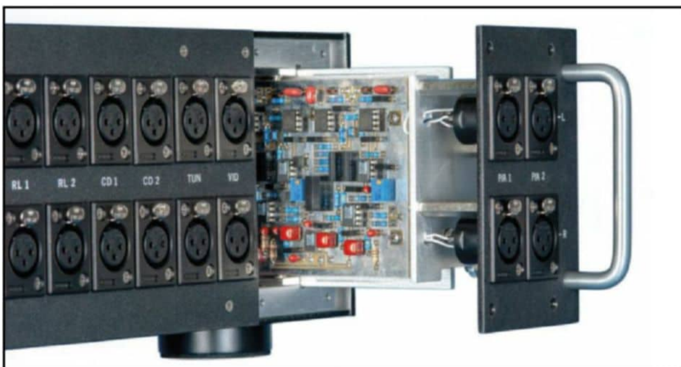
Photo 2: This is the removable dual stereo phono preamp module. This module also employs a differential instrumentation amplifier architecture.
