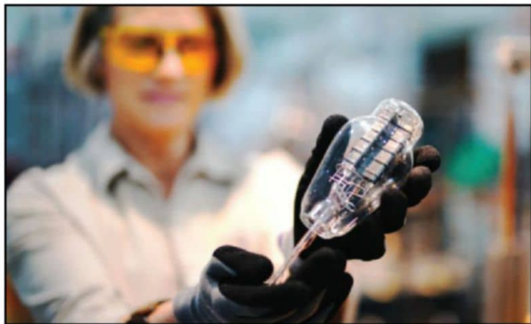
Photo 10: The sealed envelope is ready to be evacuated.
