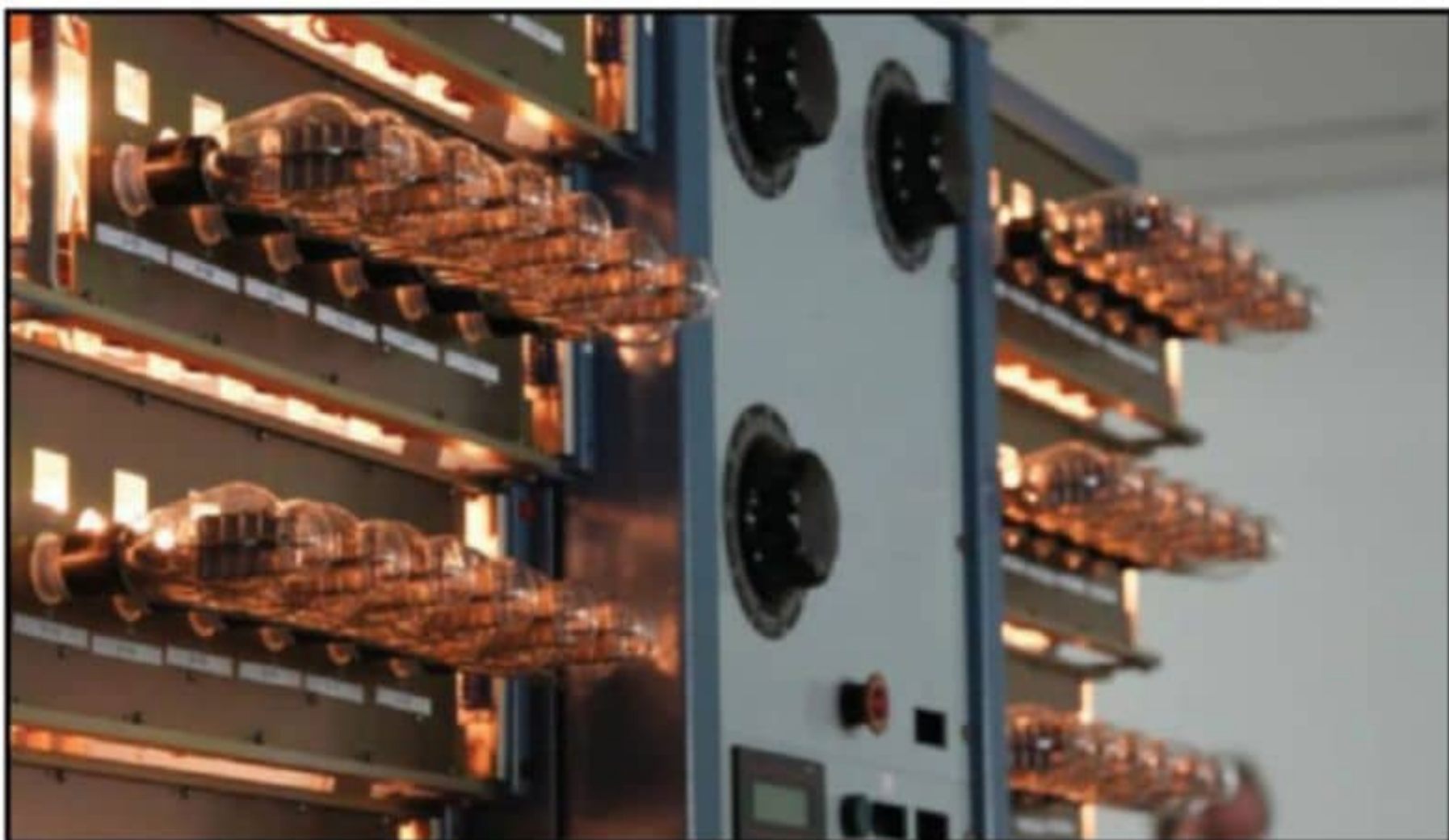
Photo 12: Racks of tubes are aged as the final step. (Photo courtesy of Klipsch Museum of Audio History, Jim Hunter, Curator)
