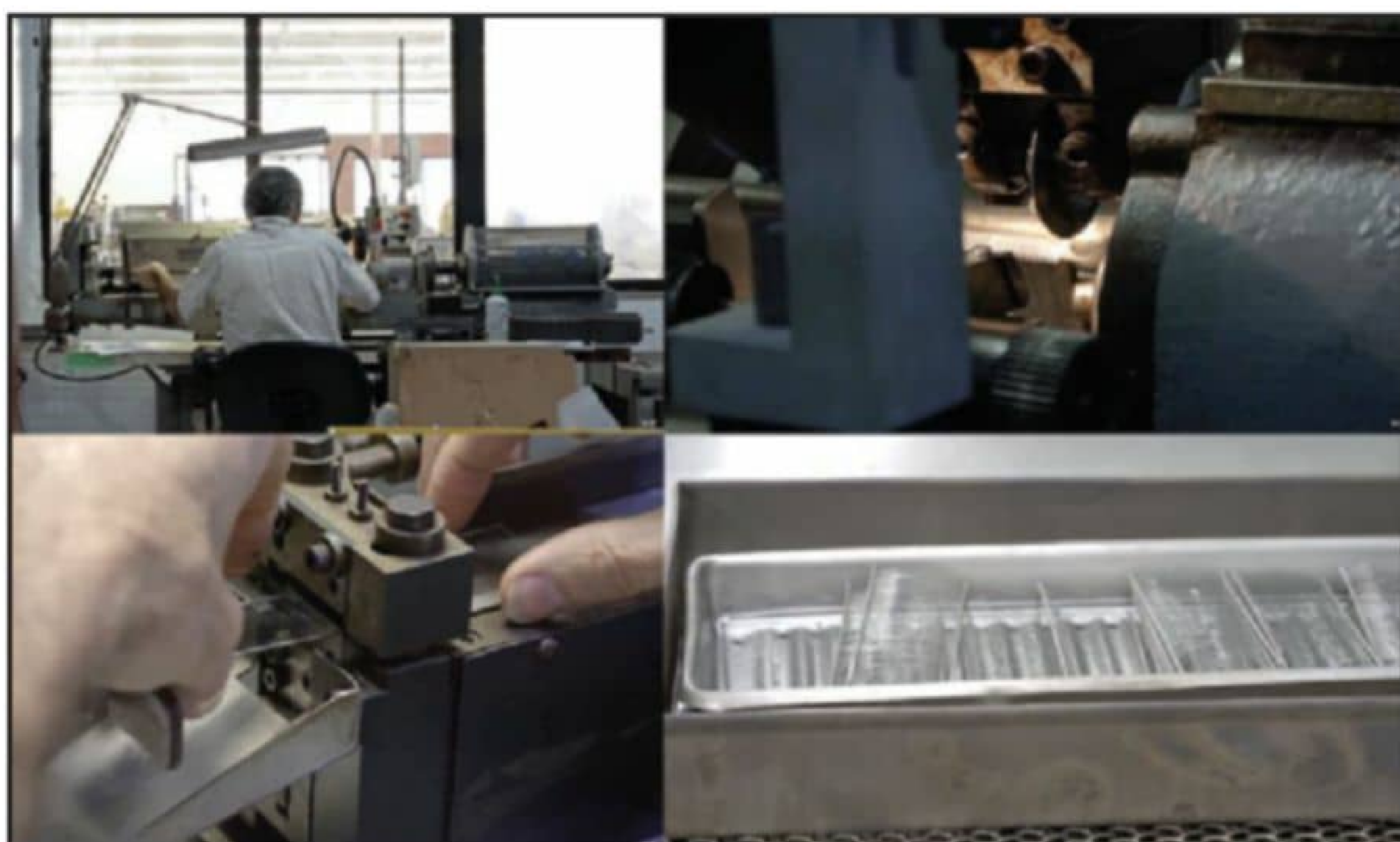
Photo 6: The grid is formed using a special grid lathe machine that Rossville Works carefully preserves.
