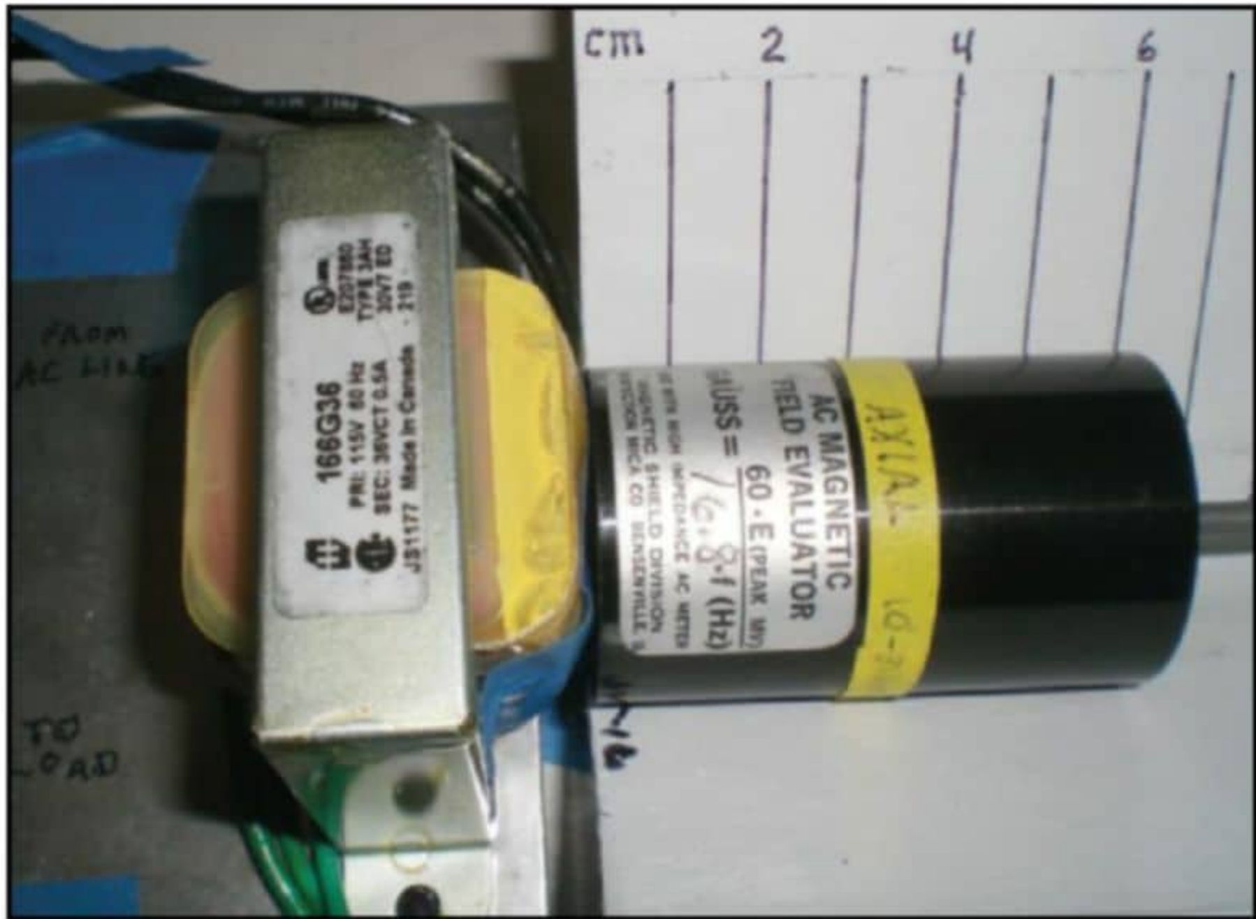
Photo 28: Leakage flux density measurement setup with Hammond 166G36 E-I core transformer mounted on the aluminum plate.
