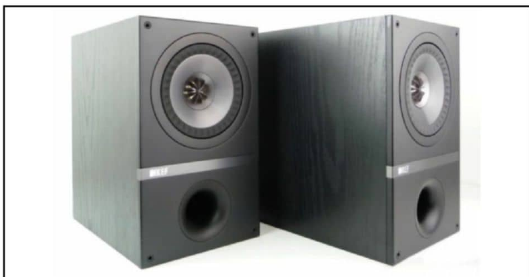
Photo 1: An example of a front ported speaker. A bass reflex system, also known as a ported, vented box or reflex port, explores a port (hole) or vent cut into the cabinet and a section of tubing or pipe affixed to the port. This port enables the sound from the rear side of the diaphragm to increase the output of the system at low frequencies as compared to a typical sealed- or closed-box loudspeaker or an infinite baffle mounting.
