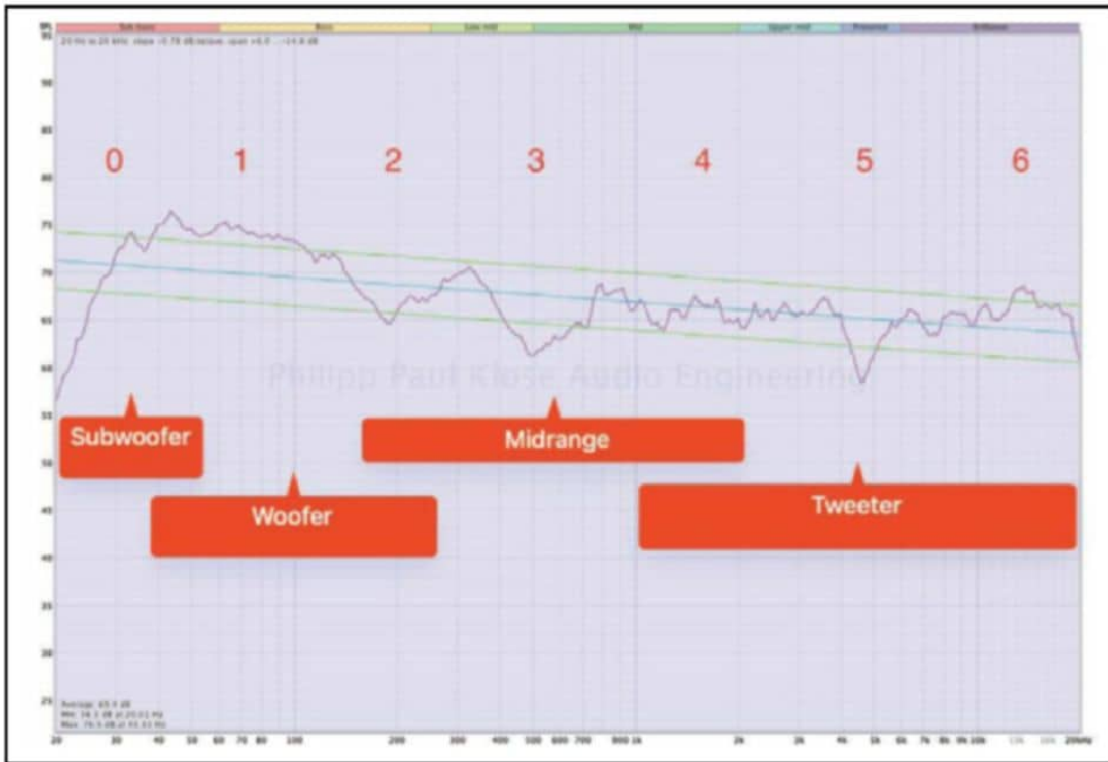
Figure 3: Challenging frequency bands and their approximate coverage from different speaker types.
