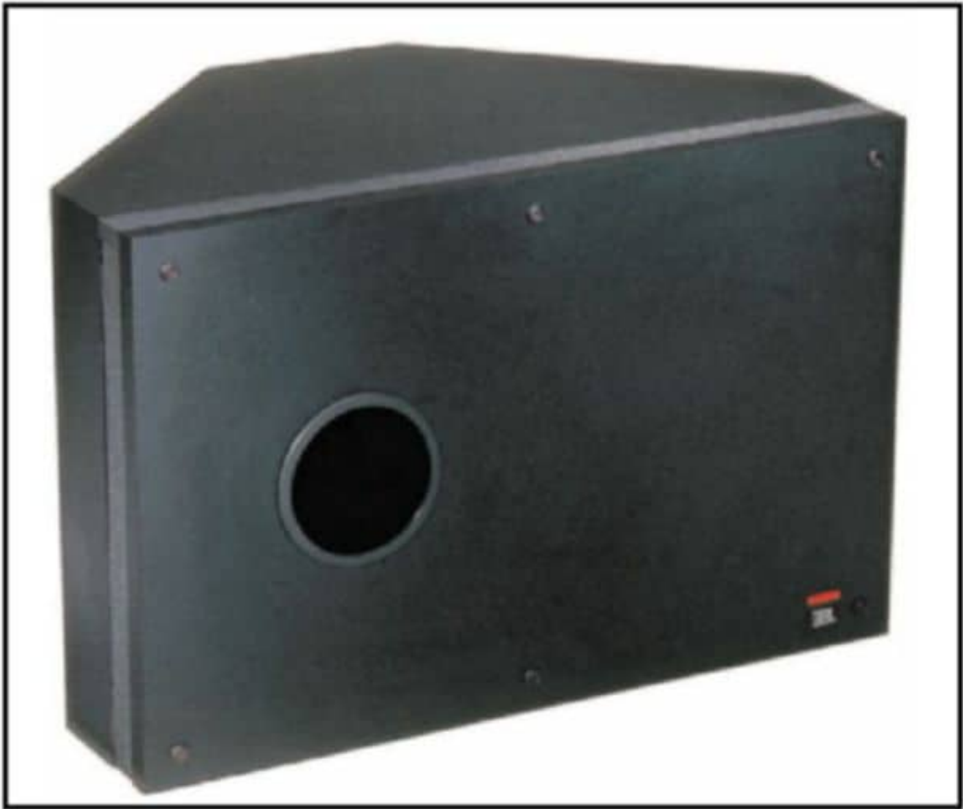
Photo 2: A bass reflex system with an opening called a port or vent cut into the cabinet, generally consisting of a pipe or duct (typically circular or rectangular cross section).
