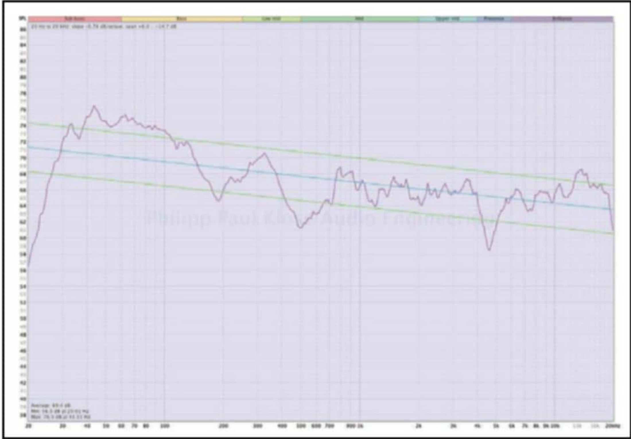
Figure 2: Average of 10 benchmark measurements of premium sound systems in cars (violet). The green lines mark ±3dBr from the blue line showing the overall average. The spectrum tilts approximately 0.75dBr per octave.
