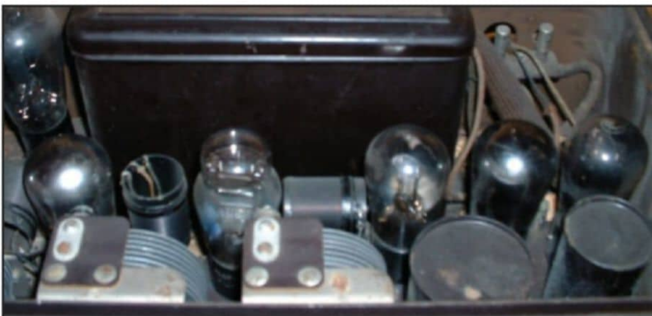
Photo 2: This view of the innards of the Atwater Kent Model 42 shows the huge power transformer, three tuning capacitors, Bakelite-form air-core coils, and six tubes.
