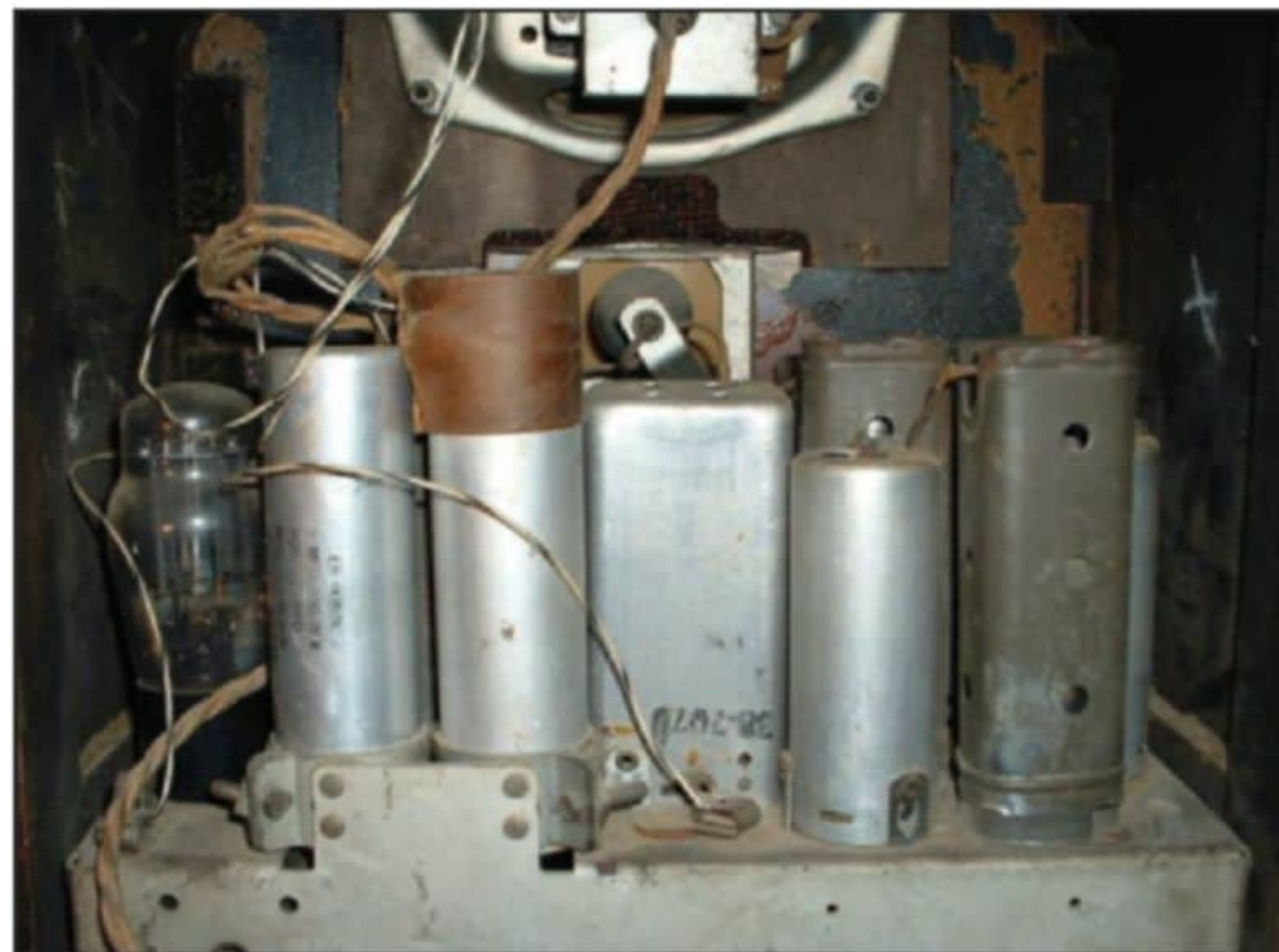
Photo 4: The Philco’s innards are more tightly packed, and show the bottom of the electrodynamic speaker, several electrolytic can capacitors, one tube with a “coke-bottle” envelope, and shields around the inductors and some of the other tubes.
