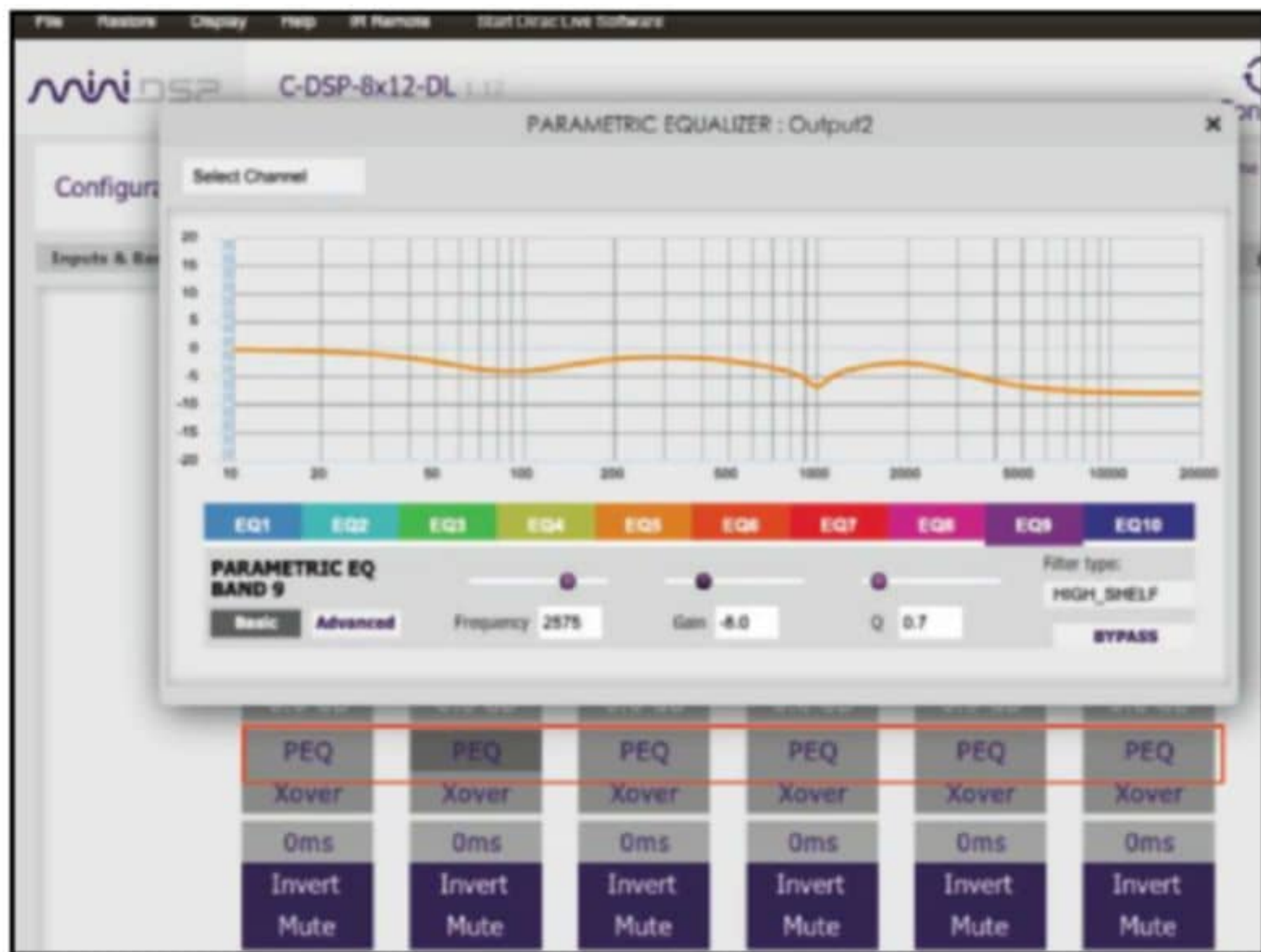
Figure 11: 10-band EQ per output channel.
