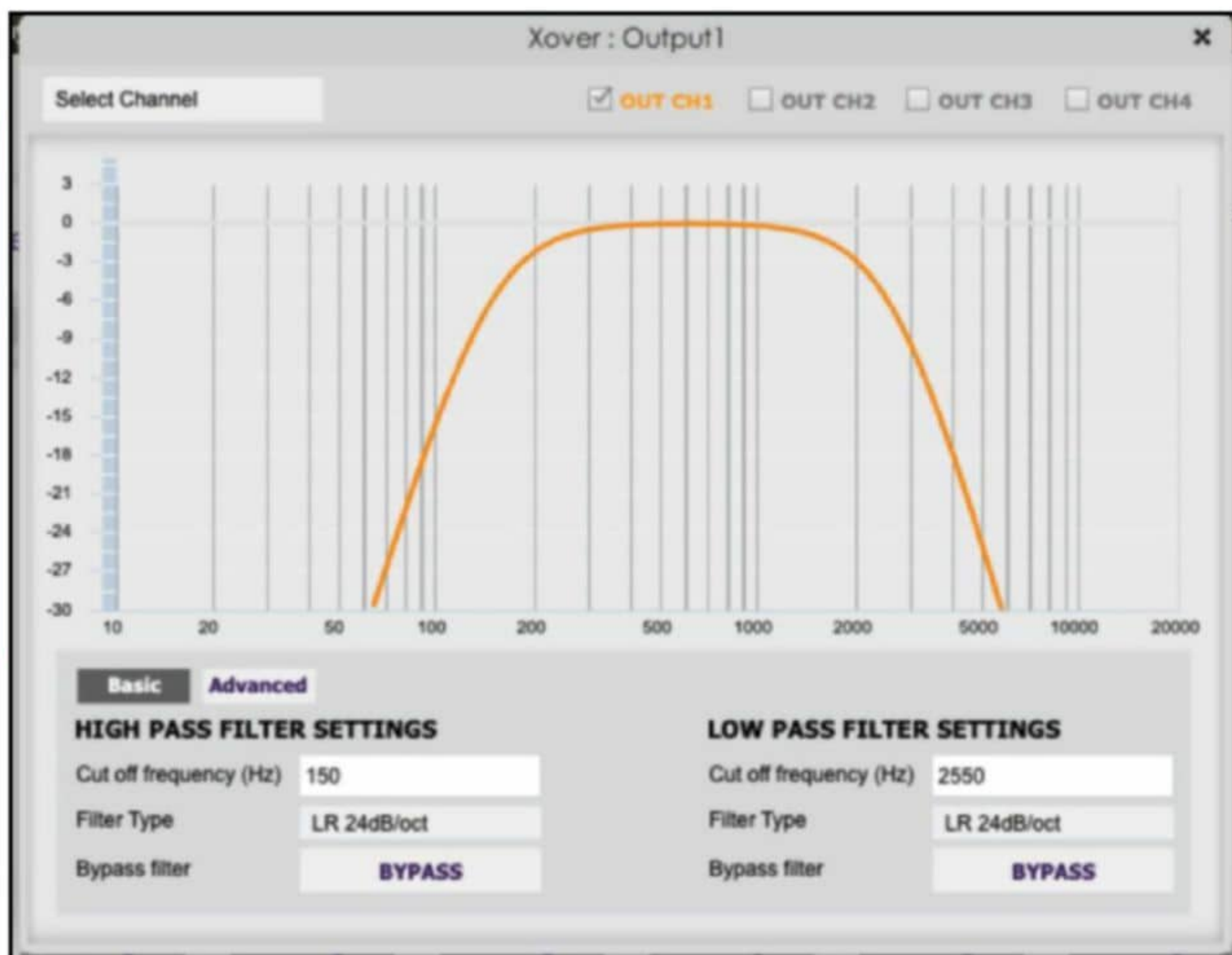
Figure 4: Crossover setup for a midrange speaker. The frequency range of the speaker is cut off at 150Hz and 2550Hz with Linkwitz-Riley (LR) filter.
