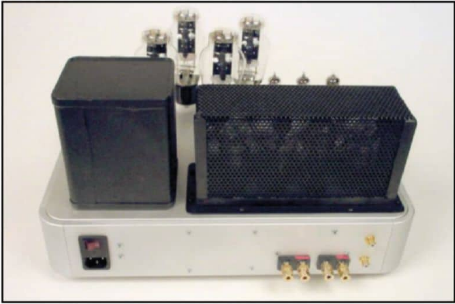
Photo 14: The rear view of the completed project shows the connectors.
