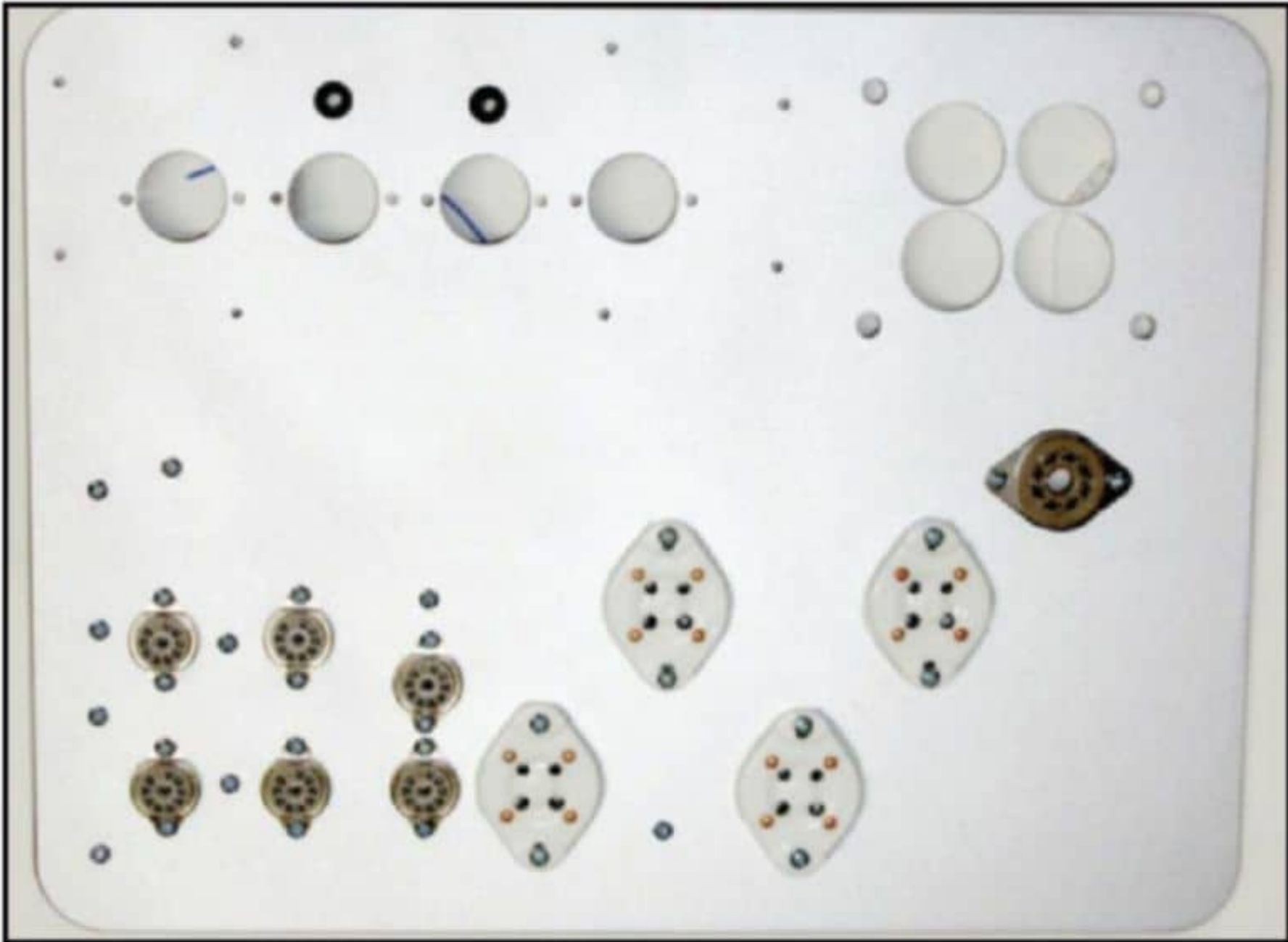
Photo 10: This is the top of the chassis with the new tube sockets.
