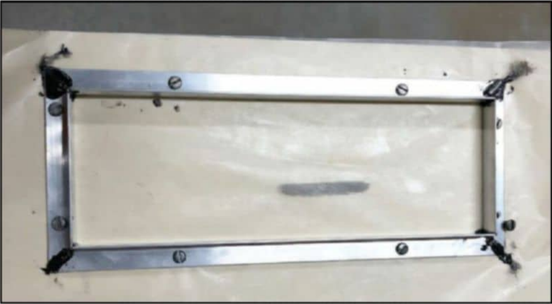
Photo 7: I used strips of right-angle aluminum to assemble the tube cage base.
