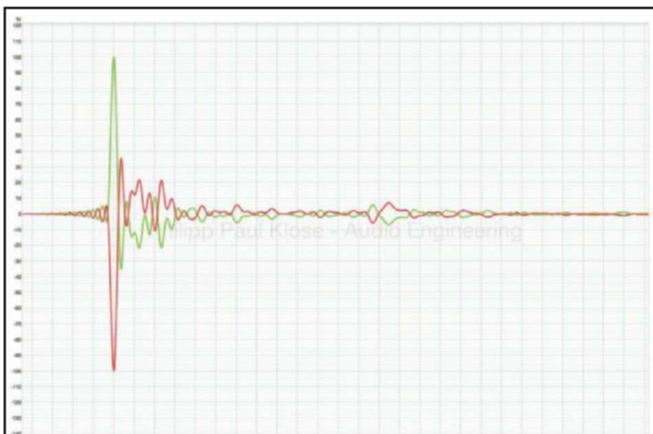
Figure 3: Polarity check through an impulse response from a log sweep measurement: Positive (correct and expected) polarity in green, vs. negative (incorrect and unexpected) polarity in a speaker setup.
