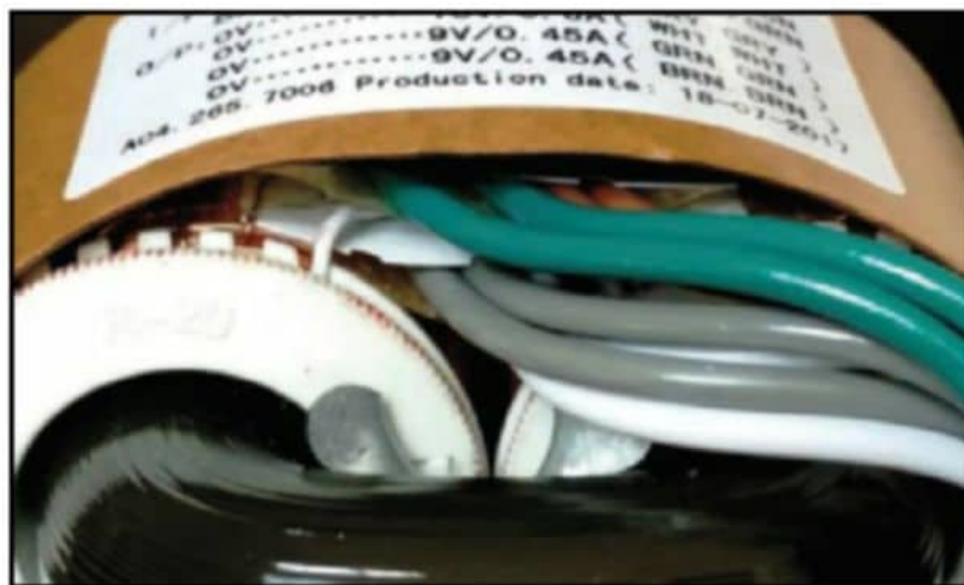
Photo 23: R core toothed gear-drive bobbin end plates and notched splicing area on a finished transformer. The curved steel mounting plate retainer lugs are visible above the curved ends of the core.
