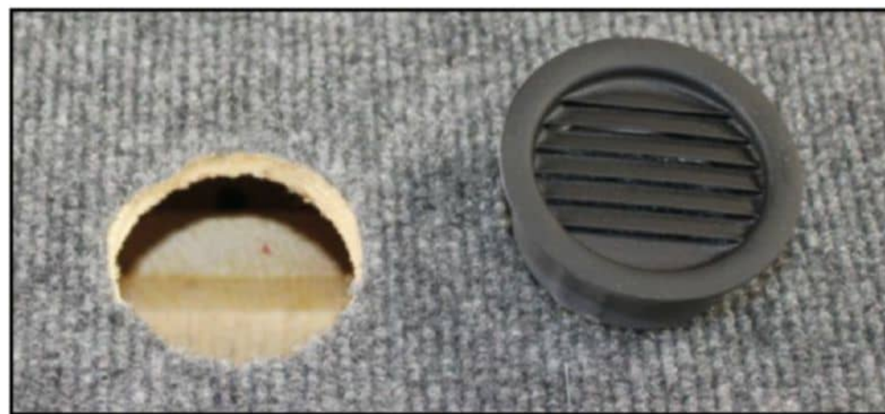
Photo 10: The amplifier soffit vent is mounted in the center of the top over the amplifier pad.
