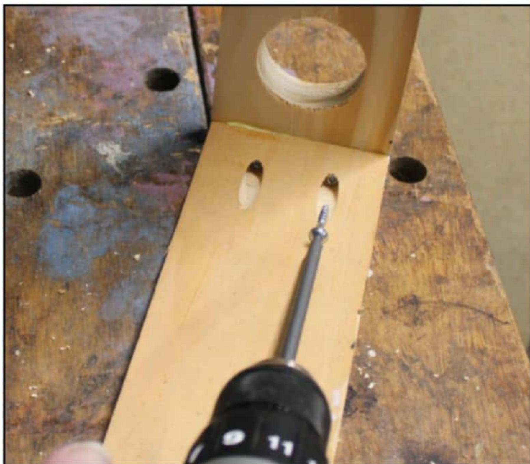
Photo 8: Corner joints in the Soundbase were glued and fastened using a "Kreg" drilling jig that leaves no exposed screw heads in the structure.
