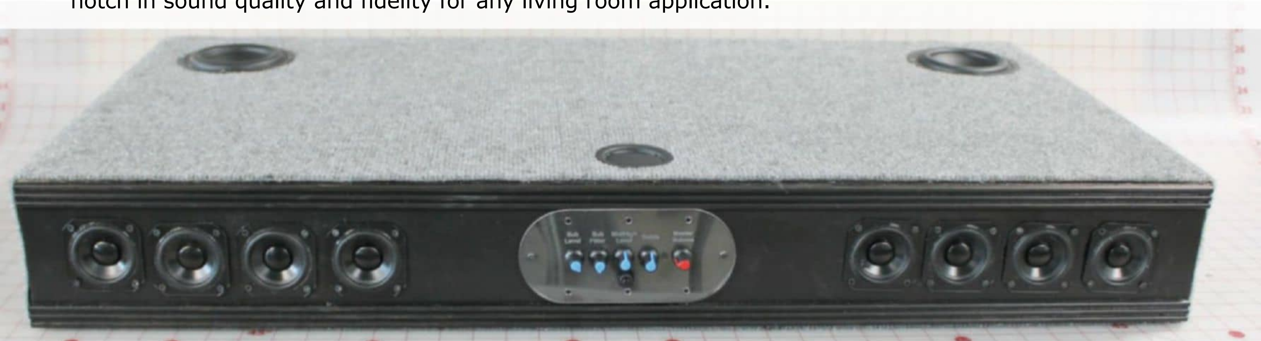
Photo 1: The completed Soundbase shows the woofer placement, which allows up to a 65" TV to be placed on it without interference.
