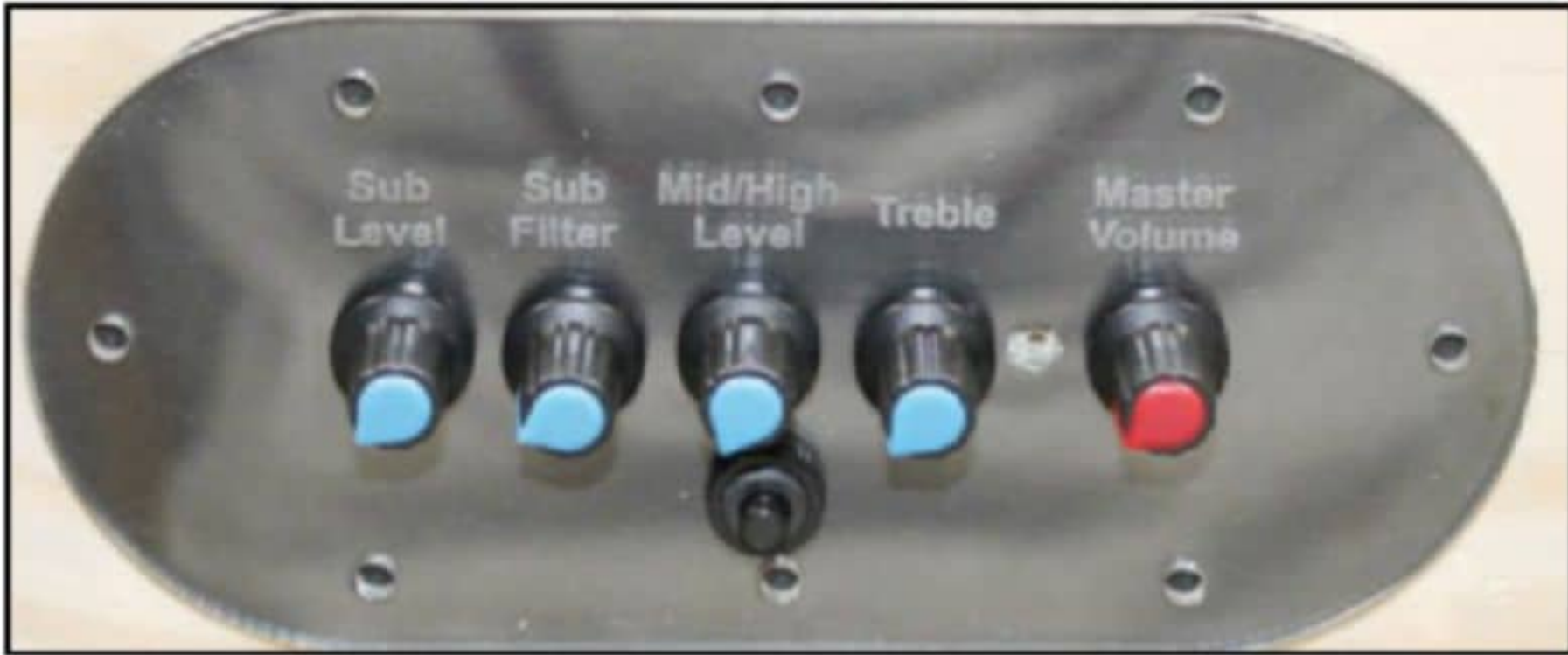
Photo 13: Detail of the amplifier front panel shows the added on/off switch.
