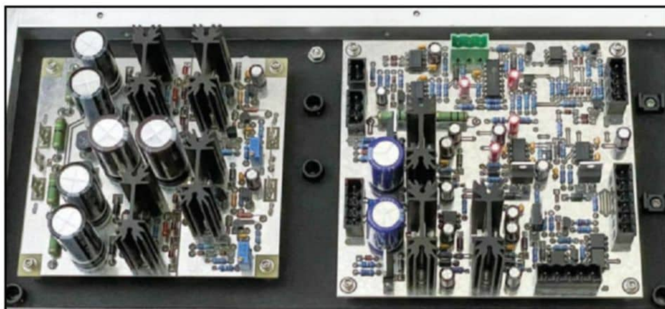
Photo 4: The High Voltage Regulator CCA (left) and Low Voltage Regulator/Protection CCA (right) are mounted on the chassis partition.
