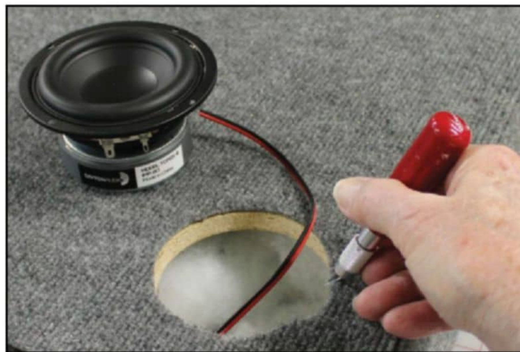
Photo 11: The carpet covering the Soundbase was cut for the woofers after being attached to the top.
