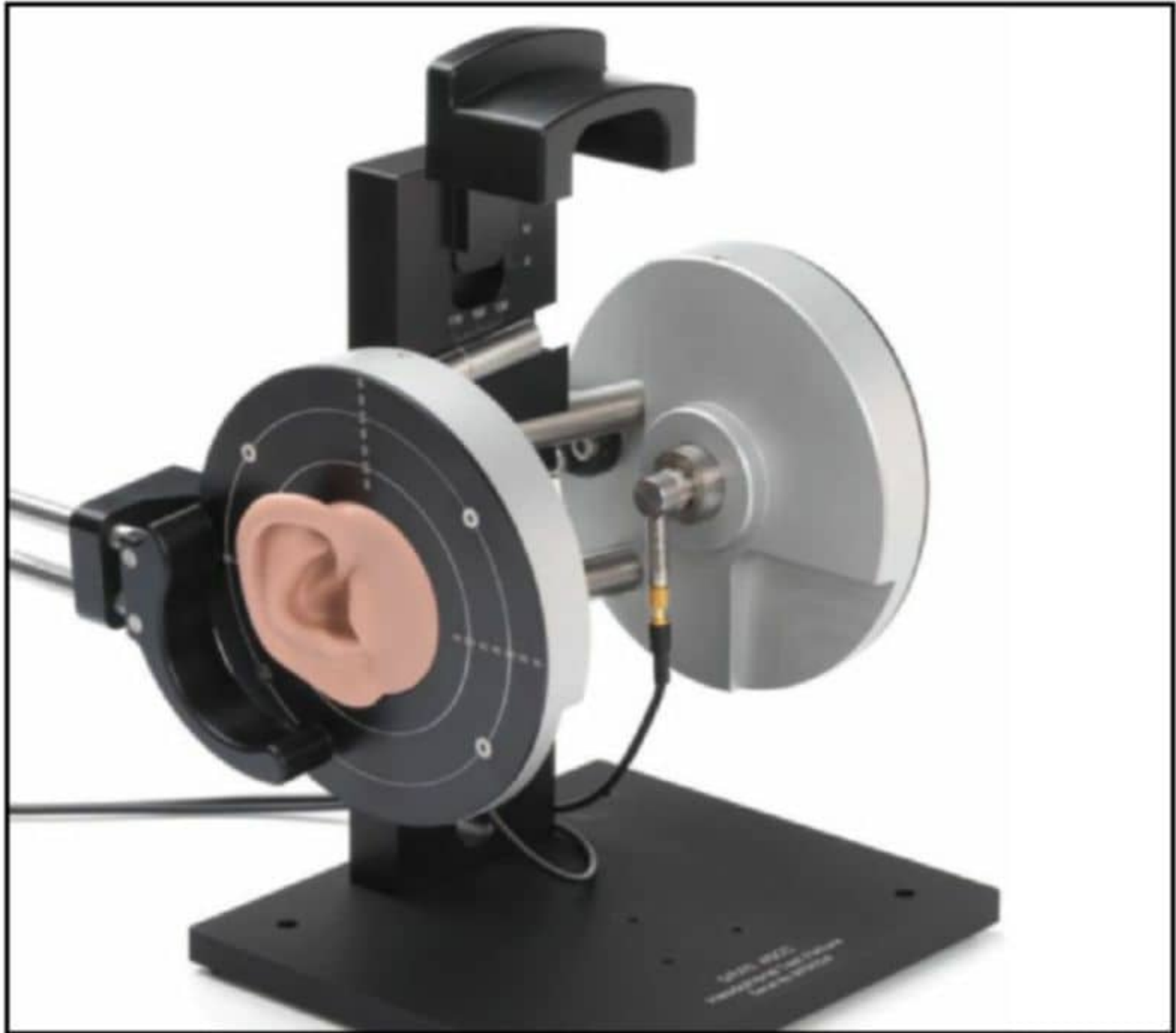
The 45CC platform already has a solid footprint in the testing market and GRAS now offers four new versions that are ideal for test scenarios that require or benefit from realistic human-like acoustic loading and ear geometry when testing any headphone or earphone type (around ear, on ear, in ear, and insert).
