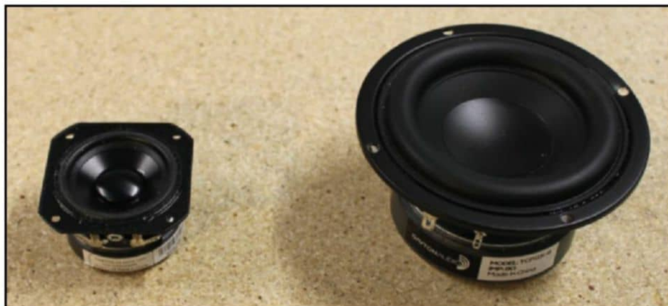
Photo 3: The Peerless 2" drivers and one of two Dayton 4" subwoofers used in the Soundbase are shown here.
