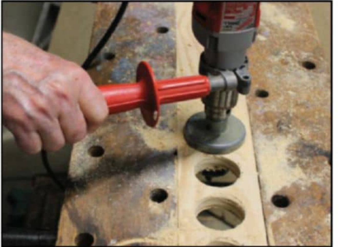
Photo 7: Use a 2" hole saw to cut the front panel speaker mounting holes.
