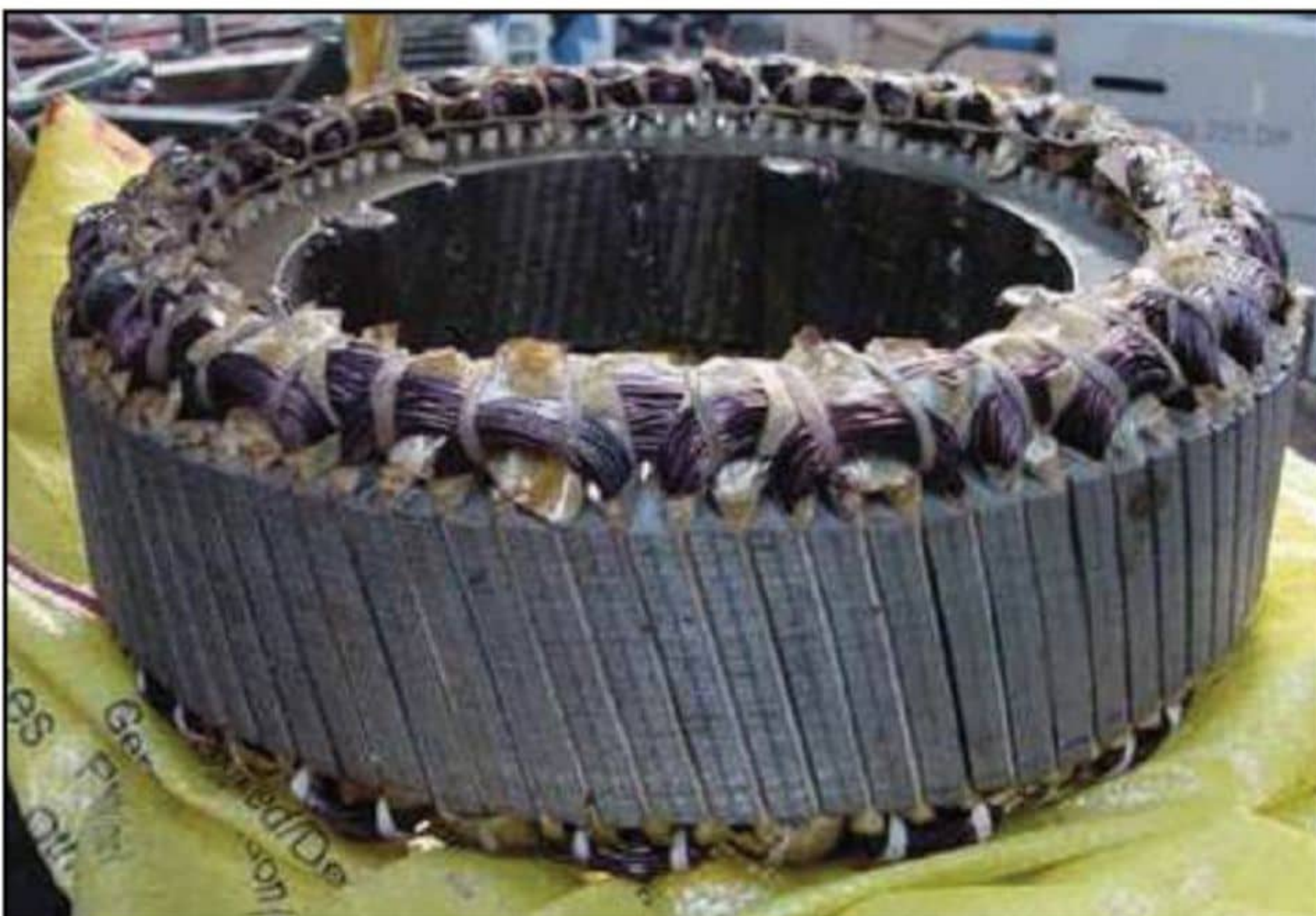
Photo 16: Generator stator skew to minimize slot harmonics (Image Source: The Back Shed)
