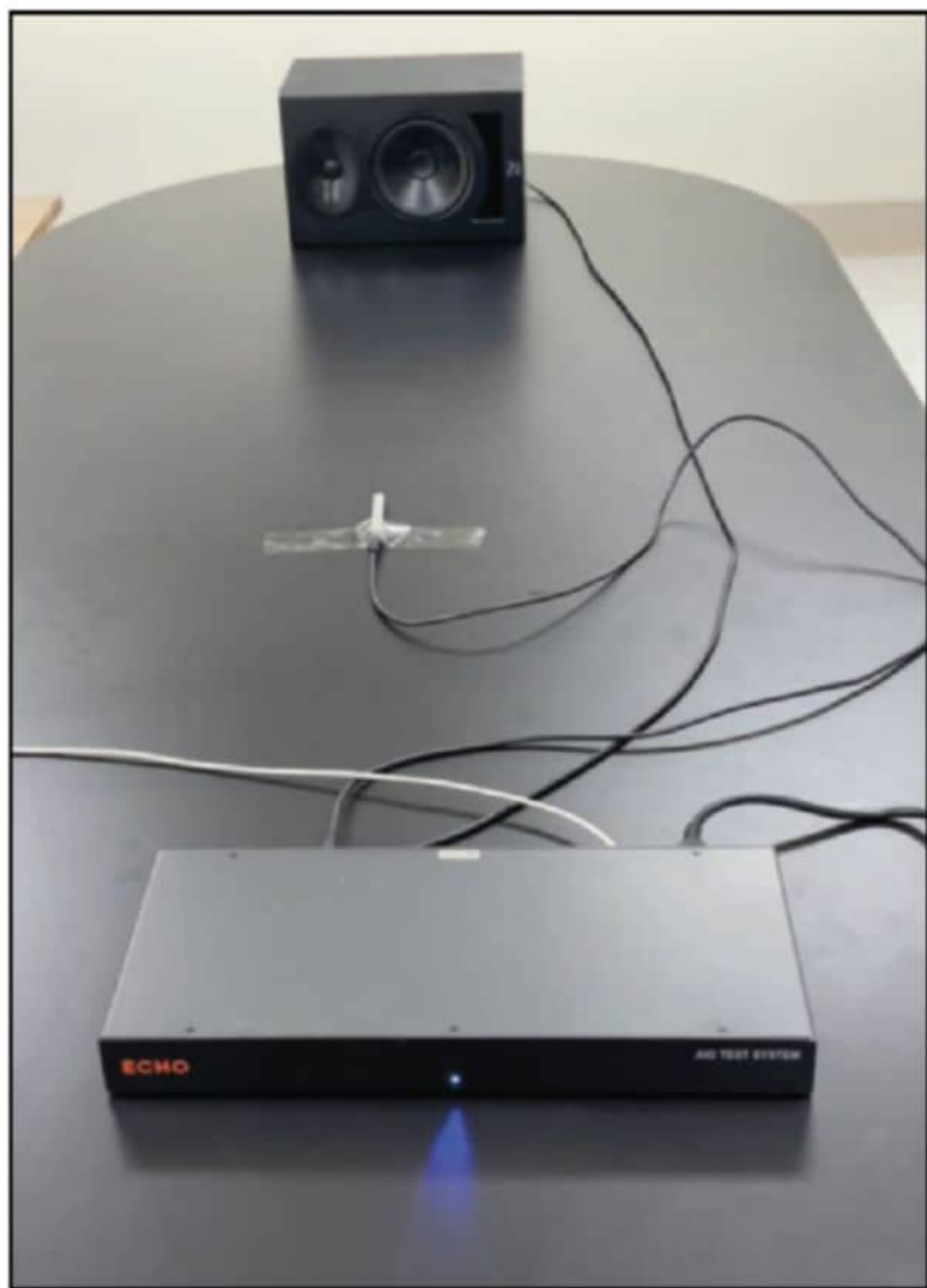
Figure 3: The ICP/CCP inputs of the Echo are TEDS-capable.
