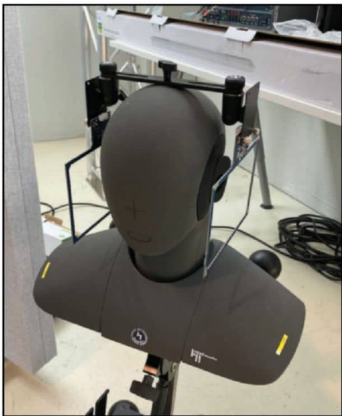
Photo 2: A good working combination is a HEAD acoustics artificial recording head combined with a Umik-X array with two miniDSP Uma-4 modules.
