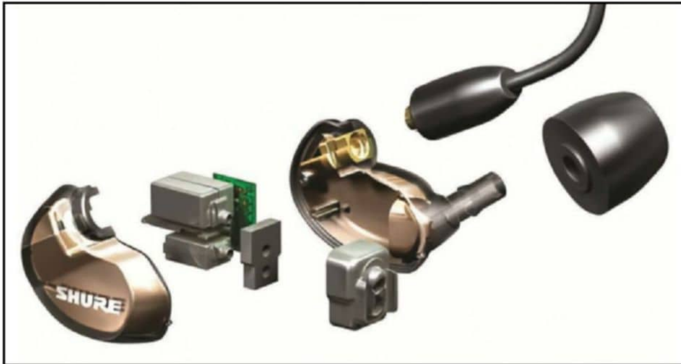
Figure 7: Exploded view of the Shure SE535 earphone. Thanks to Gojko Obradović for suggesting this Shure earphone as an example.
