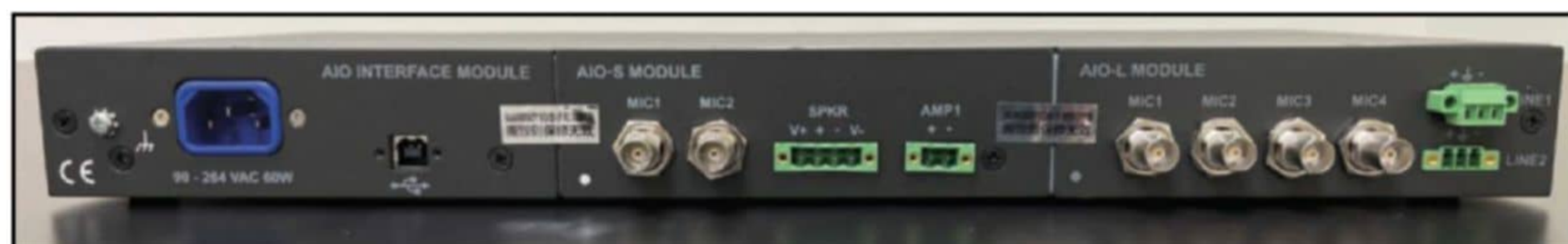
Photo 2: The "mainframe" has the power and the USB interface, then space for two modules chosen by the user to customize the test system.
