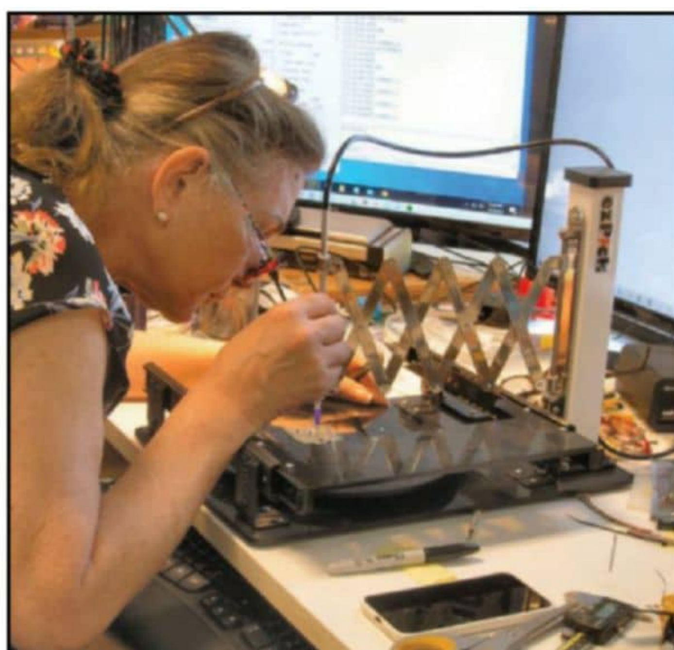
Photo 4: Julia's pick and place machine lets her precisely place teeny SMD components onto the even smaller solder pads of the PC board.
