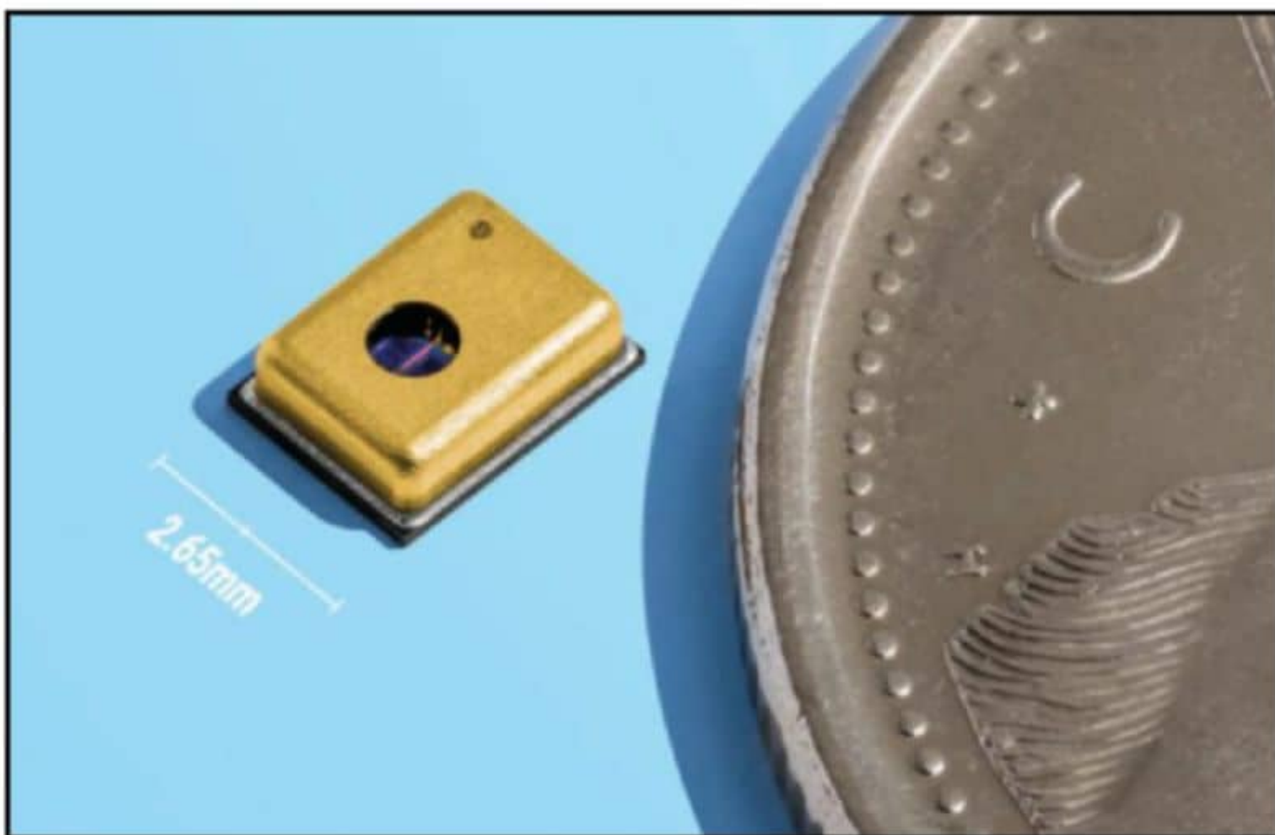
The Soundkrit SKR0400 directional MEMS microphone is able to isolate a person's voice while eliminating any other sounds and noise surrounding it.
