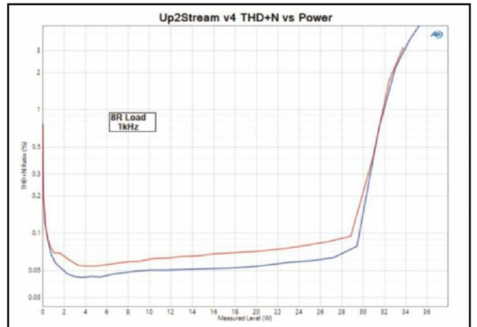
Figure 7: The V4 in stereo mode is capable of over 30W of power into an 8R load.
