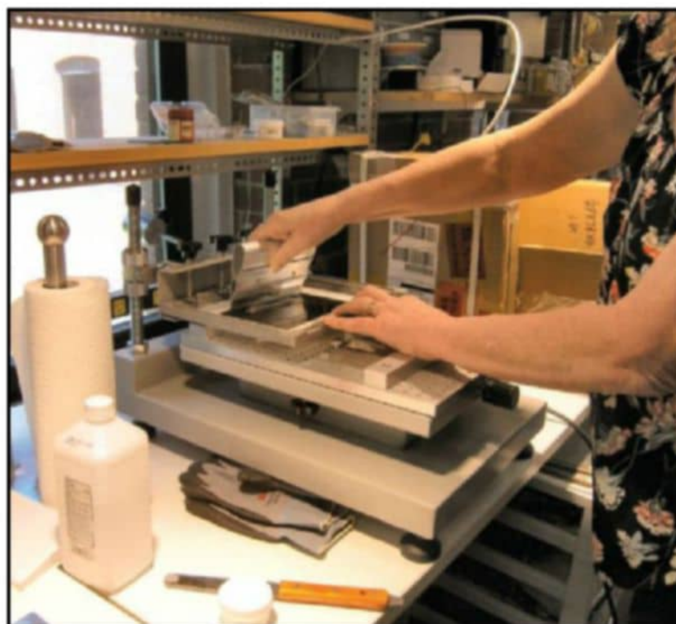
Photo 3: Black belt engineer Julia Truchsess uses a squeegee to apply solder paste to the PC board while the board and template are held in a special jig.
