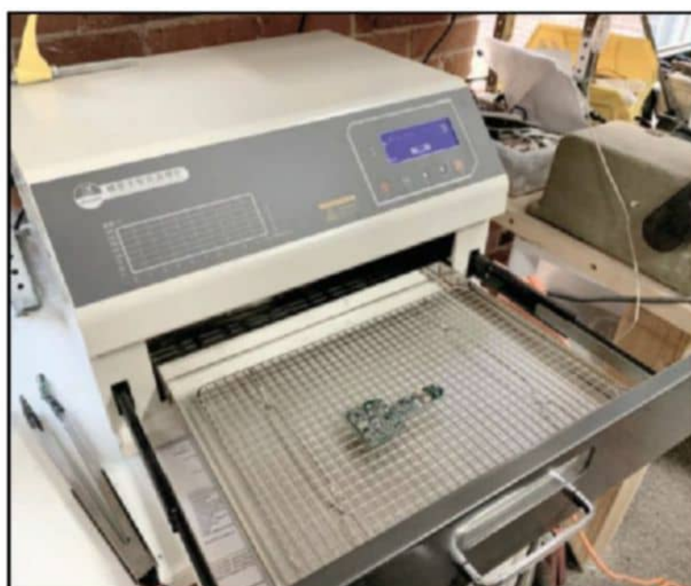
Photo 5: This oven from AliExpress lets you program a sequence of temperature changes to rise, sustain, rise again, then fall at rates matching the solder paste's specs.
