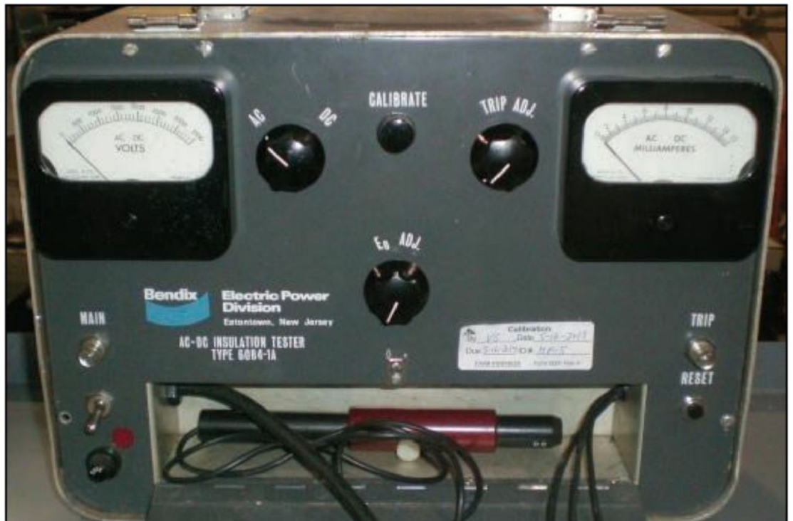
Photo 15: After transformer construction is finished, a high-potential (hi-pot) voltage test is applied with special insulation resistance and high-voltage test equipment. Shown here is a Bendix Type 60B4-1-A AC/DC Insulation and hi-pot tester.
