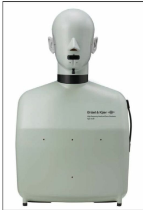
Photo 2: Another source that simulates a human mouth is the B&K Head-and-Torso Simulator (HATS).
