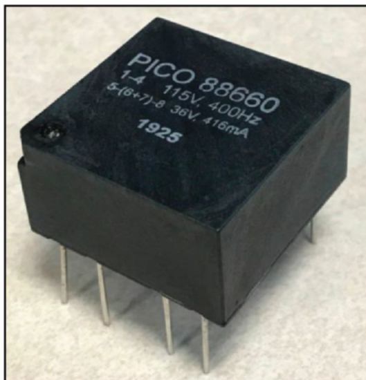
Photo 10: This is a MIL-PRF-27F Grade 5 encapsulated PC board-mounted power transformer. This particular one is a Pico Electronics 88660, 15VA toroidal transformer designed to MIL-PRF-27F Grade 5 Class S, with PC board pins (Image Source: Pico Electronics, Inc.)
