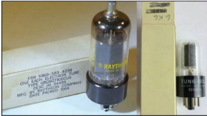
Photo 3: The 6BQ6GTB horizontal output tube and the 6K6 audio power pentode were used primarily in TVs.
