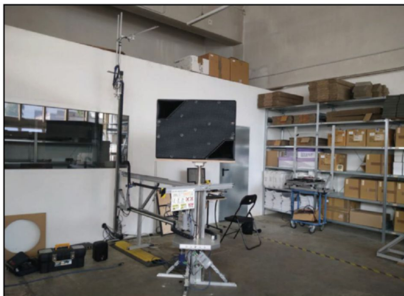
Figure 3: NFS measurement setup is shown for a full-space 4\pi scan of the X1 audio module.
