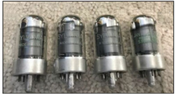
Photo 4: A variety of loctal tubes were used in car radios and guitar amps in the 1940s.
