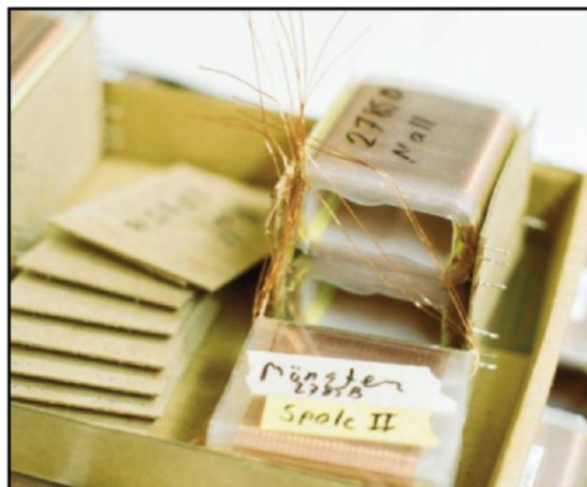
Photo 2: Double coils are assembled onto mounting plates ready for the cores.
