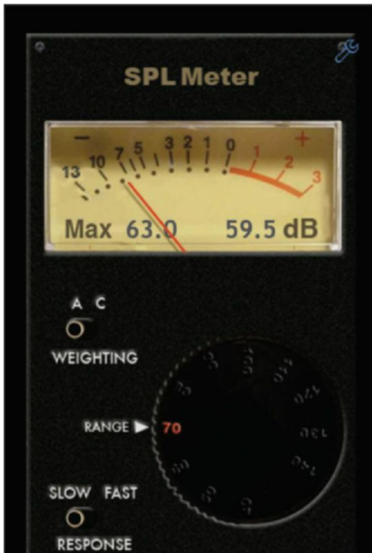
Photo 5: The Studio Six SPL Meter includes choices of “A” or “C” (flat) weighting and “SLOW” or “FAST” response time.
