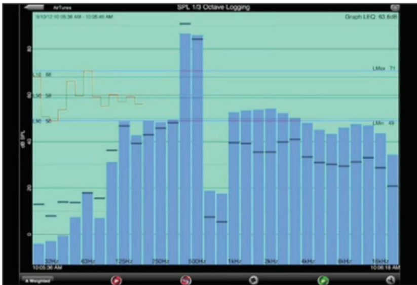
Photo 9: The Studio Six Octave and 1/3 Octave Band Logging function displays the frequency content of noise.
