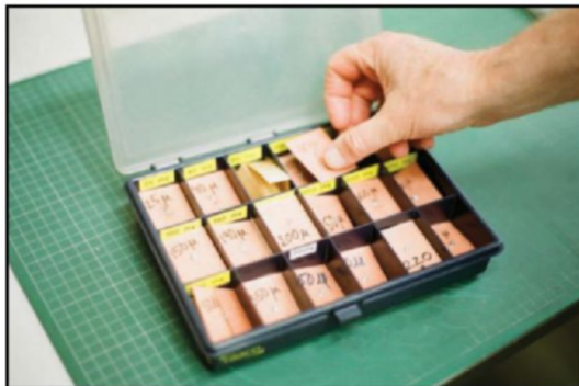
Photo 7: Spacers for core gaps
