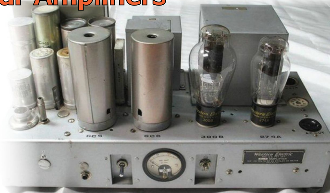
Photo 1: This Western Electric model 91A is a classic single-ended vacuum triode power amplifier.
