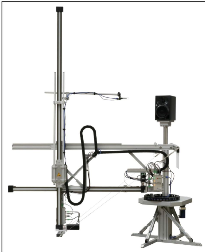
Photo 2: Measurements can now be made in a 3D space in both conventional anechoic and non-anechoic rooms. An example of this is the Klippel Near Field Scanner (NFS), which is a mechanical scanner that moves a single microphone around a loudspeaker system, or an individual transducer mounted in a baffle to effectively generate a “balloon measurement.”
