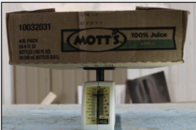
Photo A: A cardboard tray centered on a postage scale can be used to measure polyester stuffing in ounces.
