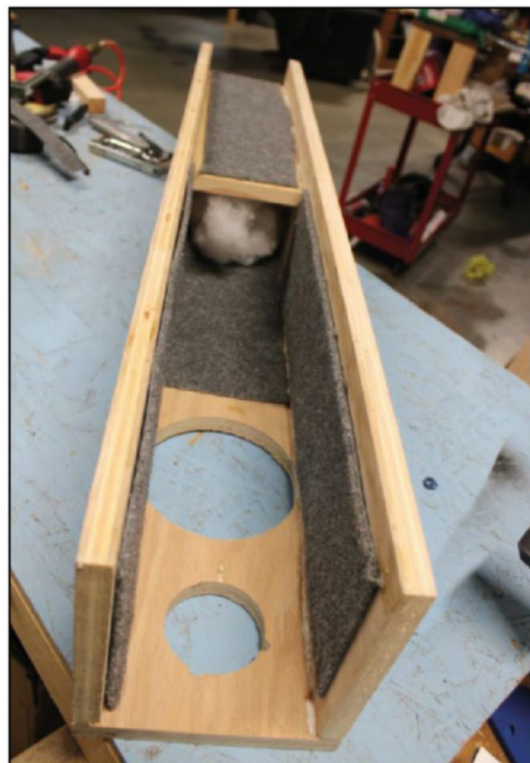
Photo 4: This image shows the application of the internal carpet in the tunnel area.
