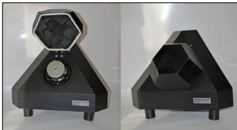
Photo 3: This is an outline of a Tetrahedral Test Chamber, with an acoustic isolator shown open (a) and closed (b).
