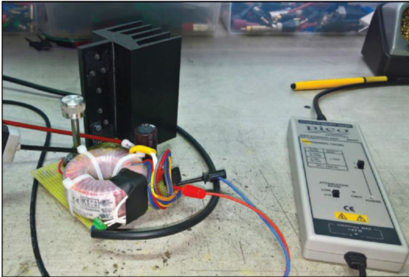
Photo 3: The little transformer (shown here) almost behaved as expected, with the output voltage near 30V DC at a full load of near 500mA DC for an output power of near 30W.
