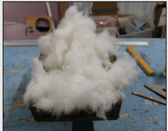
Photo B: This angry looking storm cloud is actually 6 ounces of polyester stuffing that was used in the upper portion of the system.
