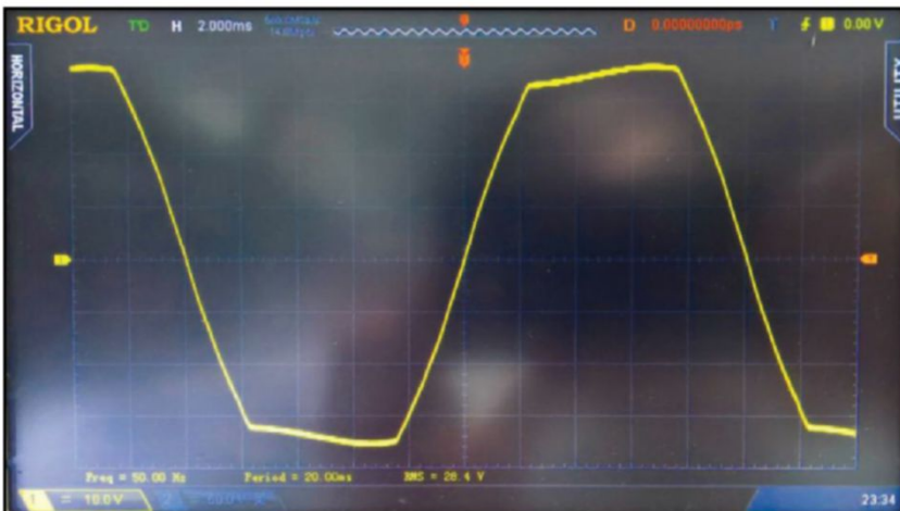
Figure 2: The oscilloscope trace, at full load, looks like a square wave with less steep flanks.
