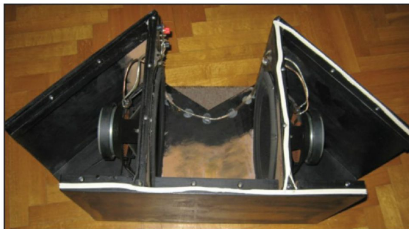
Photo 2: To fit the space, I designed a unique cabinet, the W-frame subwoofer cabinet, with three openings: the common, the left, and the right opening.
