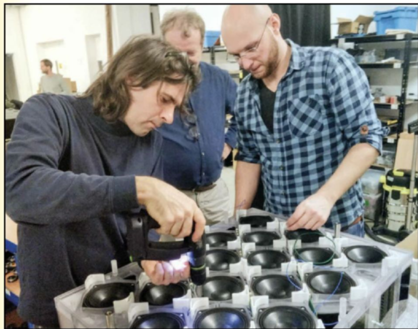
Assembly of the first beta prototype of X1 at our offices, before Holoplot had a dedicated production site. The first beta prototype was milled out of plastic, and played for the first time in December 2018.
