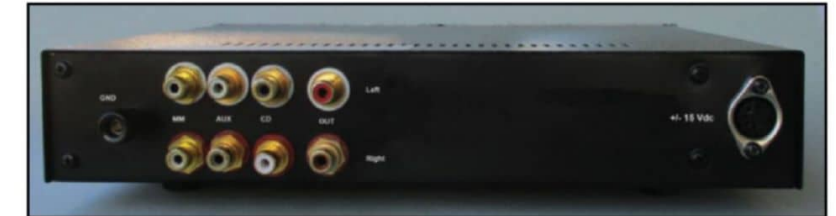
Photo 2: The back panel has a 5-pin DIN connector and eight gold-plated RCA femal connectors.
