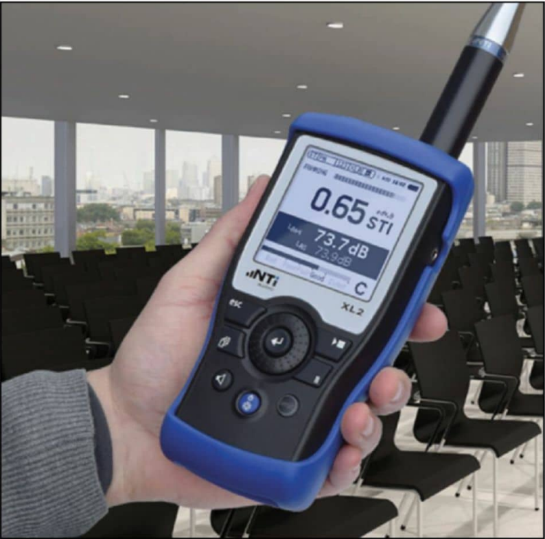
Photo 4: The NTi XL2 functions as a STIPA meter, sound level meter, RTA, spectrum analyzer, and vibration analyzer.
