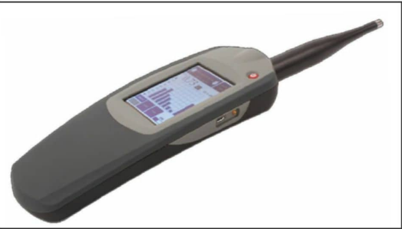
Photo 3: The Bedrock SM50 measures full STI (65-second measurement) as well as quick STIPA for screening, and functions as a sound level meter and RTA.
