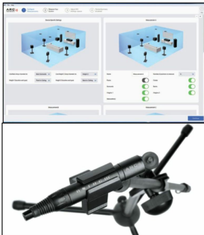
The Anthem Room Correction (ARC) helped establish sound correction at home, being supplied with a microphone and software, with corrections uploaded to the Anthem Electronics or Paradigm processors.
