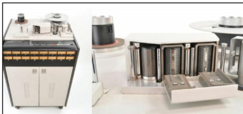
The Ampex MM-1200 16-track 2" tape machine introduced in 1976 was used in countless hit records in the 1970s and 1980s. There were 24-track (2") and 8-track models (1" tape) also manufactured.
