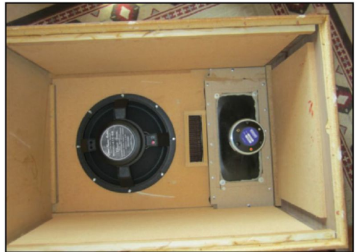
Photo 5: Here is the inside of one of the Altec Lansing enclosures with both drivers in place.
