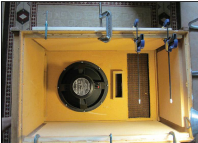
Photo 4: I added extra strengthening to the cabinet.
