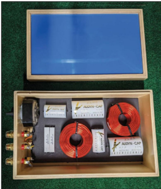
Photo 8: I used wooden “card file” boxes I purchased from a department store to house the components.
