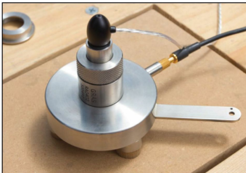
Photo 4: The Megaclite is being measured in a GRAS RA0402 high-resolution coupler.
