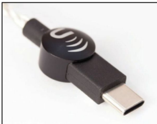
Photo 3: The integral amp-DAC dongle on the source end of the Megaclite's cable
