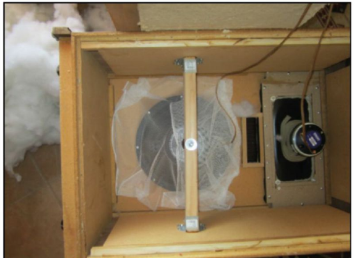
Photo 7: I put a net over the woofer to keep any pieces of the wool from encountering the woofer cone.
