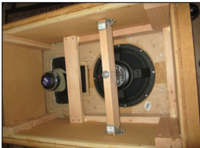
Photo 6: I added a cross brace, which has a provision for adjusting the tension it applies to the rear of the woofer.
