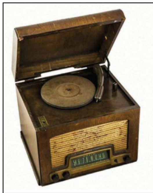
Photo 5: This 1940s-vintage Arvin radio-record player was convenient, but its relatively small speaker limited its fidelity.
