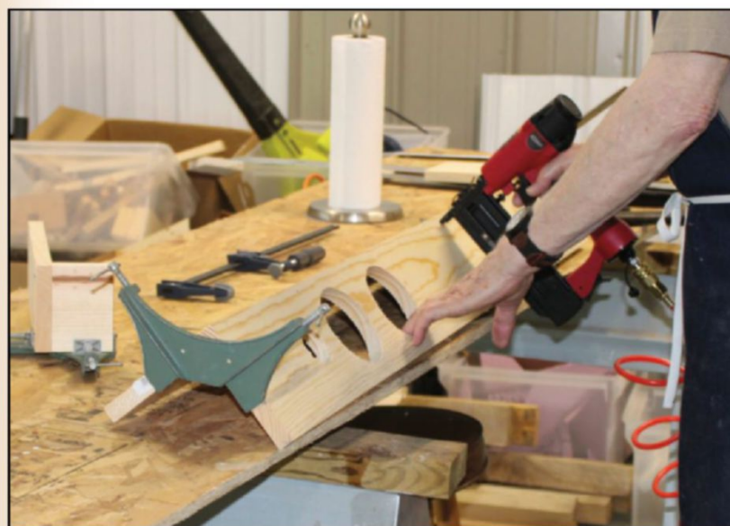
Photo 6: Use corner clamps to hold the assembly while the walls are glued and nailed together.
