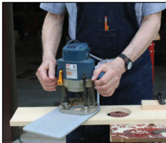
Photo 3: Use a Jasper router jig to cut the speaker holes.
