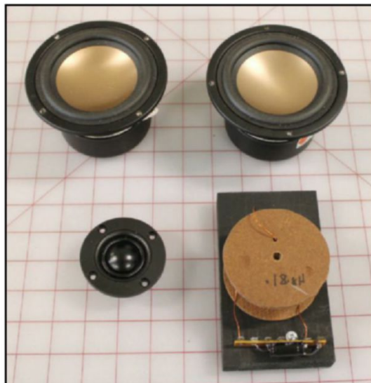
Photo 1: The drivers used in the system include the two Hi-Vi woofers and a Dayton Audio 1" dome tweeter. The crossover was hand wound and consist of a 0.18mH coil and a 10µF capacitor.
