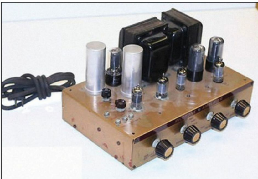
Photo 6: The Pilot Model AA-903 mono hi-fi amplifier was used as a control-room monitor amplifier in many broadcast studios, as well as in many homes.
