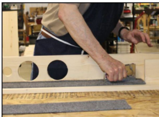
Photo 4: Add indoor/outdoor carpet to the enclosure sides.
