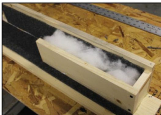
Photo 5: Polyester stuffing is added to the lower cavity of the enclosure.
