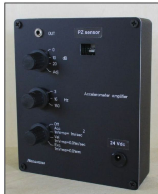
Photo 2: For the completed amplifier. I used the same metal box from Hammond and the aluminum frontplate that I had designed for the ACH-01 amplifier.
