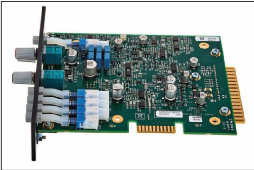
The Solid State Logic (SSL) Alpha VHD-Pre is considered one of the best solid-state mic preamps in the market today, allowing for up to 75dB of gain. Available in rack-mount and 500 series modules, it is an example of a very flexible preamplifier thanks to its Variable Harmonic Drive (VHD) circuit, originally designed for the famous SSL Duality studio console.
