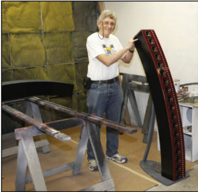
Photo 11: Inventor Don Keele shows a CBT array made for location on a floor (ground-plane use). There is also a model designed to be suspended. These are available as kits.
