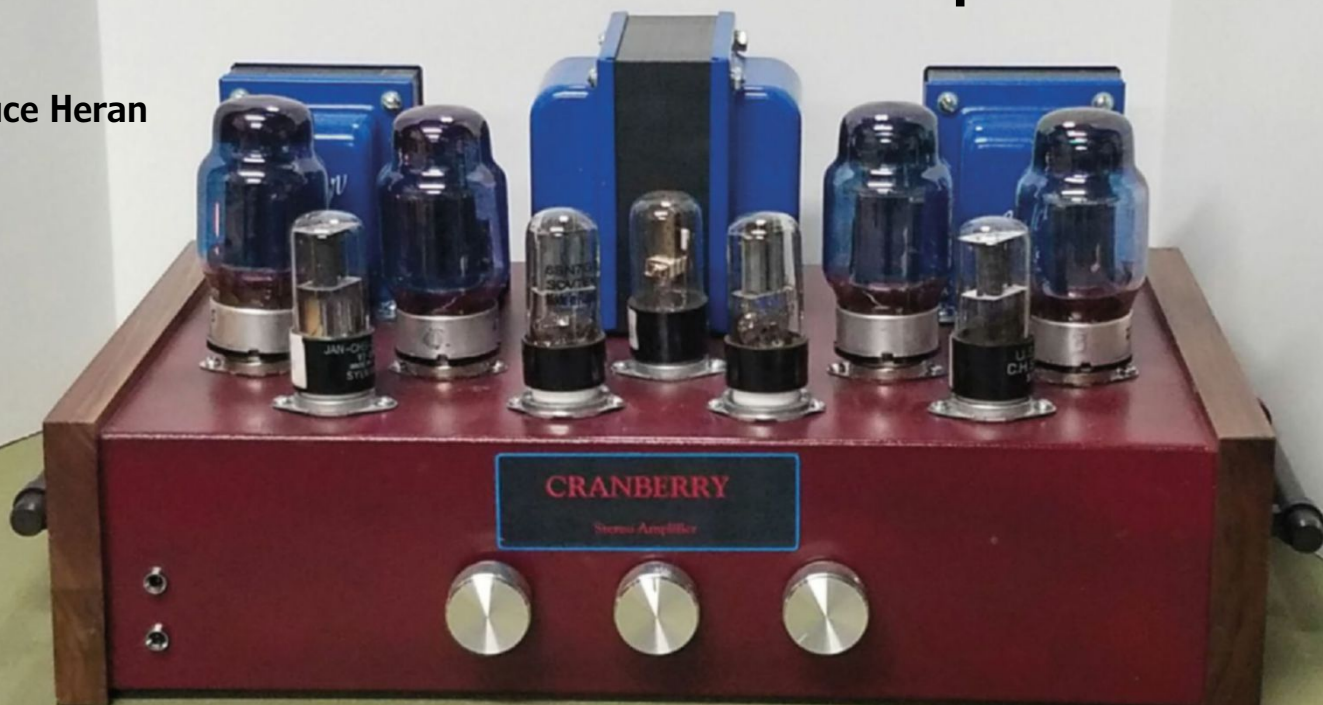
Photo 1: For this project, Bruce Heran built a versatile stereo vacuum tube amplifier that has a single chassis and a shared power supply that he calls the "Cranberry" due to its unique color.
