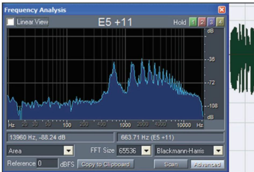
Photo 4: The spikes at the fundamental and overtone frequencies of a cornet playing a trill are wider.
