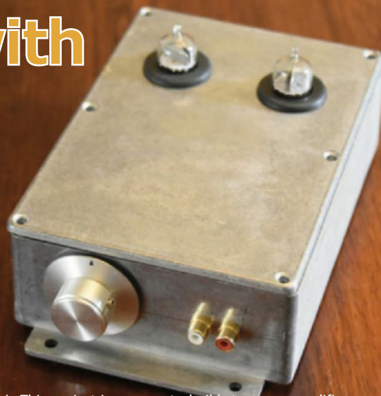
Photo 1: This project is an easy-to-build stereo preamplifier with matched vacuum tube and solid-state signal paths.
