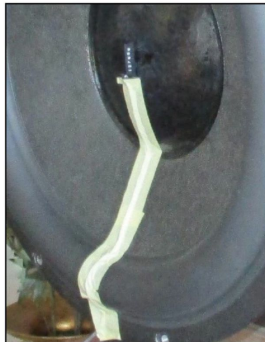
Photo 3: Masking tape is used to firmly attach the cable.
