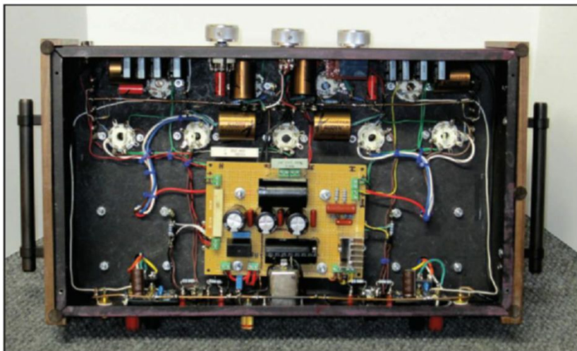
Photo 3: The interior layout shows the partial modular design with most wiring point to point.
