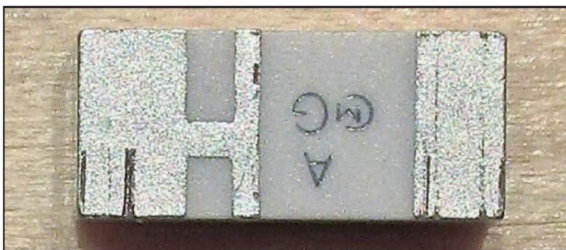
Photo 5: The Murata vibration sensor
