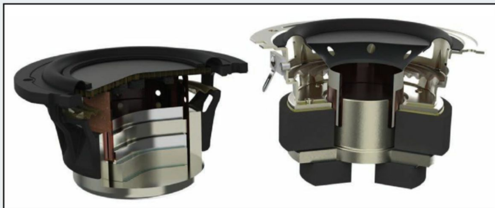
A BMR driver with the composite panel (left) vs. a traditional driver (right)
