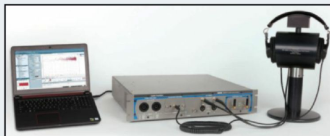
The APx517B Acoustic Analyzer paired with a GRAS 45CA Headphone Test Fixture to demonstrate headphone performance measurement.
