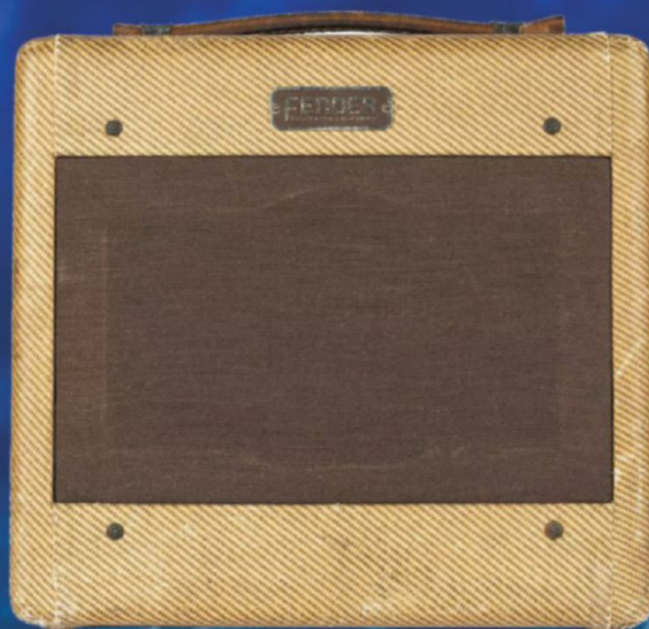
Photo 1: Long a popular small guitar amp, the Fender Champ was available for a time as model 5C1, using a 6SJ7 pentode preamp tube.
