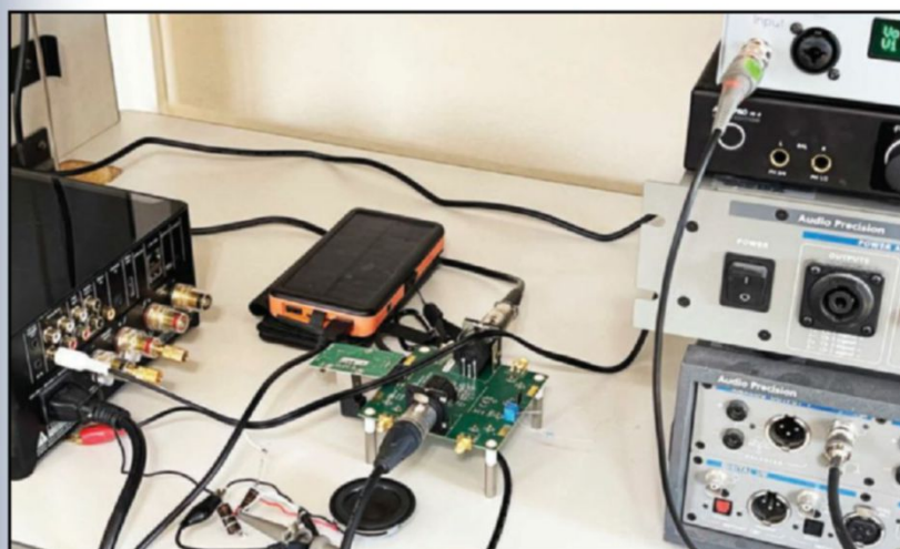
Photo 2: Taking measurements is not always pretty. This is a kluged together setup to simultaneously measure current and voltage when driving a small loudspeaker.
