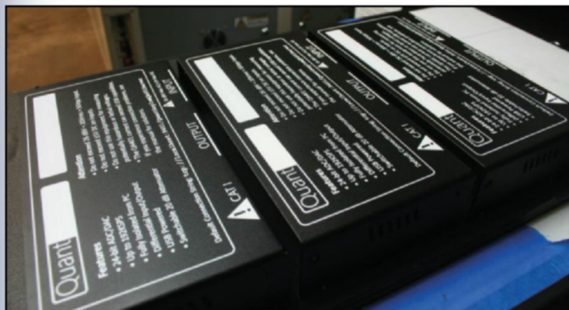
Photo 4: Three top cases are printed in parallel with a UV color printer. After the white layer is complete, the color layer is printed next.
