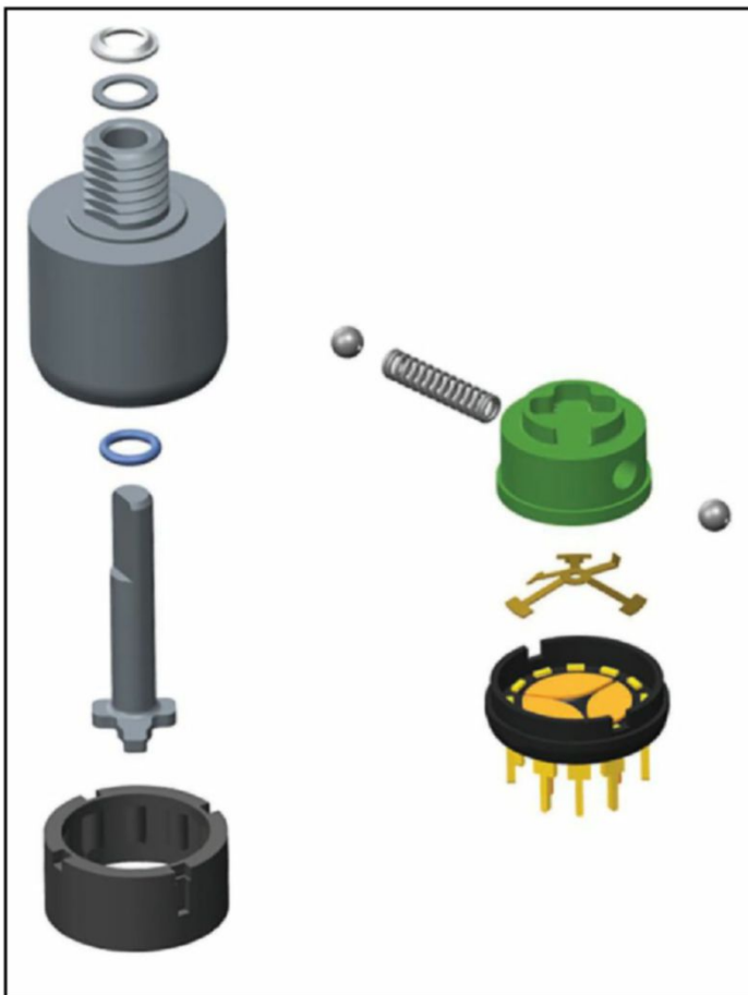
Figure 1: This exploded view shows the construction of a 16-position BCD rotary switch. The ball bearings click into fixed positions in the slots inside the tube at bottom left. (Source: Grayhill, Inc.)
