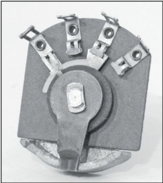
Photo 2: This conventional rotary switch has three positions. The Common terminal at left connects alternately to the other three contacts. Note the small detents in the switch’s metal frame at bottom. The springy metal attached to the center knob shaft clicks into place for each fixed position.
