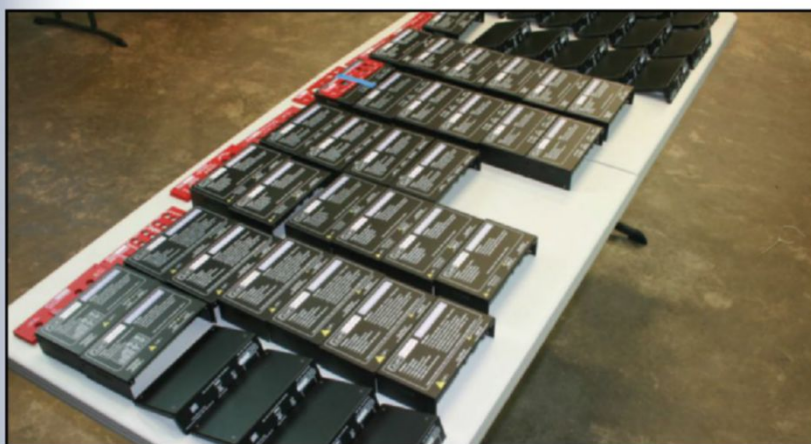
Photo 3: The QA401 panels have been fully printed and are ready for assembly with the PCBs.
