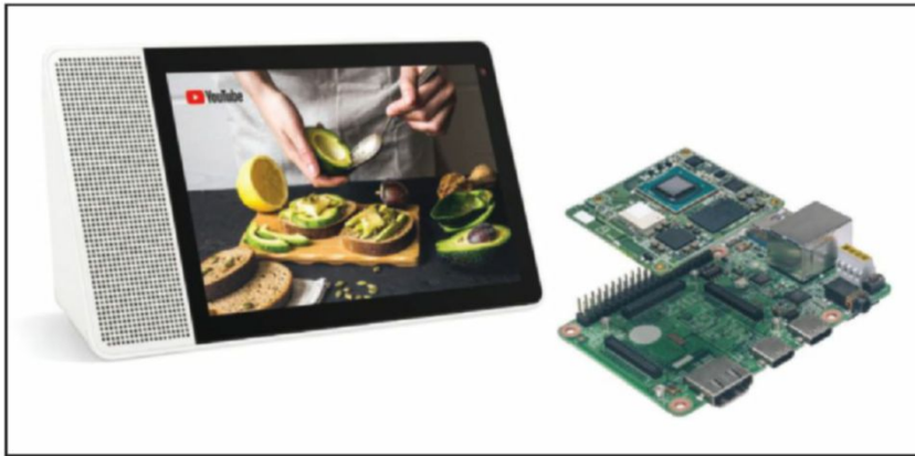
A Google Edge TPU machine-learning development kit with Google's purpose-built ASIC is designed to run inference at the edge. The type of solution used to develop applications for devices such as Smart Displays with Google Assistant.
