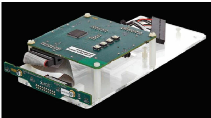
XMOS VocalFusion 2-Mic Dev Kit for Alexa Voice Services, based on the XMOS XVF3510 voice processor
