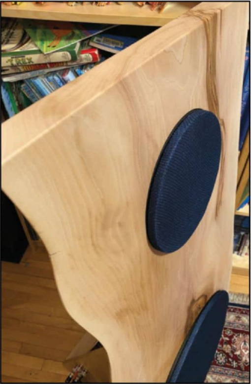
Photo 6: The flush-mount grille hoops, made on a CNC machine and wrapped with dark blue cloth, complete the design. The live-edge birch is lightly stained with lacquer spray.
