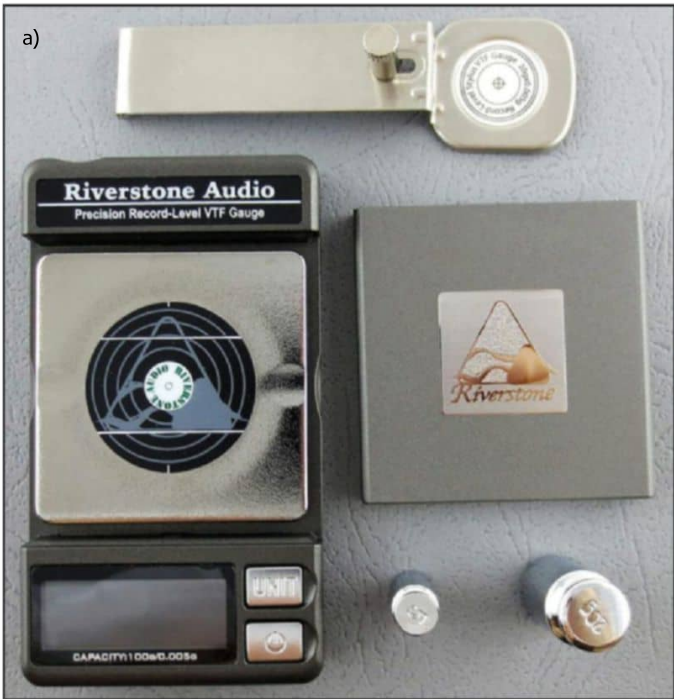
Photo 4: The Riverstone Audio RL100 comes with 5 gram and 20 gram calibration weights and a special cantilever extension arm to place the stylus at the approximate thickness of an LP record (a). The device is shown in use with the author's archival playback setup—a Stanton 500AL cartridge and 3.3 mil truncated-elliptical stylus mounted on a Jelco SA-750L tonearm. The nickel glued to the Jelco headshell adds mass necessary to achieve a tracking force of 7.0 grams for shellac 78-rpm records (b). (Source: Photo 4a, Amazon.com)
