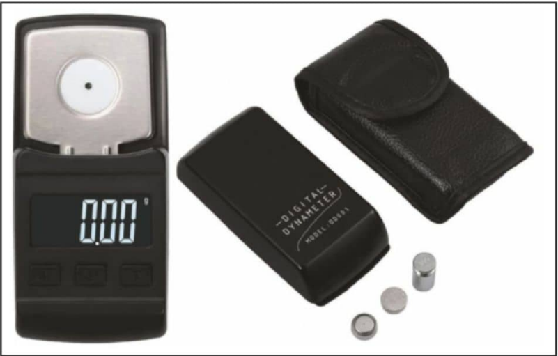
Photo 3: The newer Neoteck EMB-02 is supplied with a protective cover, a case, batteries, and a 10-gram calibration weight. The gauge will operate over a range of 0.03 grams to 100 grams. The photo on Amazon shows the previous model number, DD001. (Source: Amazon.com)
