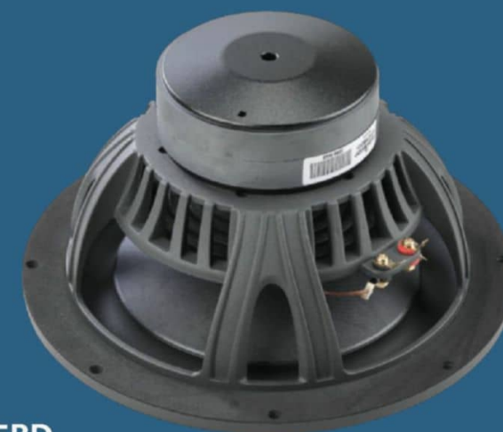
WF275BD New 10" bass driver. Usable for 2-way designs. 27 Hz resonance. 450 W long-term power handling.
