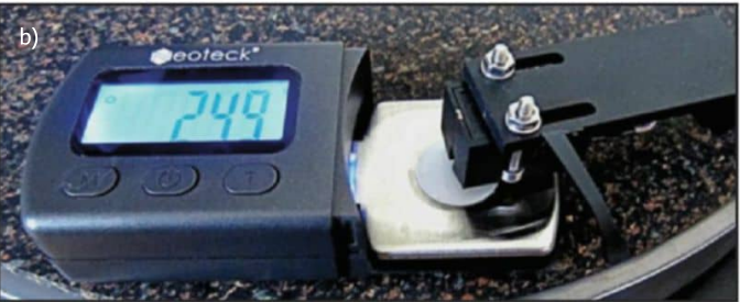
Photo 2: The Neoteck NTK002 is supplied with a case, batteries, and a 5-gram calibration weight (a). Maximum tracking force is 5.00 grams. The gauge is shown in action with the author's Jelco SA-750D tonearm and Denon DL-103R cartridge (b). (Source: Photo 2a, Amazon.com)
