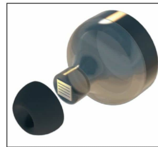
Figure 4: A commercially attractive electrostatic MEMS microspeaker should have a size of not much more than about 10mm 2 and be able to produce a sound pressure level of 120dB in the ear canal. The battery drain of the entire audio reproduction system, including the amplifier and the charge pumps providing the necessary MEMS drive voltages from a lithium polymer battery, should not exceed 3mW for typical use cases to be competitive.
