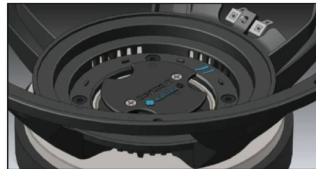
Figure 1: The Maltcross technology is a forced convection circuit at the core of the driver, helping to lower the working temperature of the coil and also acting as a demodulation ring, linearizing the inductance of the transducer.
