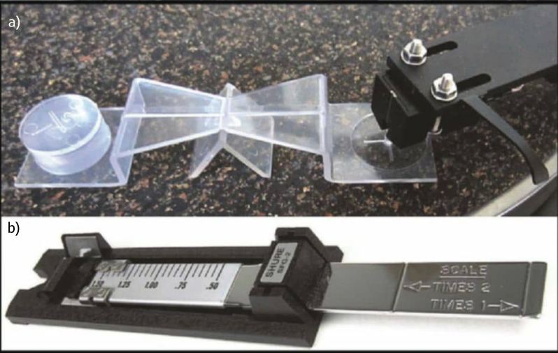
Photo 1: Here are two popular analog stylus tracking force gauges—the AR (a) and the Shure SFG2 (b). Both have been discontinued, but Esoteric Sound is selling a clone of the AR, and many online dealers have remaining stock of the Shure. (Source: Photo 1b, Shure Brothers)
