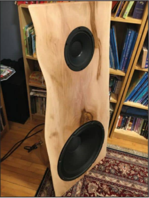
Photo 3: For speakers, I chose the Eminence Kappa Pro 18LF woofer and the 8" Radian 5208 coaxial mid bass + Constant Directivity horn tweeter.
