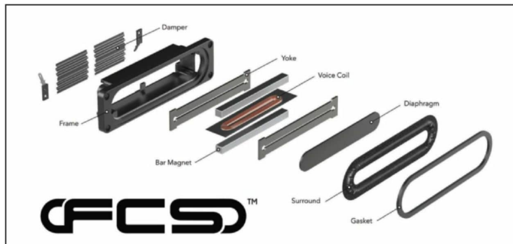
Exploded view of the Resonado Flat Core Speaker (FCS) technology, detailing the parallel bar magnet and planar voice coil array mounted perpendicularly to a flat diaphragm.
