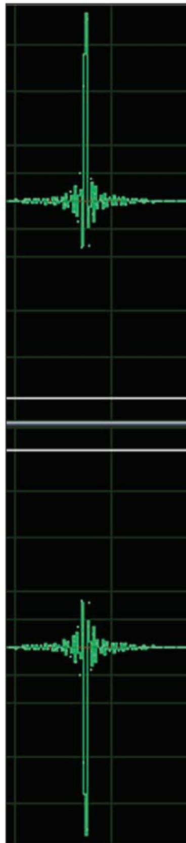
Photo 3: The out-of-phase impulses show that the speakers are wired out of phase.
