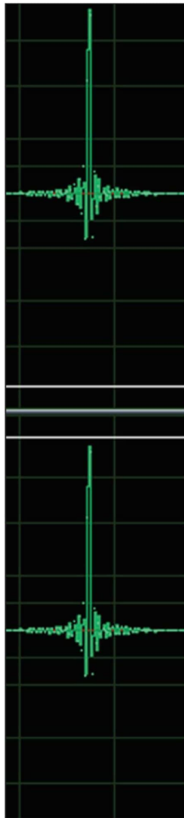
Photo 2: The impulses from the two speakers are in phase, so the speakers are wired correctly.
