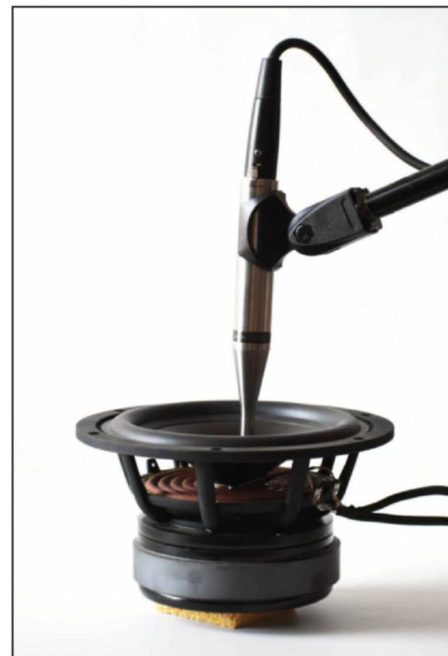
Photo 3: I use a near-field method to hit the mic with high SPL at low distortion.
