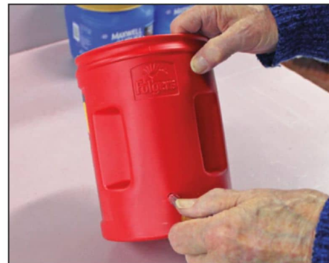
Photo 3: I used a hand reamer to enlarge the mounting holes for the parts, which I drilled first with a 1/8" bit.
