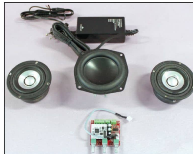
Photo 2: The main electronic parts are displayed with the woofer, two satellites speakers, the power supply, and the three-channel Bluetooth amplifier.
