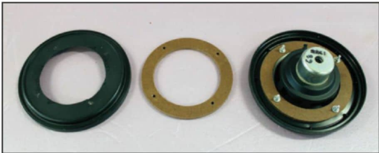
Photo 7: This image shows the modified can lid on the left with the baffle ring in the center. The completed baffle is shown on the far right. The ring is 5.5" in diameter; the hole for the woofer is 3.75", and for the satellites, 2.75".
