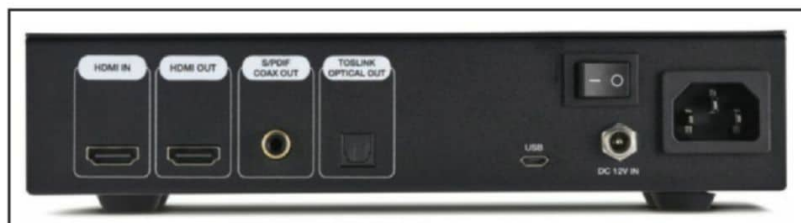
Photo 2: This is the rear panel of the D.BOB. Digital Audio connections, from left to right, include HDMI In and Out, S/PDIF Coax Out and TOSLINK Optical out. The unit can be powered from an AC power outlet using the IEC power connector on the far right, or from an external 12 VDC power supply using the DC power connector located below the power switch. (Photo courtesy of GeerFab Audio)
