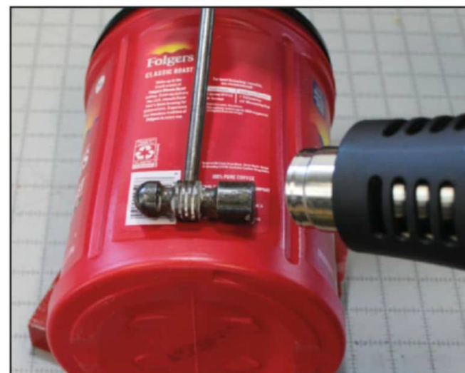
Photo 4: I used this technique to slightly flatten the bottom portion of the woofer/amplifier housing (see text).
