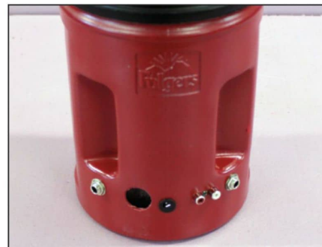
Photo 5: The handled portion of the woofer/amplifier can shows, left to right, the right satellite output jack, the 1" port, the 2.5 mm power jack, the RCA audio in jacks, and the left satellite jack.
