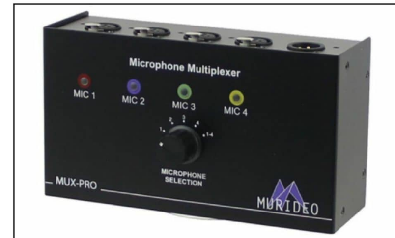
Photo 2: The Murideo microphone multiplexer allows simultaneous measurement of the frequency responses at up to four microphone locations.
