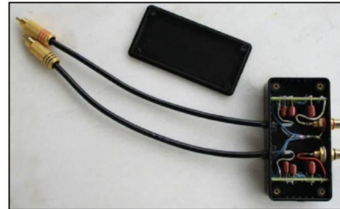
Photo 3: The internal construction of the passive equalizer
