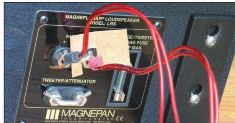
Photo 3: The input terminals are closely spaced bare metal, hence the cut paperboard. In this picture, the "tweeter attenuator" terminals and the factory iron jumper are clearly visible along with the fuse protection.
