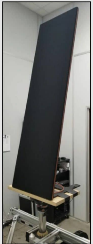
Photo 1: Magnepan's LRS is shown in its default angle for measurement using the Klippel Near-Field Scanning (NFS) system at Warkwyn's facility.
