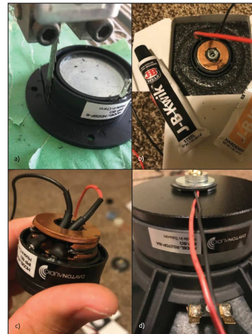
Photo 2: Construction of the tweeter assembly. a) Mounting flange is removed on the bandsaw. b) Copper washers and a nut are epoxied on. c) Washers are stacked until adequate spacing is obtained. Note the gap for the wires to be routed to the inside. d) Mounting screw and wires are routed out the rear.
