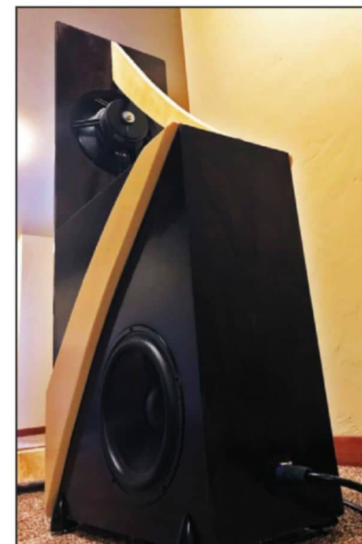
Photo 4: The back of one of the two 10" aluminum passive radiators is shown, along with the Speakon connection for the crossover and the open-baffle mid.
