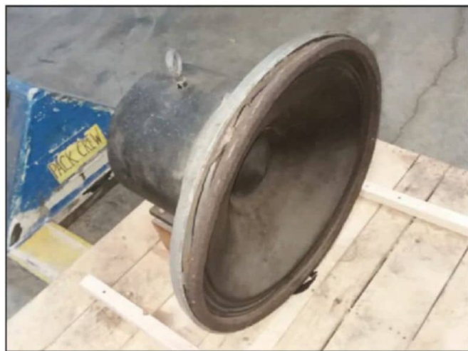
Photo 5: This huge speaker was one of eight used to drive the low-frequency double horns at the Lagoon of Nations system. (Photo courtesy of Jim Hunter, Manager of Engineering, Operations, and Resident Historian of the Klipsch Museum of Audio History)
