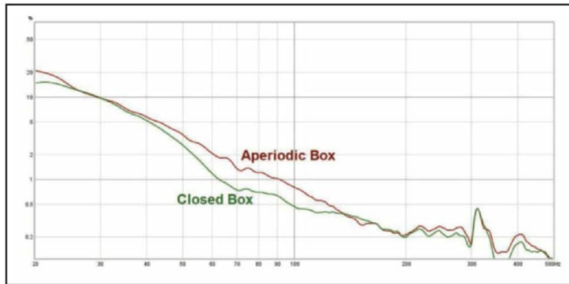
Figure 10: Distortion measurements at the low frequencies
