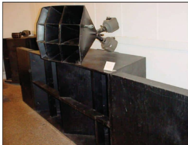
Photo 4: This is a copy of the original Shearer horn: two W boxes with 15" drivers topped by a multicellular high-frequency horn with RCA compression drivers. (Photo courtesy of Jim Hunter, Manager of Engineering, Operations, and Resident Historian of the Klipsch Museum of Audio History)
