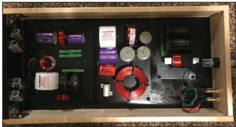
Photo 5: The crossover was constructed using a separate board for each driver. Zister resistors were mounted to the front heatsink for the higher dissipation positions. I used XSim to calculate how much power each resistor will potentially need to dissipate as heat.
