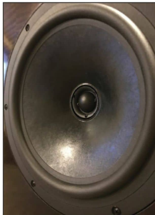
Photo 3: This is a close-up image of DIY coaxial driver constructed from a Dayton RS270P and a ND28.
