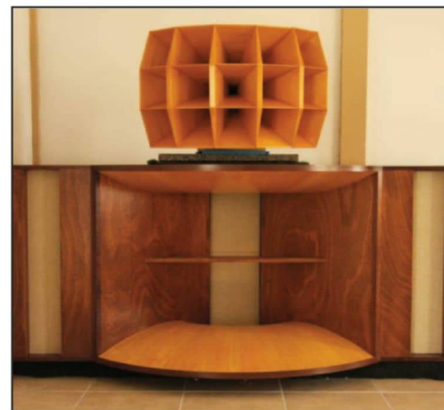
Photo 7: This RCA MI9462 bass horn is shown with an Altec 1503 multicellular high-frequency horn.
