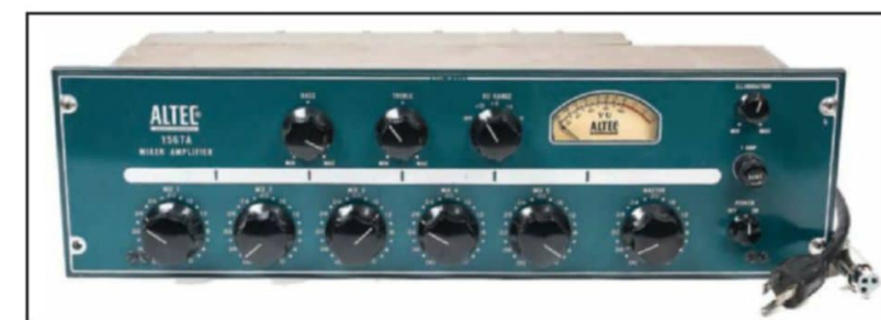
Photo 6: The Altec-Lansing 1567A was a small portable hollow-state mixer that was quickly adopted for all sorts of venues.
