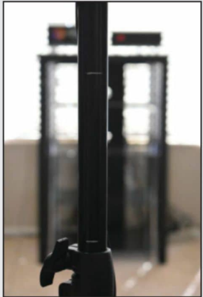
Photo 2: Putting marks on the tripod shaft enables consistent and repeatable changes in mic height for the Dirac measurements.
