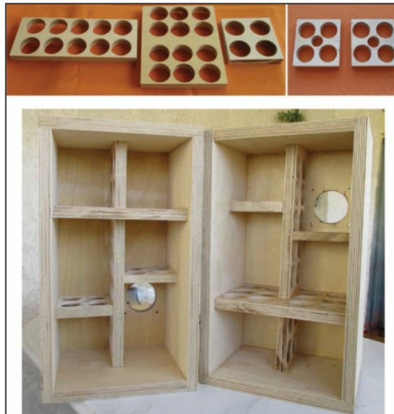
Photo 5: The internal braces of the box
