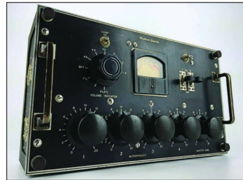
Photo 3: This Western Electric Model 22C "portable" four-channel mixer was designed for broadcast and sound-reinforcement use with speech signals.
