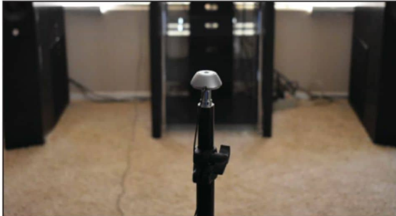
Photo 3: A measurement microphone with a calibration file is included with the M10 to set up Dirac. It mounts on any photographic tripod and points upward.
