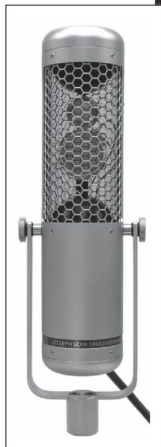
Photo 2: This is the Josephson C700S stereo microphone. This unusual stereo mic contains three condenser capsules and can be used for a variety of single-point stereo techniques, including Blumlein, X-Y, and M-S. (Photo courtesy of Josephson Engineering)
