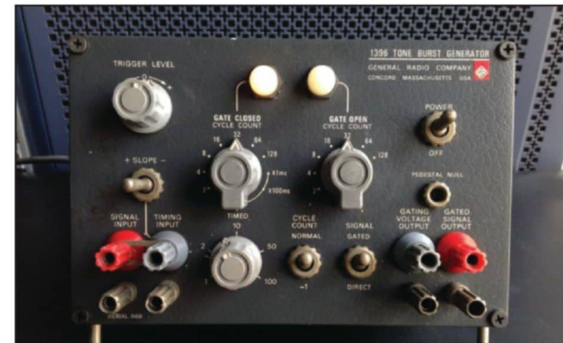
Photo 2: The General Radio 1396-A Tone burst generator is actually a gating device that allows various repeating signals to be transmitted for different periods of time.
