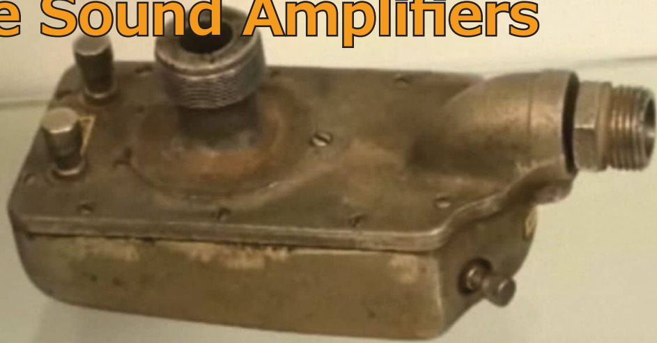
Photo 1: This Vocal Air modulated airstream driver, similar to the one used by Gaumont in 1900, is capable of producing the loudest amplified sound of any speaker even today. (Photo courtesy of Jim Hunter, Manager of Engineering, Operations, and Resident Historian of the Klipsch Museum of Audio History in Hope, AK.)
