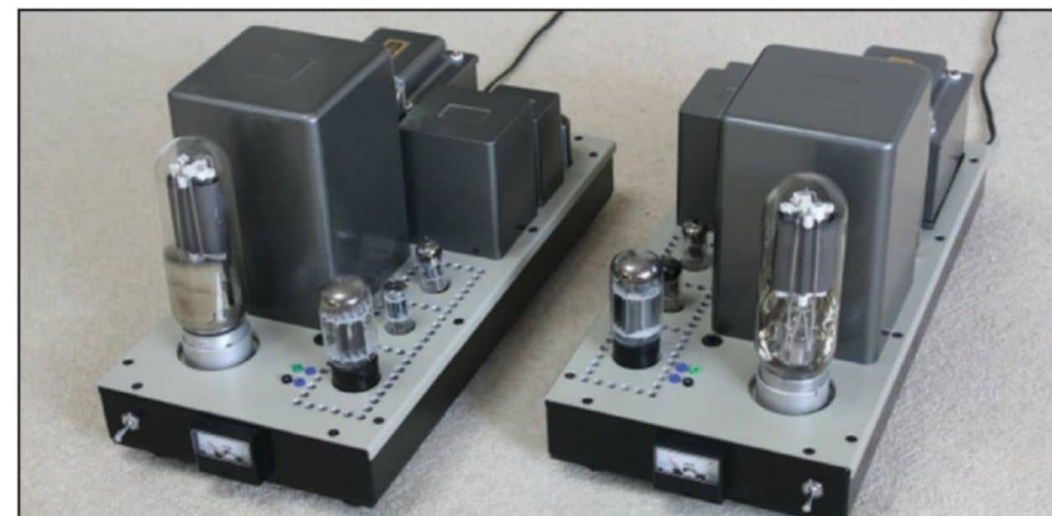
Photo 6: These left- and right-channel single-ended audio power amplifiers illustrate the use of the 838 tube, and show its size in comparison with a 5998 driver triode and miniature dual triodes 12AT7 and 12BH7. (Photo courtesy of Michimori Hirokuni)
