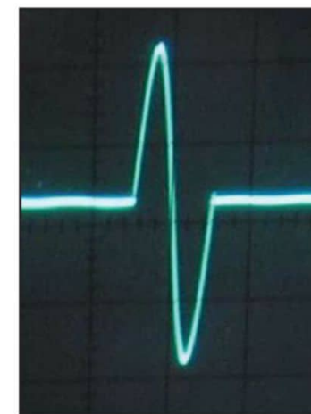
Photo 3: This is one cycle of a gated 400 Hz sine wave.
