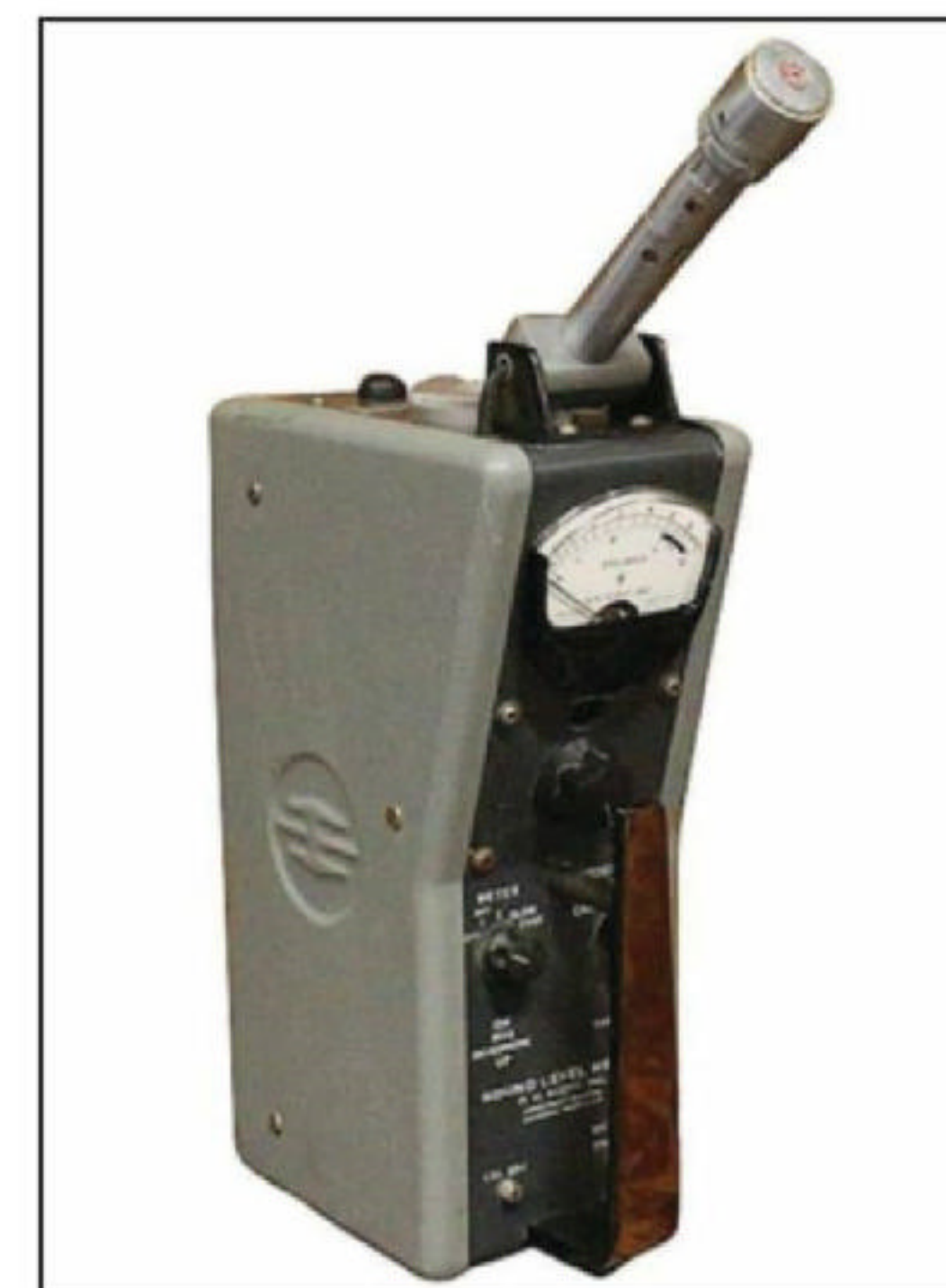
Photo 3: This H. H. Scott sound level meter used jelly-bean-sized triodes.
