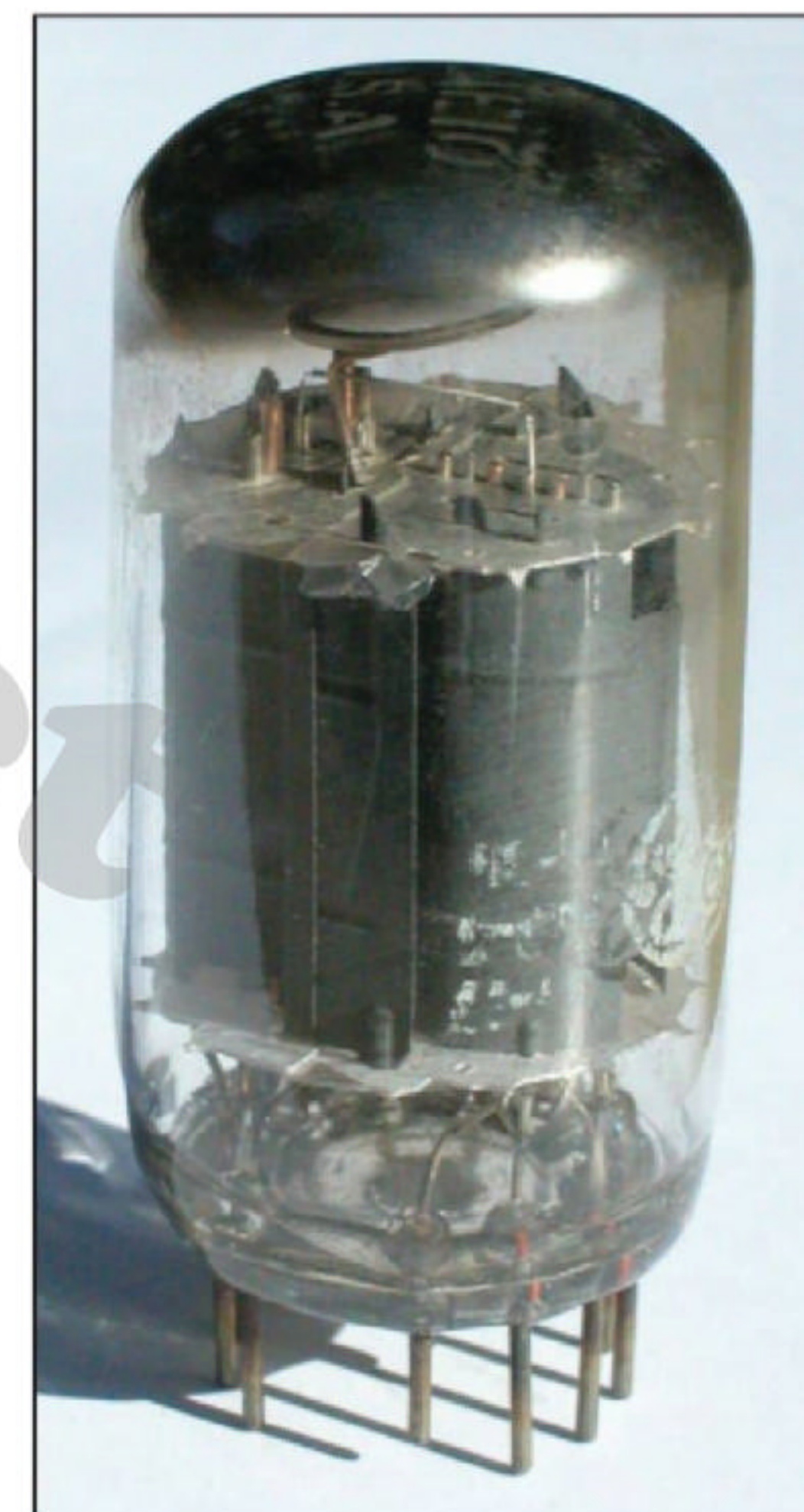
Photo 4: The Compactron achieved miniaturization by combining multiple tube functions within a single envelope.
