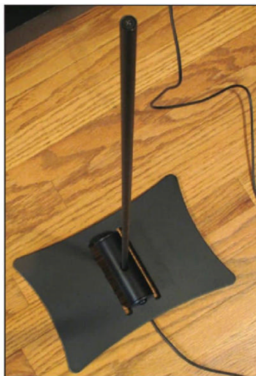
The room calibration process is essential to adapt the sound to the specifics of a living room. The supplied wand-mounted probe mic’s hinged base makes it easy to position at ear level.
