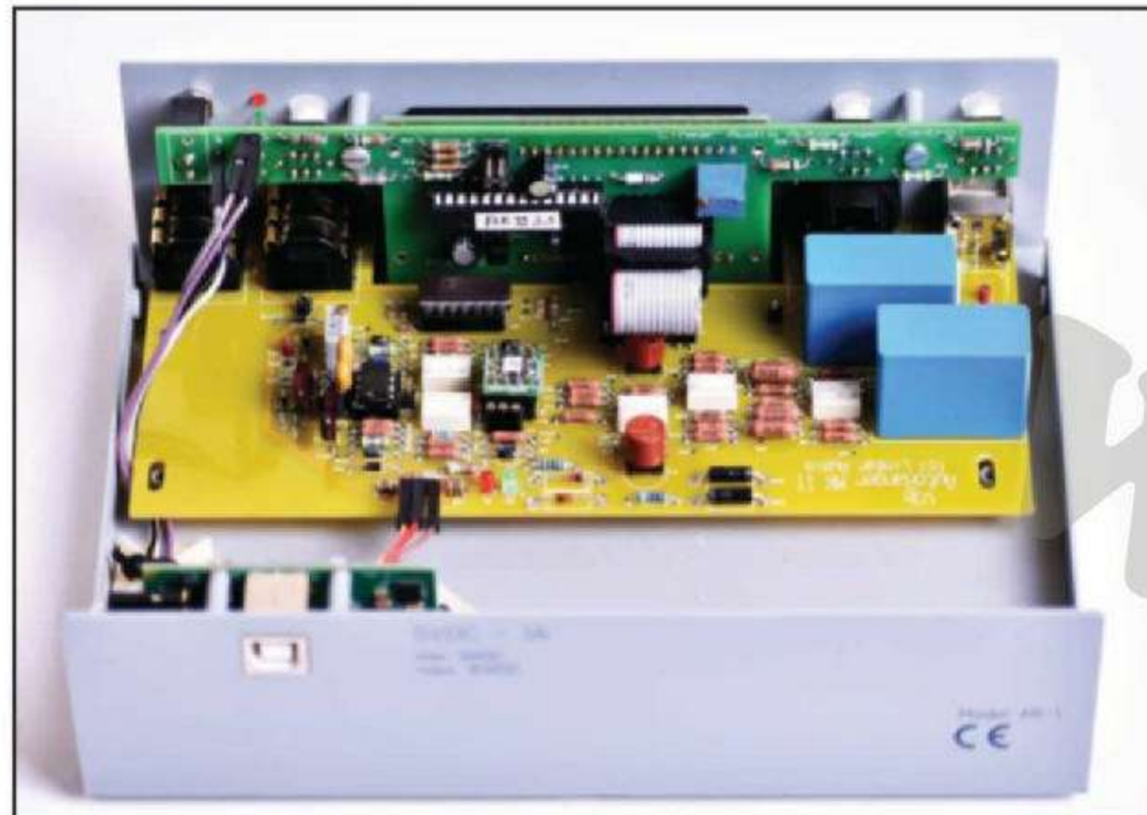
Photo 2: The interface comprises three circuit boards, which separately accommodate display/logic, analog signal circuits, and the SilentSwitcher power supply.
