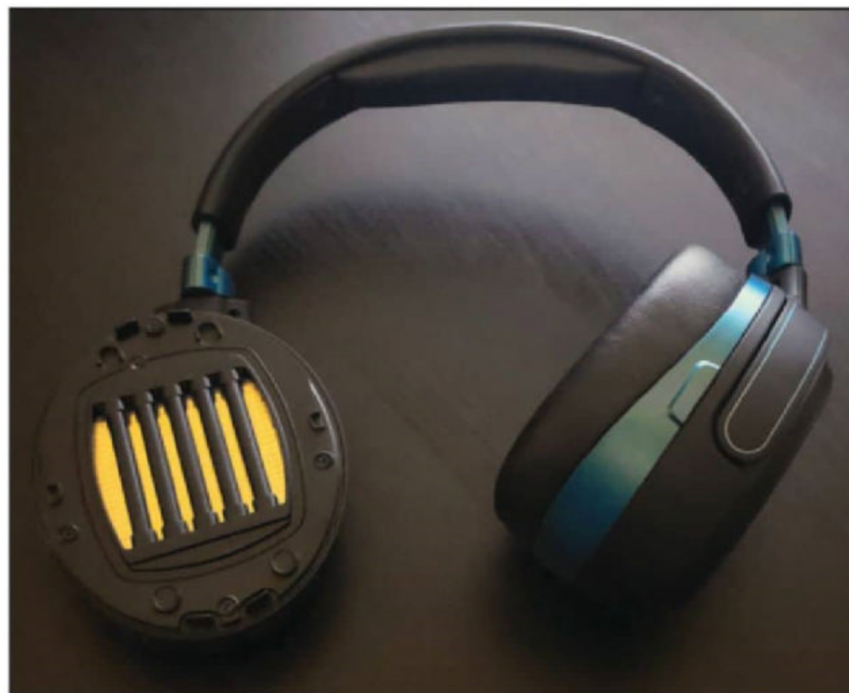
Photo 3: Each Mobius earcup features a single 100 mm planar magnetic driver, relying on DSP to virtualize surround sound.
