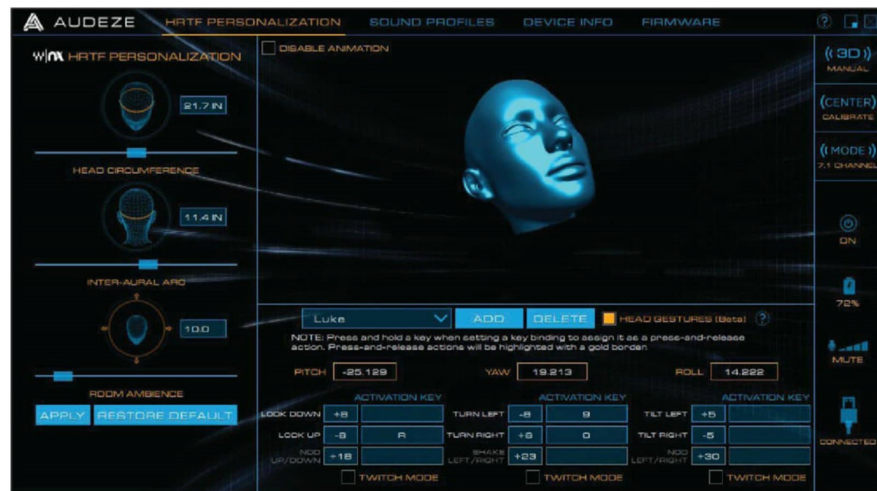
Figure 2: AudezeHQ, a desktop application, supports setup and options for the Mobius. The animated head's angle is updated in real-time by head-tracking. HRTF settings are on the left.
