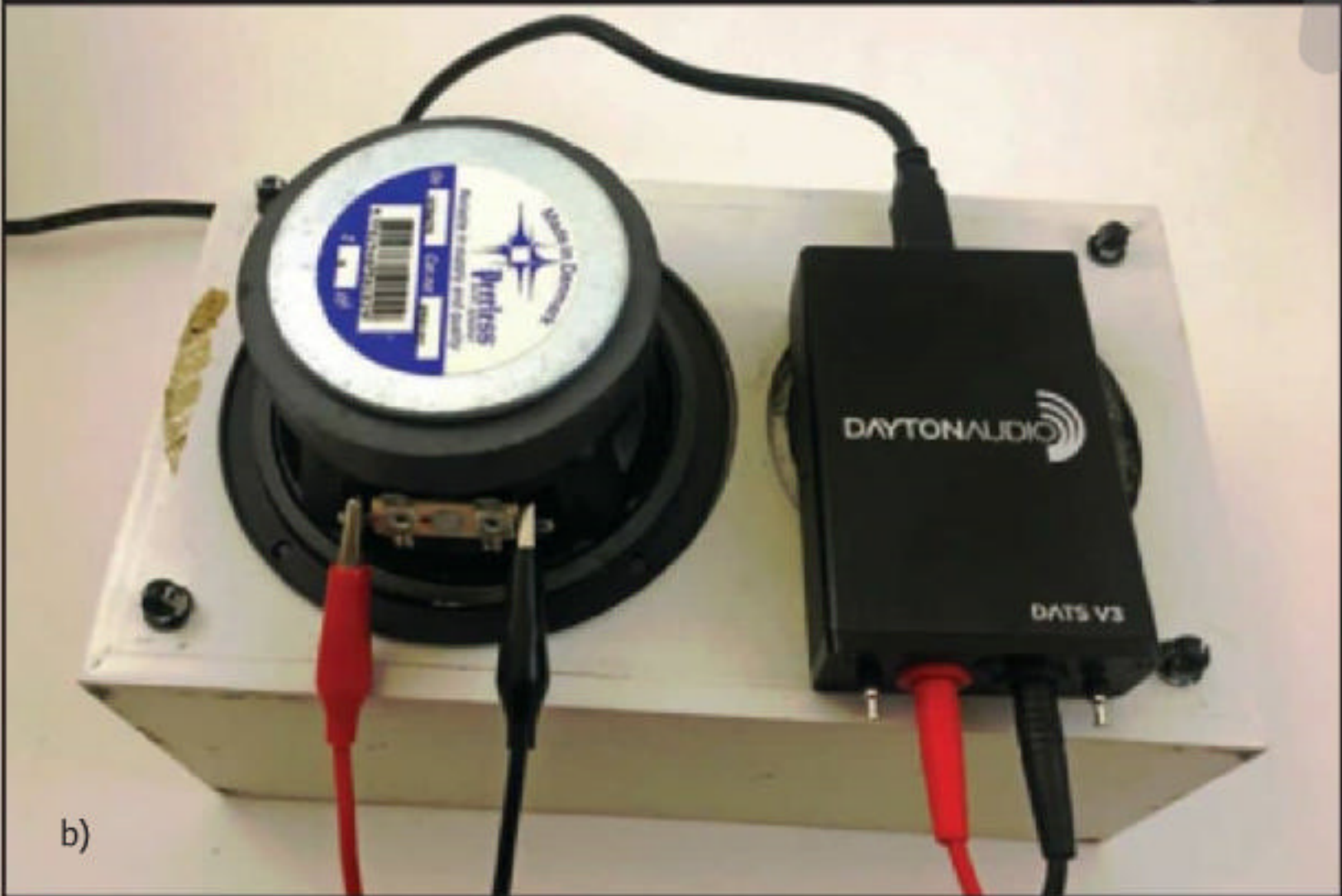
Photo 4: The DUT is tested using the Vas Added Mass method (a) and the DUT is tested using the Vas Test Box method (b).
