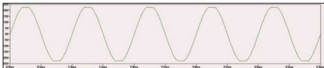
Figure 2: The power amp produced this output wave into a 16-Ω load.
