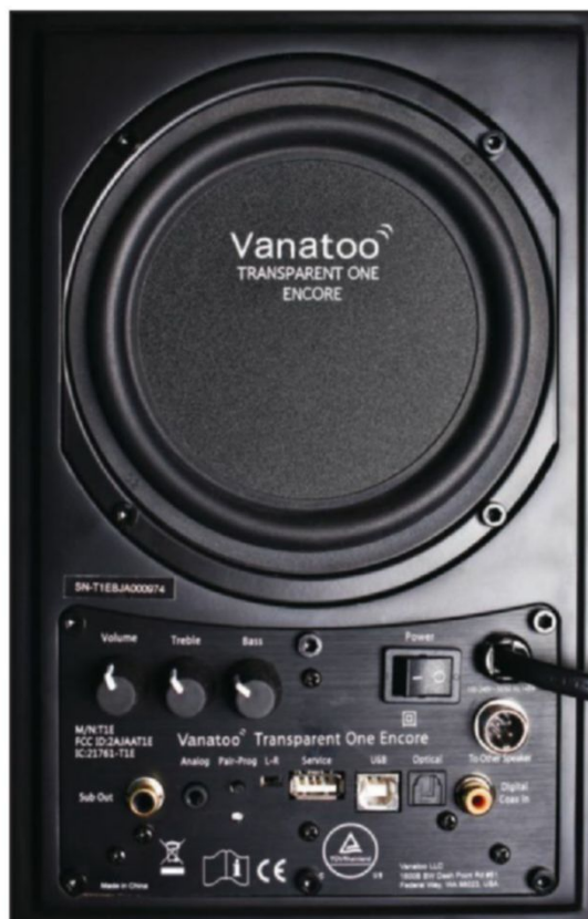
Photo 3: The back panel sports a passive radiator, an array of input options, and basic tone and volume controls.
