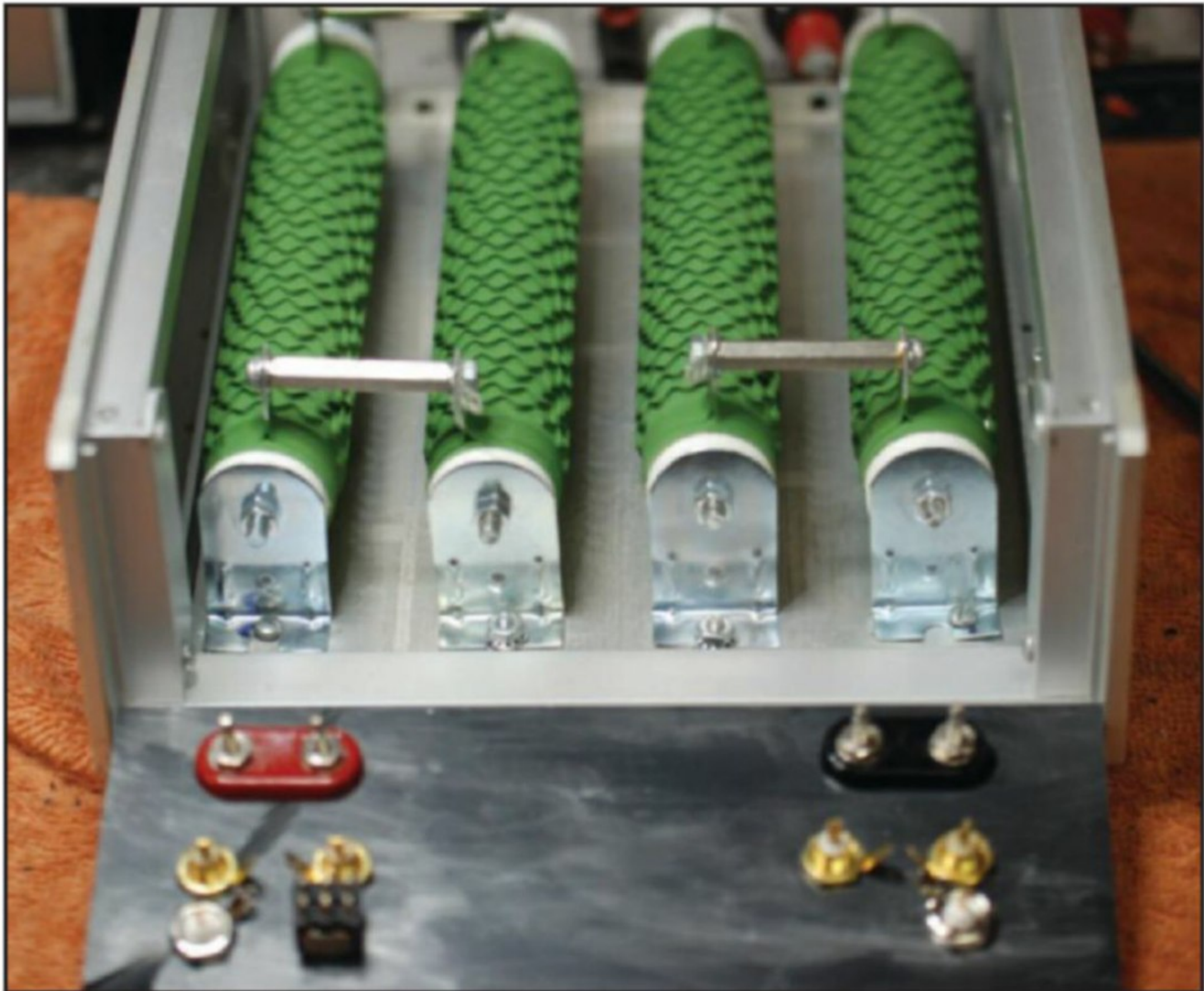
Photo 2: You can choose whatever you want for a case, but be sure you have enough space to keep the resistors away from each other so they can get adequate circulation.
