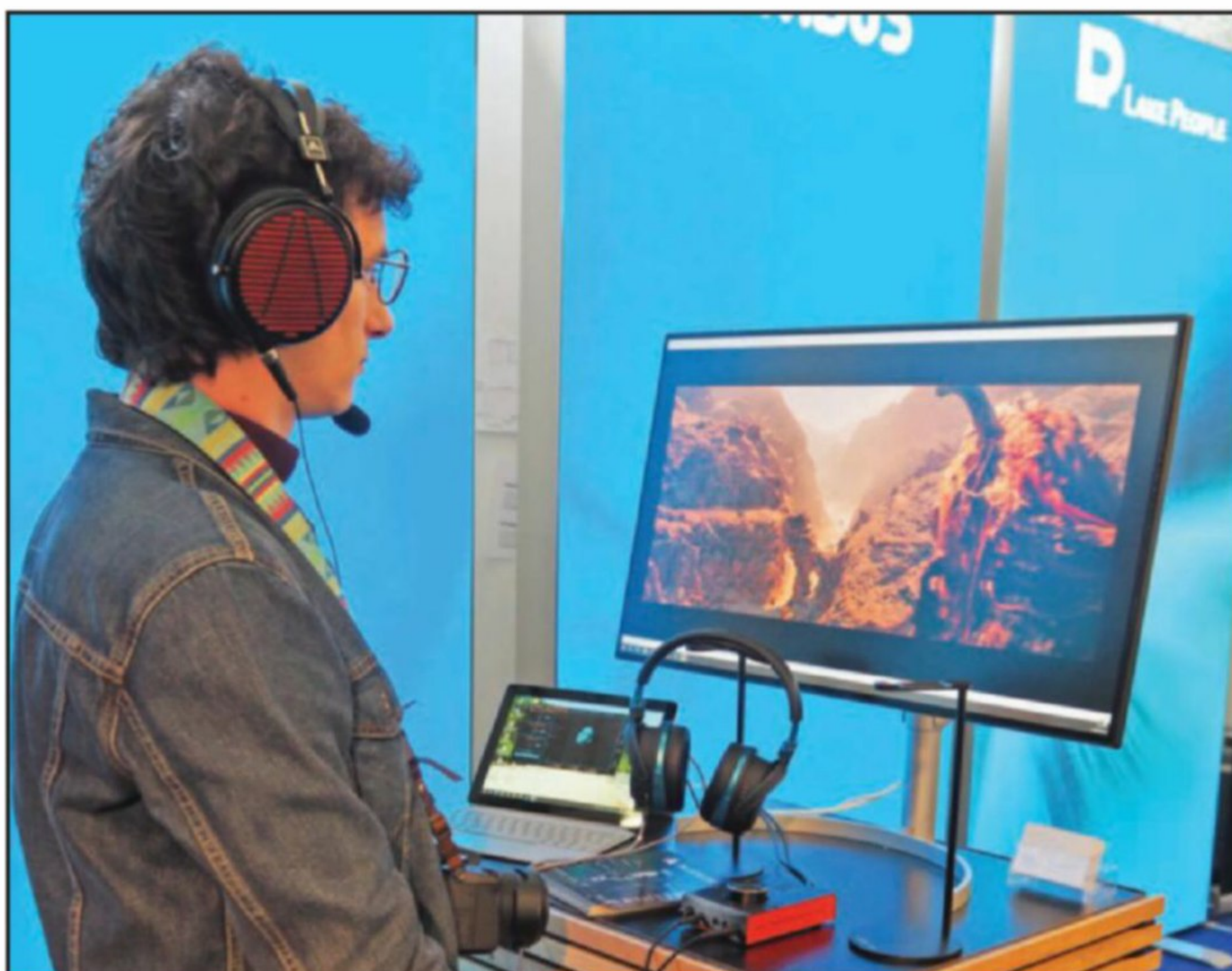
Targeting high-end gaming, the Audeze LCD-GX headphones use Audeze's gigantic Fluxor magnets and Uniforce diaphragms and a detachable microphone.
