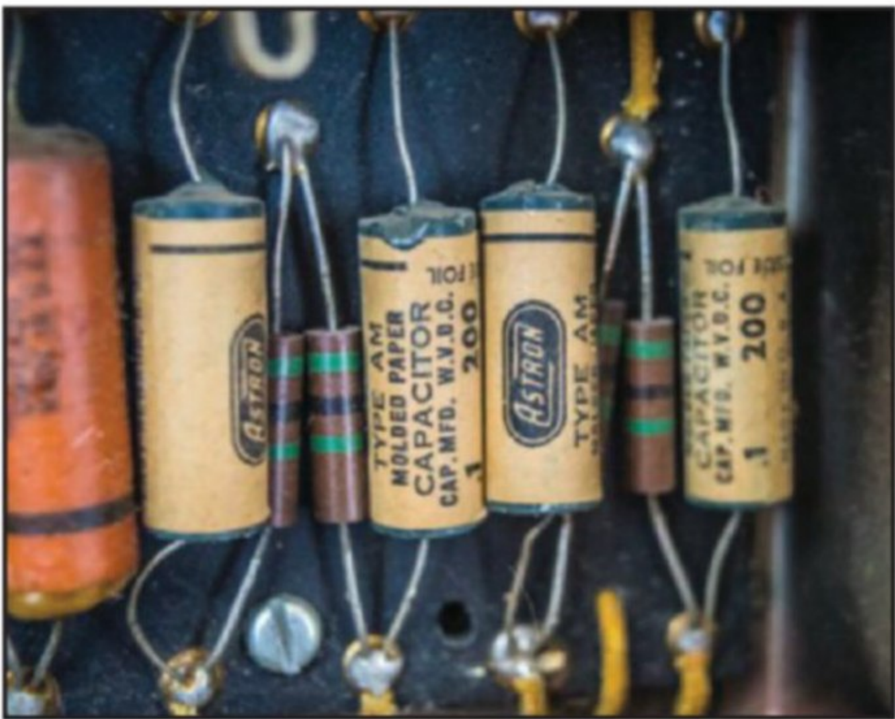
Photo 4: Here are four tubular molded paper-oil capacitors and at the far left of the image, a wax-paper capacitor.
