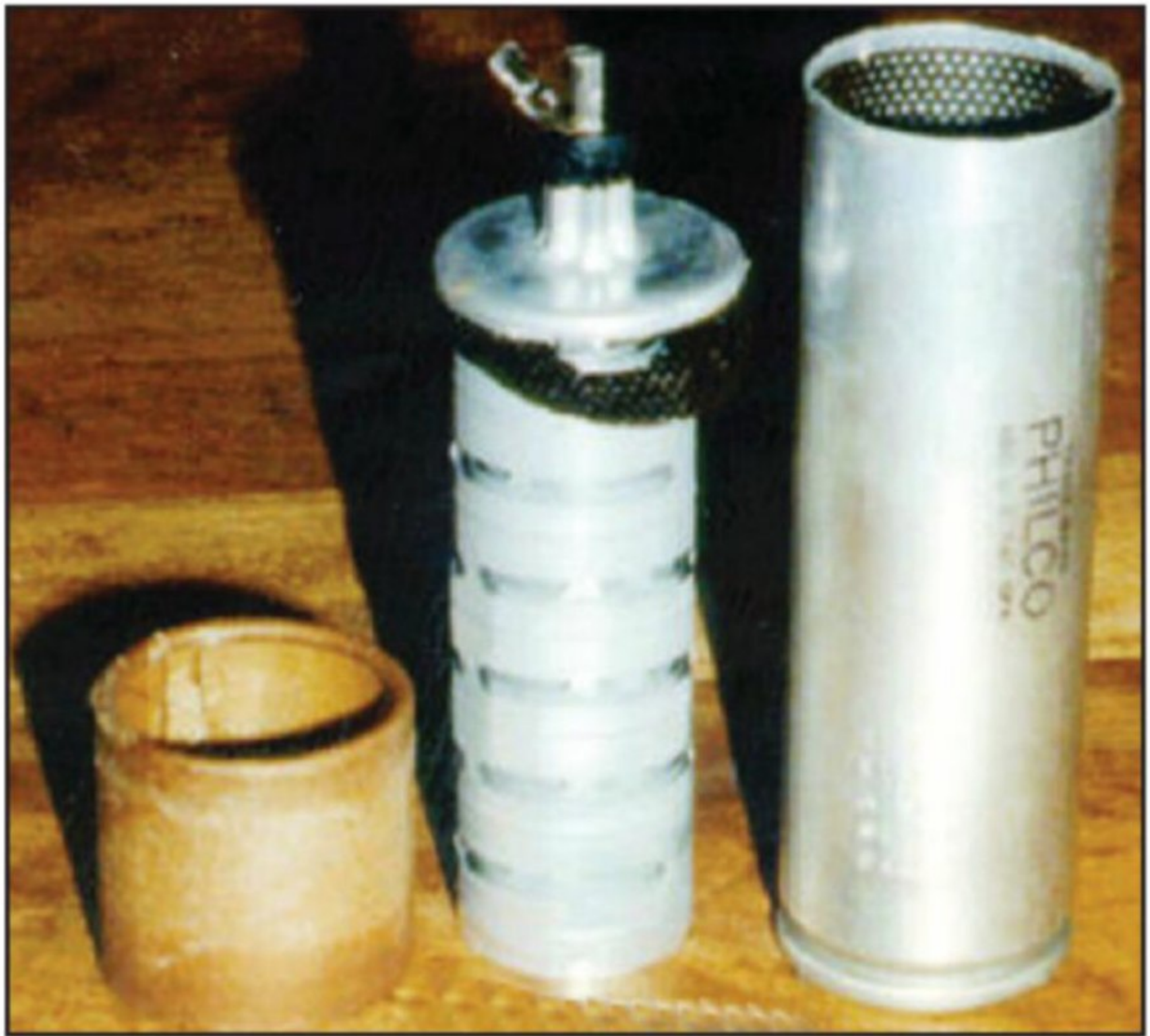
Photo 6: The parts of a disassembled wet electrolytic cap include: at left, a cardboard spacer; in the center, the loosely coiled positive plate; and at right, the can that serves as the negative plate.
