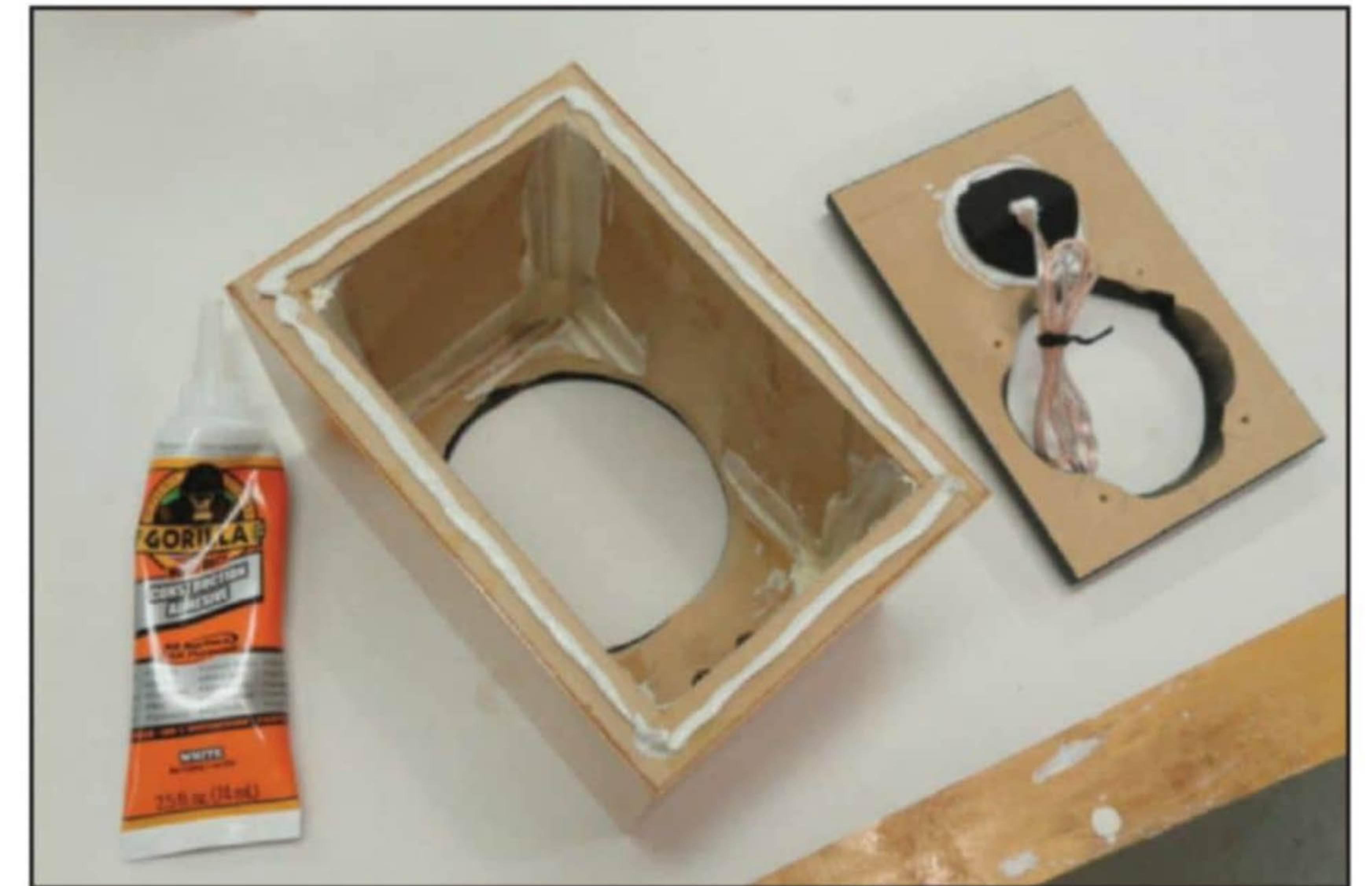
Photo 9: Construction adhesive was applied to the front end-grain of the cabinet. I wiped off any squeeze-out with a damp rag immediately.
