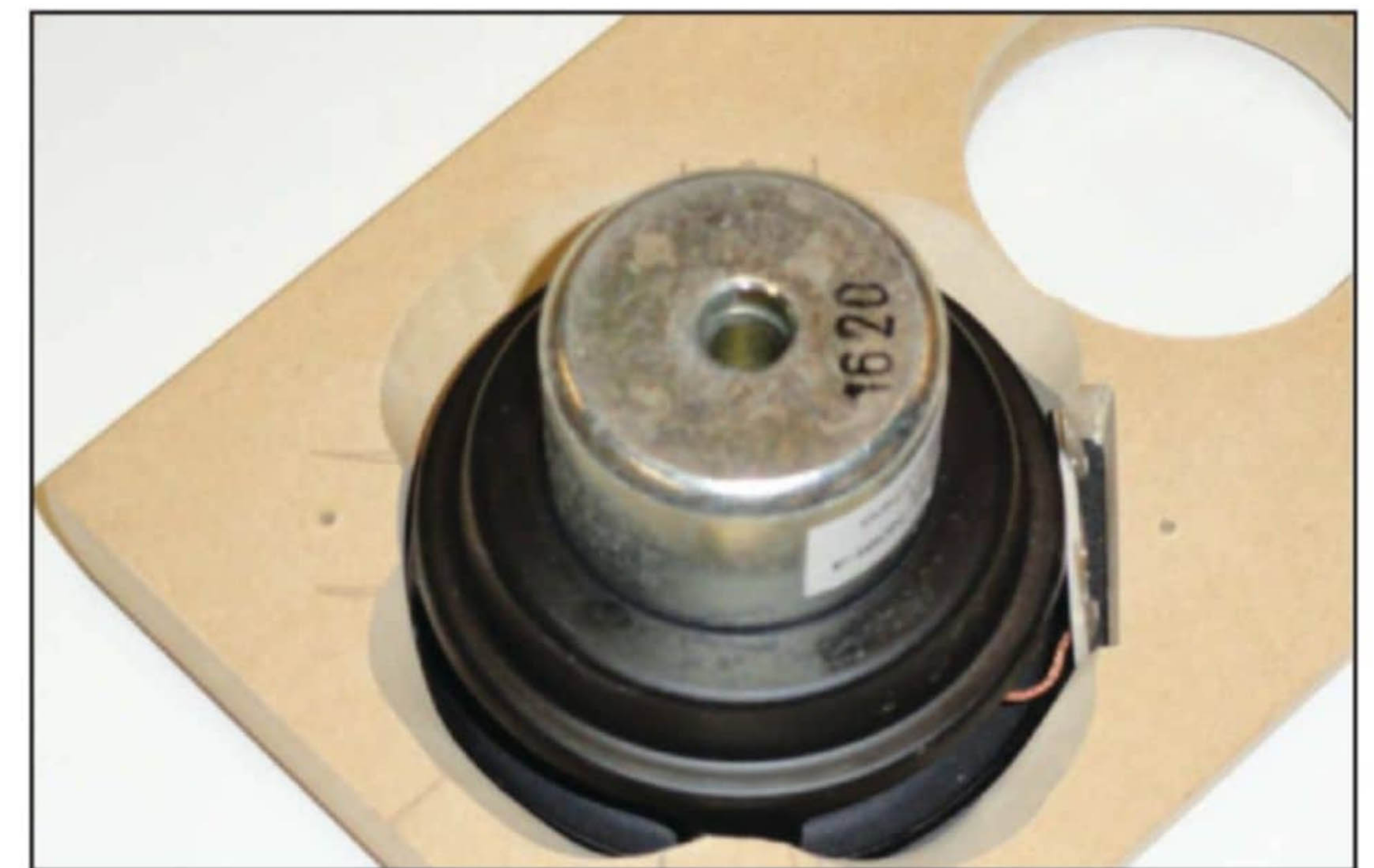
Photo 4: Driver openings are machined. The woofer opening needs a notch to make clearance for the terminal. I created scallops on the rear of the baffle to allow for proper air flow around the rear of the driver.
