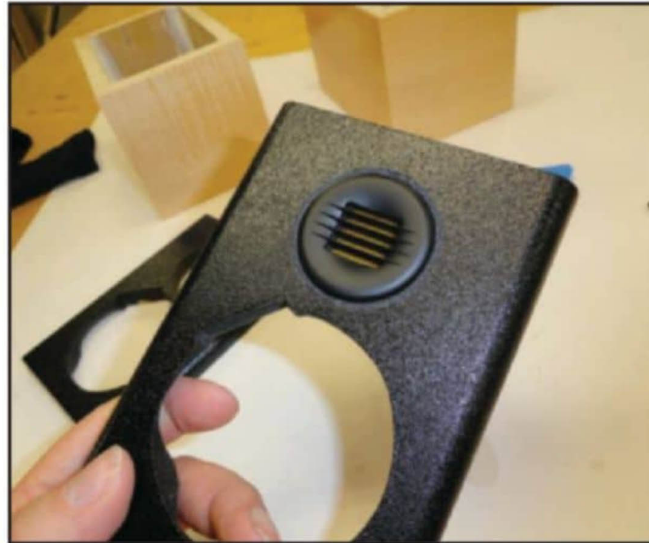
Photo 8: The baffle was painted with Rustoleum textured paint, then shot with rattle-can gloss black. Tweeter pressed in place on the finished baffle.
