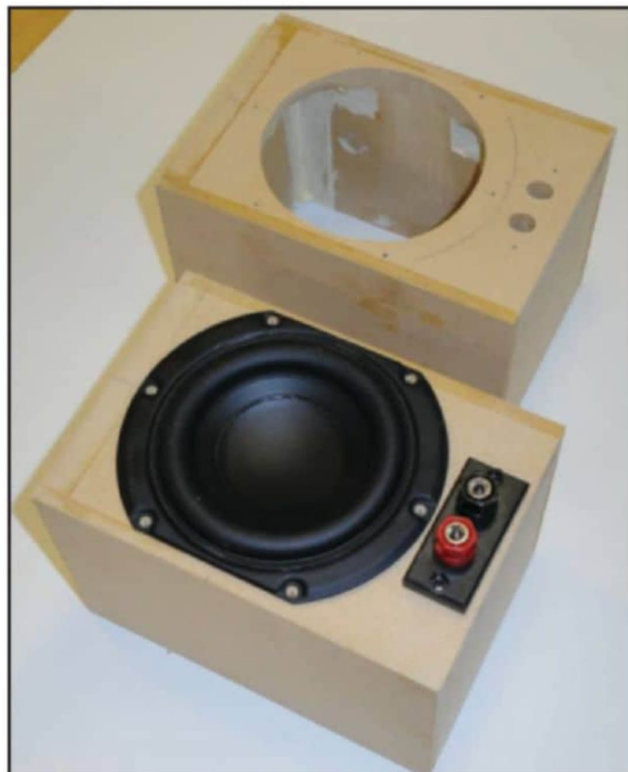
Photo 5: I cut out the opening for the passive radiator. Note the “wings” on either side of the resulting disc, which are actually thin slices of the cabinet walls.
