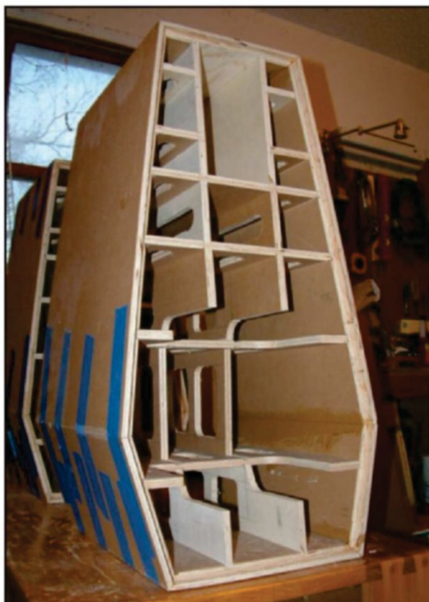
Photo 3: The front panel is placed within the dado as it is folded to ensure a square result.
