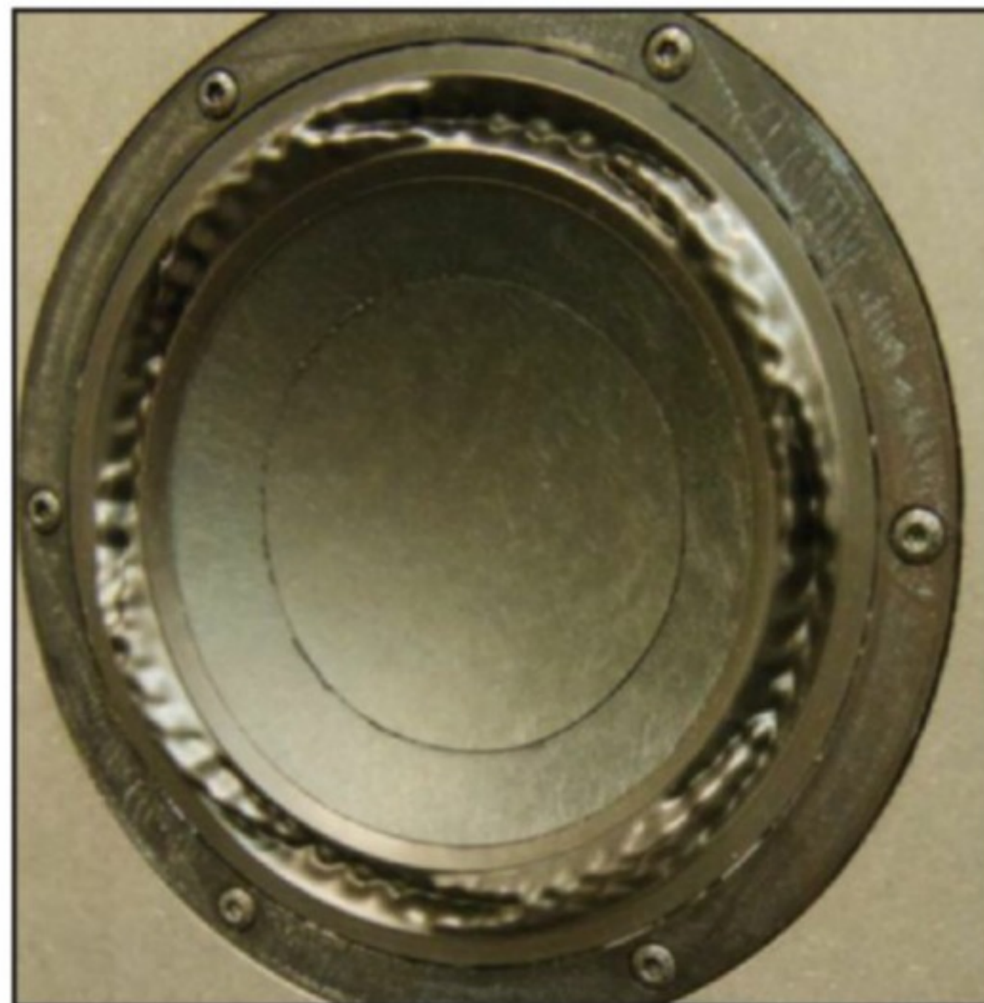
Photo 3: The new surround decreases the change of effective radiated surface with excursion, further decreasing the driver distortion.
