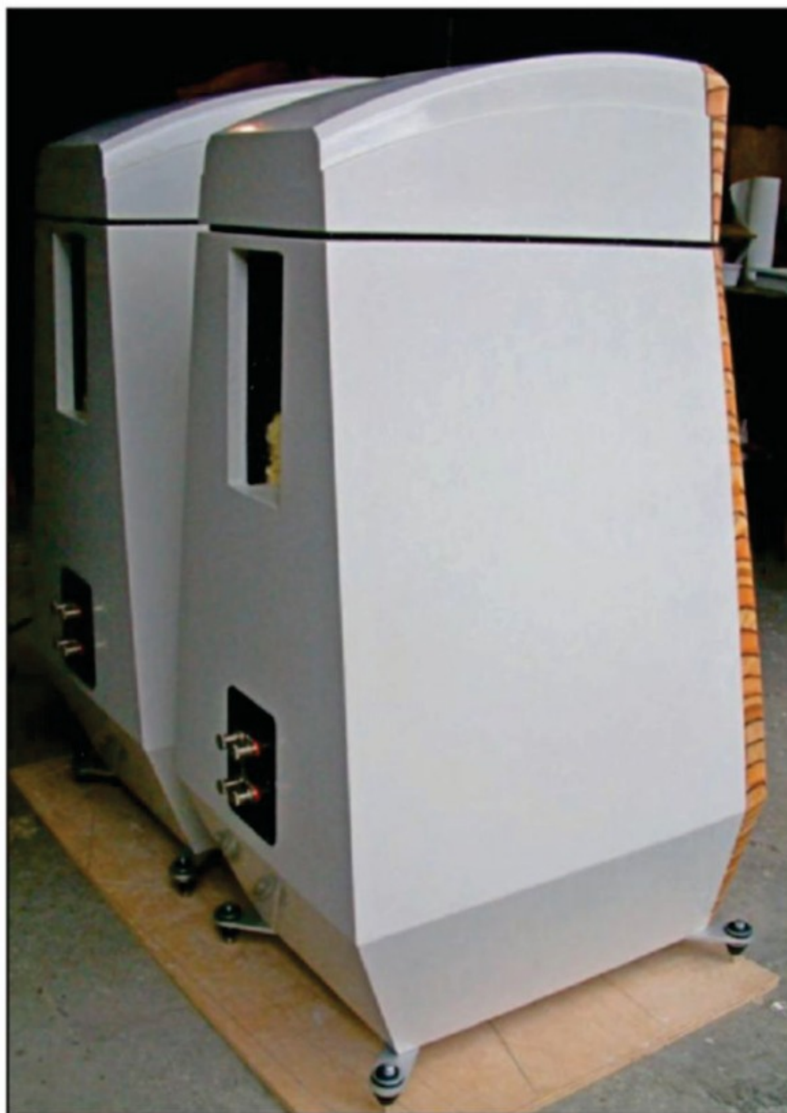
Photo 5: The tweeter box is held in place over the woofer/mid box using cap head screws and threaded inserts, with the screws accessible from inside the midranges tube.
