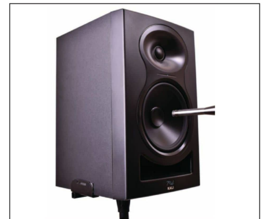
Photo 5: Near-field measurement of the Kali Audio LP-6 Studio Monitor shows excellent bass extension and quality.
