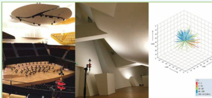
Examples of measurements made with the IRIS system by Marshall Day Acoustics for the Philharmonie de Paris acoustic design project. (Images courtesy of Marshall Day Acoustics)
