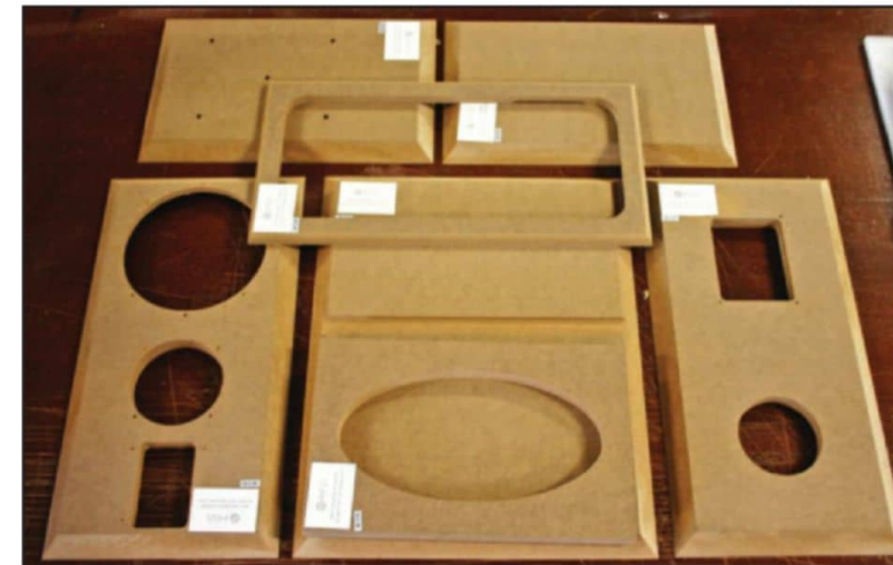
Photo 5: The pre-cut MDF panels are laid out for assembly.
