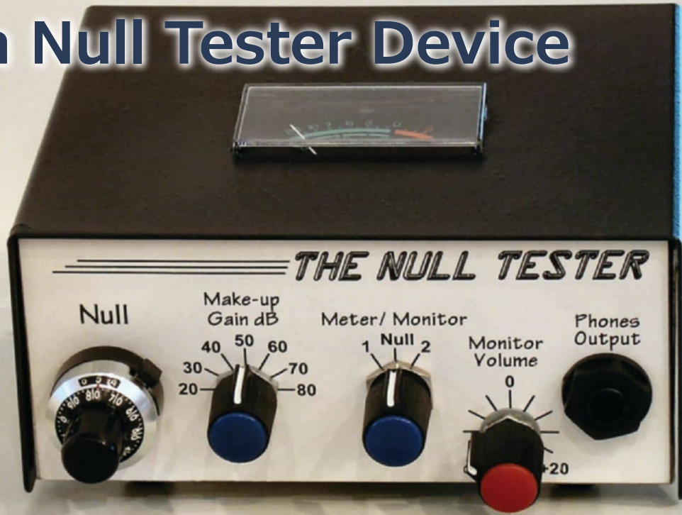
Photo 1: The Null Tester is self-contained and compact thanks in large part to the use of surface-mounted devices (SMDs). The rear panel accepts inputs from XLR, 1/4" phone, and RCA phono plugs.
