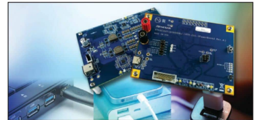
Renesas Electronics recently announced two new reference designs that simplify and speed the development of USB Power Delivery (PD3.0) and USB-C battery charging applications. The RTK-251-1PowerBank3 and RTK-251-BuckBoostConverter2 are USB-IF PD3.0 certified design kits, and represent the first in a new series of reference designs for applications implementing the USB Type-C power and data connection standard.
