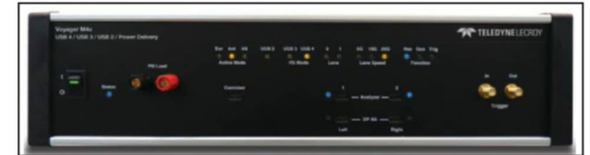
A vast set of protocol analyzers and compliance test systems are available for USB 3.2, Power Delivery, and USB Type-C from companies such as Keysight, Ellisys, Granite River Labs, and Teledyne LeCroy. Pictured above is the Teledyne LeCroy Voyager M4x Protocol Analyzer platform for testing next-generation USB4 and Thunderbolt 3 systems.
