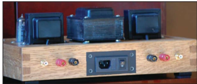
Photo 3: The rear view of the amplifier shows input, output, and power connections.
