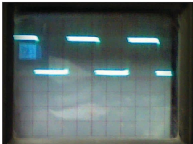
Figure 5: A test square wave produced by an Eico 390 signal generator
