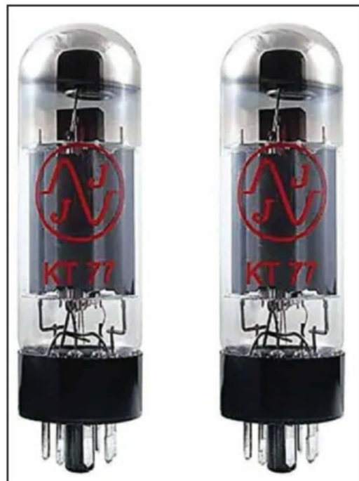
Photo 1: This is the JJ Electronic KT77, which is a beam power pentode with an octal base. According to JJ Electric, it can be used in most EL34 amplifiers.
