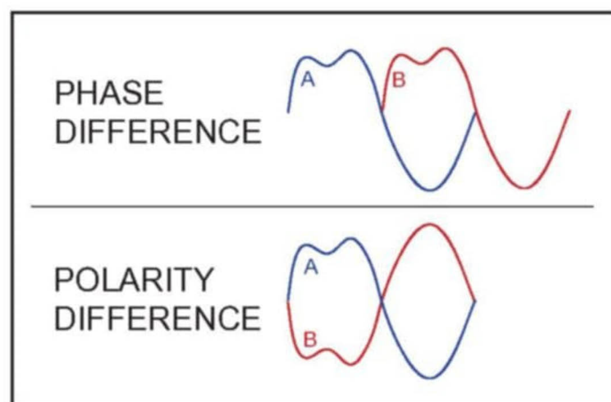
Figure 1: The difference between phase and polarity is best illustrated using asymmetrical waveforms. The upper illustration shows a phase difference—waveform B lags waveform A by 180°. The two waveforms in the bottom illustration are of opposite polarity.
