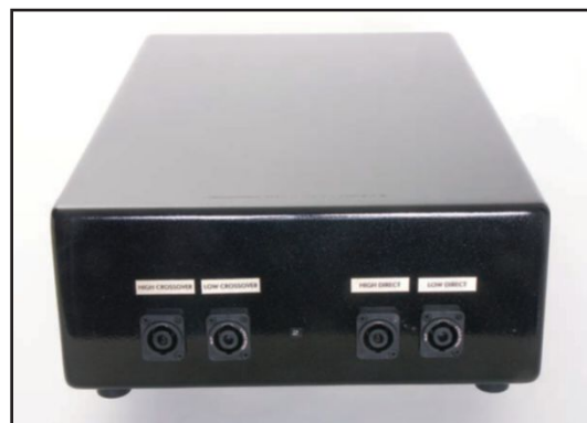
Photo 11: Speaker connections on the rear of the crossover
