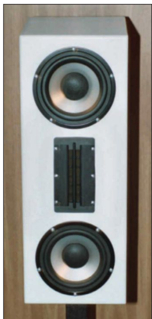
Another speaker built by Ron, which he described as: This model TSMD1 speaker is half of a stereo pair. The closed box measures 23.75" tall by 9" wide by 12" deep. Construction is 3/4" thick MDF for sides, top, bottom, and back with a 3/4" thick 13-ply birch plywood front panel. The drivers include a pair of Dayton Audio #295-337 7" aluminum woofers and a single Dayton pt2 planar tweeter crossed over at 3 kHz with a passive second-order Linkwitz-Riley network. Response is flat to within 3 dB from 100 Hz to 20 kHz.
