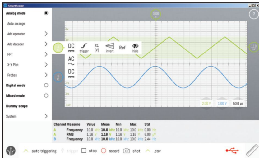
Figure 3: For each input channel you can specify AC or DC coupling, trigger direction (up, down, or both), probe sensitivity, and other parameters.
