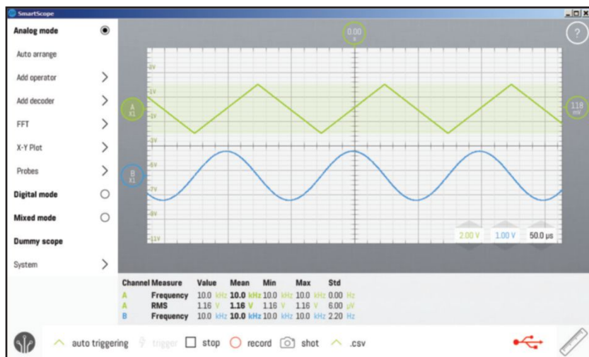
Figure 1: The bold legends at left in the SmartScope software expand to show the various options within each section.
