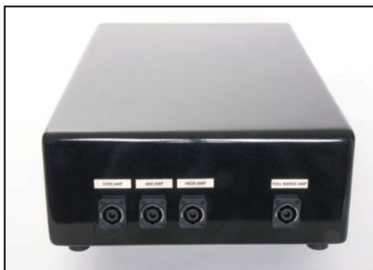
Photo 10: Amplifier inputs on the front of the crossover
