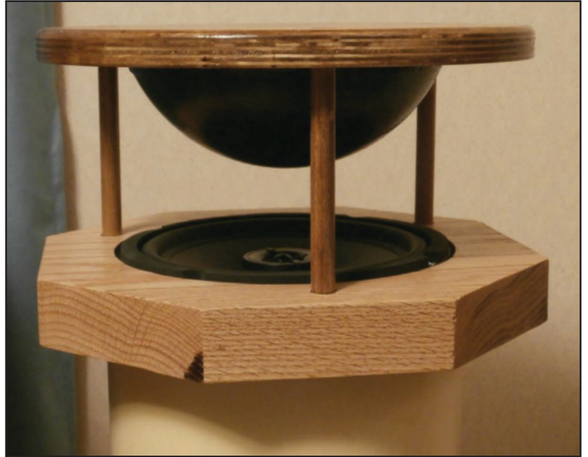
Photo 2: The top, top plate is an 11-1/2" disc of 13-ply Baltic Birch plywood stained golden oak. The black hemispheres are Styrofoam sound reflectors. The wooden dowel spacers are glued to the plywood disc and just set in the slightly oversize holes in the oak top.
