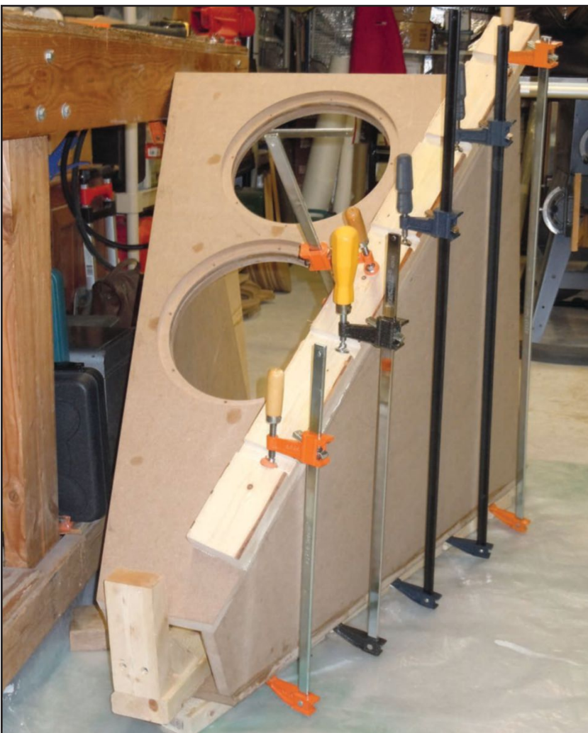
Photo 20: I clamped the fixtures to assemble the pyramid sides.
