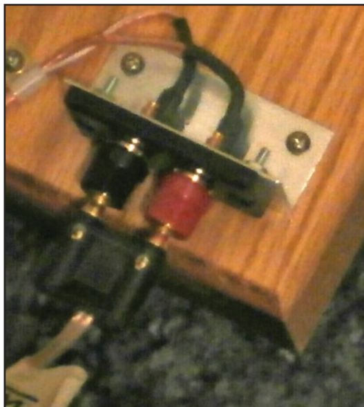
Photo 8: The twin alligator socket connects the omni-pipe to the power amplifier. The two conductor wire routes over the edge and through the 1/2" hole and through the fiber-fill up to the speaker. As a final operation, I caulked the 1/2" hole.
