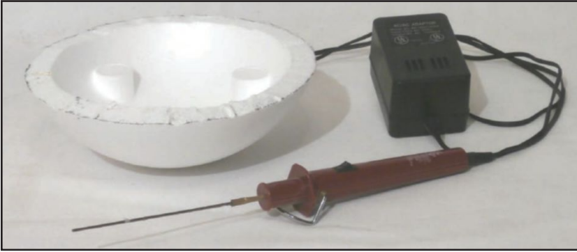
Photo 5: I used a hot knife cutting tool to cut the Styrofoam reflectors down to the proper size.
