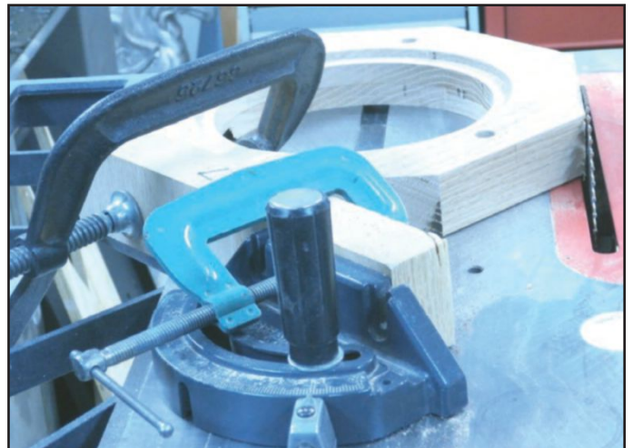
Photo 4: I built this jig from two C-clamps and a scrap of wood to cut off the corners off the two oak tops. I think the octagon tops are more attractive than their original square. However, I left the bottom oak pieces square for better stability.
