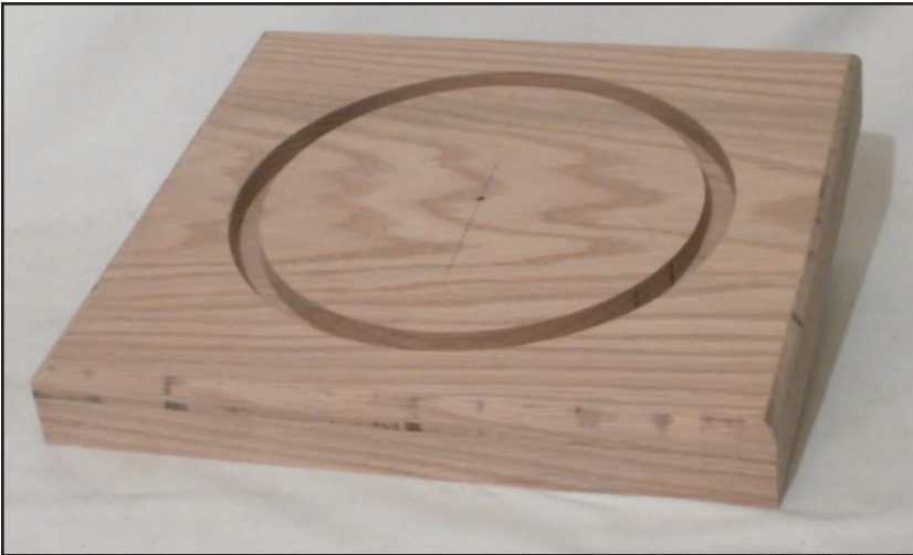
Photo 6: A view of one of the oak bottoms shows the circular glue ring, a half inch wide by a half inch deep. The top corners have been rounded on the table router.
