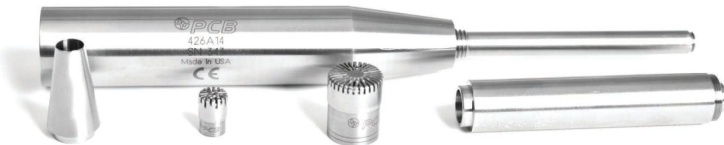
Photo 1: The 426A14 microphone preamp and body is supplied with adapters to allow use of both 1/2" and 1/4" capsules. (Photo by Cynthia Wenslow)
