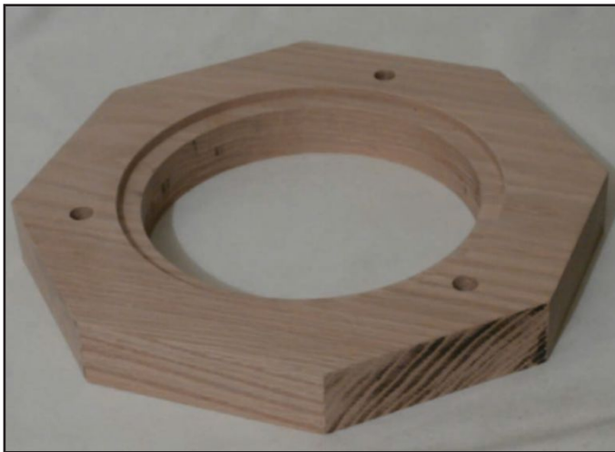
Photo 3: The top side of the red oak top shows the speaker cutout. The circular groove for gluing to the PVC pipe is on the other side and it must be cut before the speaker cutout is completed.
