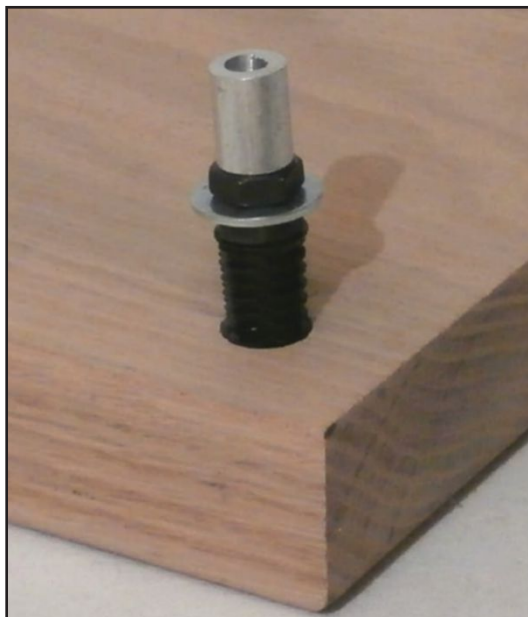
Photo 7: This is the corner spike and its holder before being pressed into the oak bottom. The top spacer covers the tip of the spike.
