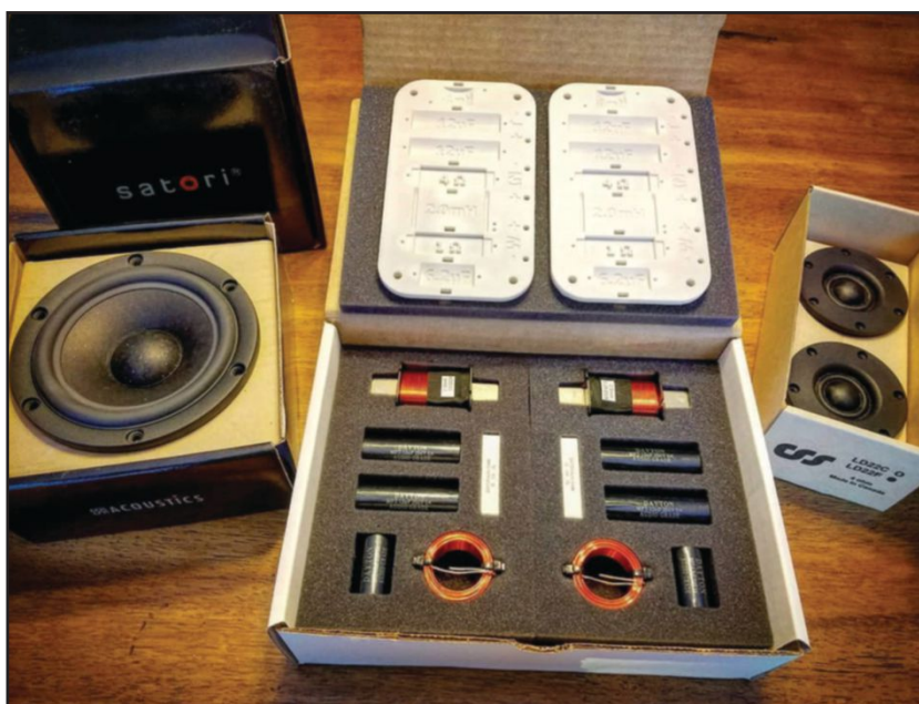
The new CSS P215 Kit uses a Satori MW 13P-8 Egyptian papyrus cone woofer and a CSS LD22 tweeter. The crossovers come with clearly labeled components and pre-formed/drilled fully labeled plates.
