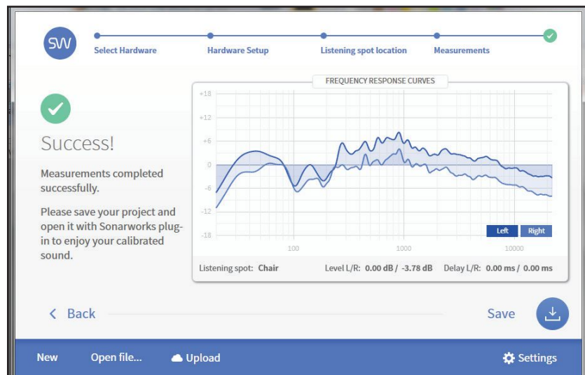
Figure 6: After completion of the 24 response measurements, the software generates frequency response correction curves for left and right channels.
