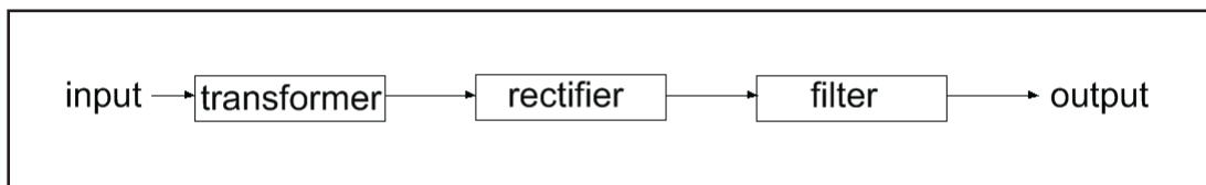
Figure 1: This is a block diagram of an unregulated power supply.
