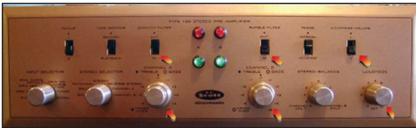
Photo 2: High-fidelity mono and early stereo amplifiers had several tone controls such as these found on the H. H. Scott Type 130 preamplifier.
