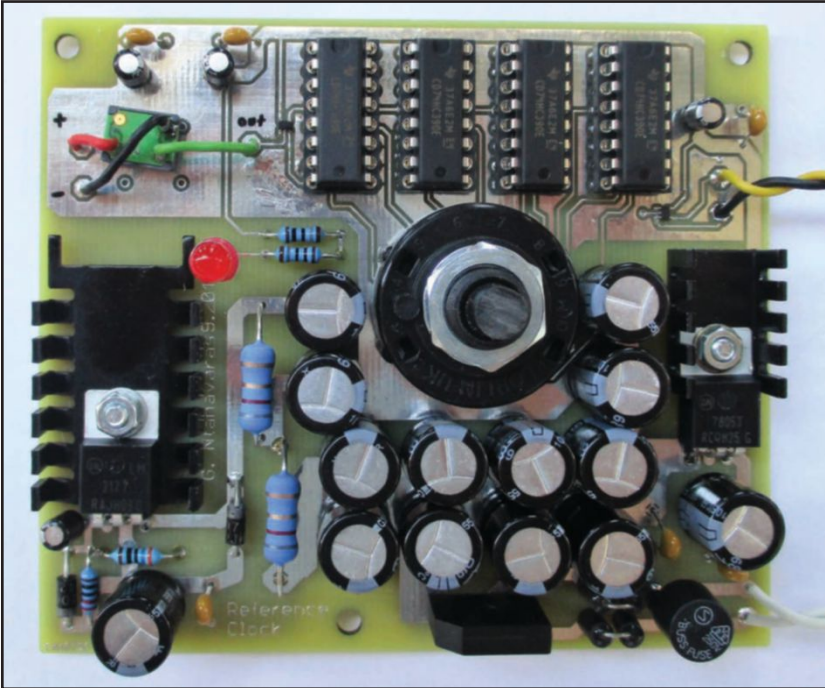
Photo 5: This is a top view of the Reference Oscillator's completed PCB.
