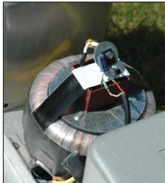
Photo 4: This is the toroidal power transformer for Amplifier 5. On top of it, the Meanwell AC/DC converter plus slow-start for the ECC81 filament.
