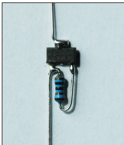
Photo 2: Here is the simple construction of the constant current source.
