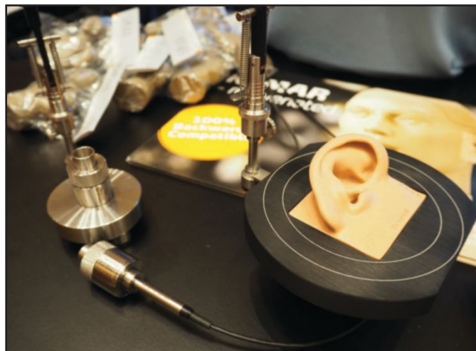
This is the GRAS 43AG Ear-and-Cheek Simulator and the new GRAS RA040X High-Resolution Ear Simulator.
