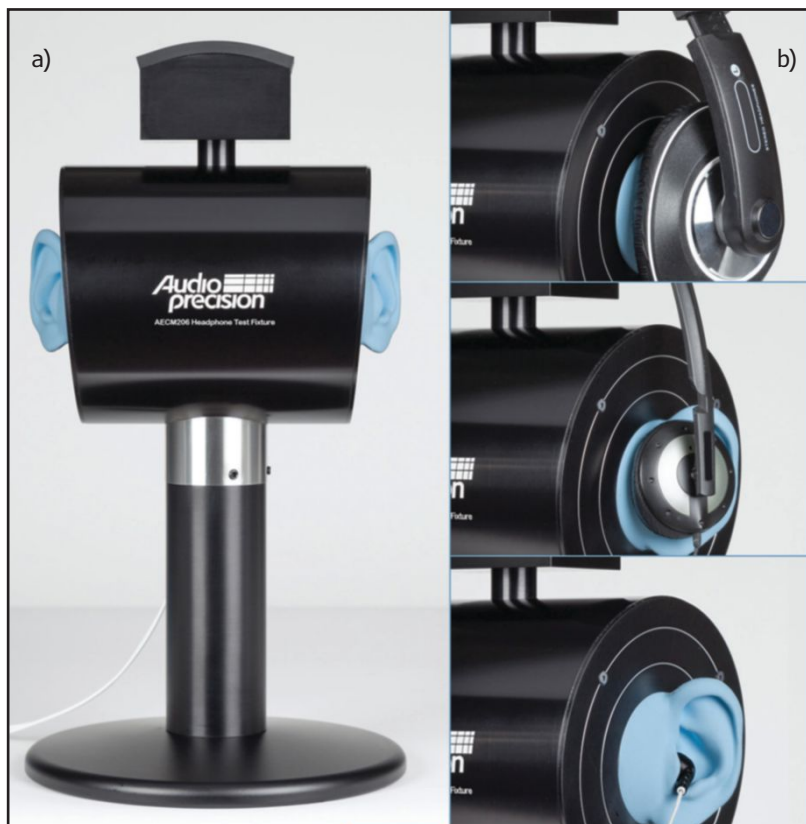
The new Audio Precision AECM206 (a) is a dense, robust fixture mounted on a resilient base to isolate ambient noise. Two sets of pinnae are provided with the unit (b).
