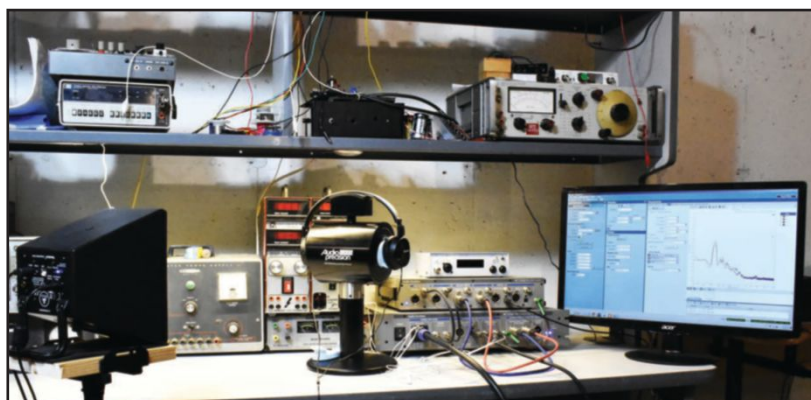
Photo 4: To test the noise cancellation of headphones, I set up a loudspeaker near the AECM206 on my test bench.
