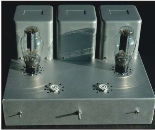
Photo 3: Menno van der Veen's Amplifier 1 is an FET driver stage plus 300B in 2A3 configuration.
