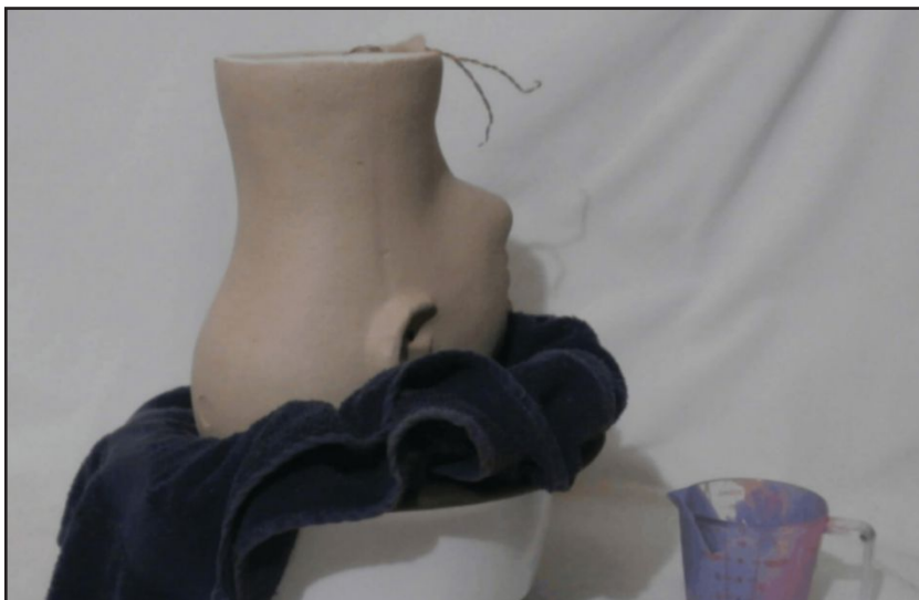
Photo 4: With the head upside down, slowly pour the liquid rubber mixture into the center hole until the level is about an inch from the top. This leaves space for the splices connecting the microphone wires to the shielded microphone cable. The rubber takes about 6 hours to cure. Part A is pink and Part B is blue so it's fairly easy to get them well mixed.
