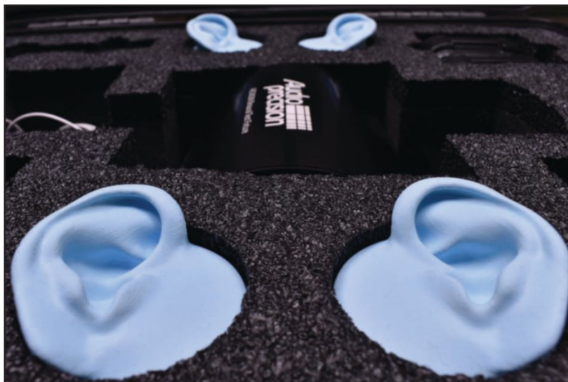
Photo 3: The system includes two sets of molded ears with different stiffness.
