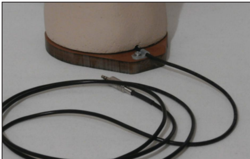
Photo 9: Allow 24 hours for the caulk to set, then trim off any leakage and attach the microphone cable to the base plate. Your HRTF head is ready for testing and use. Enjoy!
