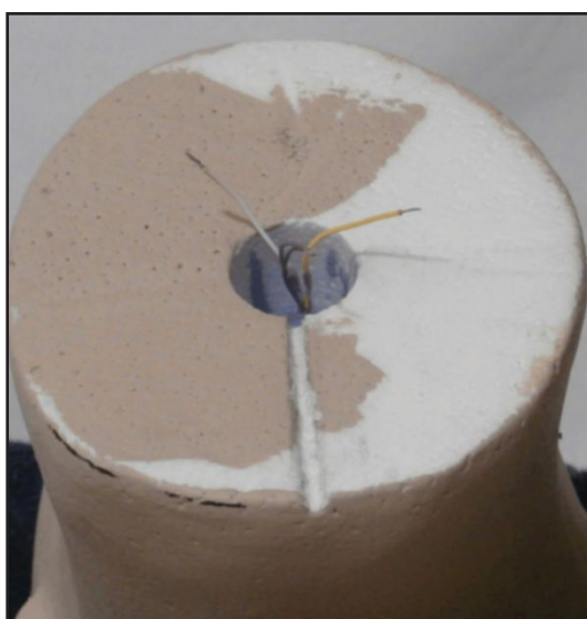
Photo 4: With the head upside down, slowly pour the liquid rubber mixture into the center hole until the level is about an inch from the top. This leaves space for the splices connecting the microphone wires to the shielded microphone cable. The rubber takes about 6 hours to cure. Part A is pink and Part B is blue so it's fairly easy to get them well mixed.
