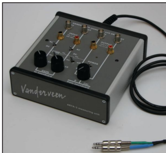
Photo 5: The Arta-2 measuring unit can be connected to a sound card.
