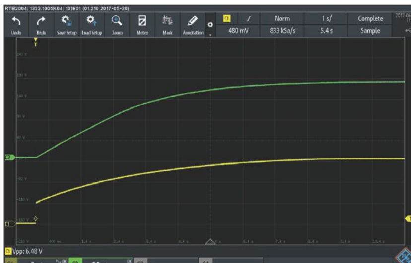
Figure 3: This graph shows filament and the high voltage rise gradually over about 10 seconds on turn on.
