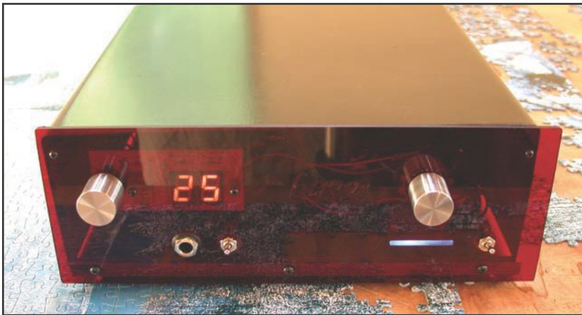
Photo 2: The 6922's more traditional case was much easier to build with the benefit of having all the boards separated by a good distance.
