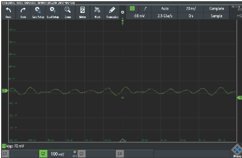
Figure 4: Although the high voltage supply contains 180 V, it emits very low noise (70 mV).
