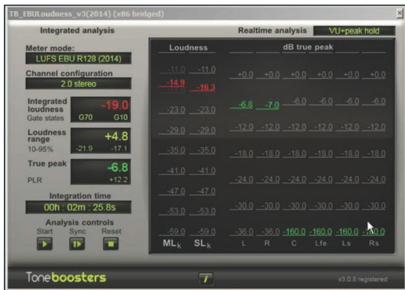
Photo 2: The Toneboosters Loudness Meter continues to display all the final values when the file analysis ends making it easy to write the numbers down. The Meter modes include LKFS ITUR BS.1770/3, but it has not yet been updated to include BS.1770/4. In all my measurements, Meter modes LUFS EBU R128 (2014) and LKFS ITUR BS.1770/3 gave the same results.
